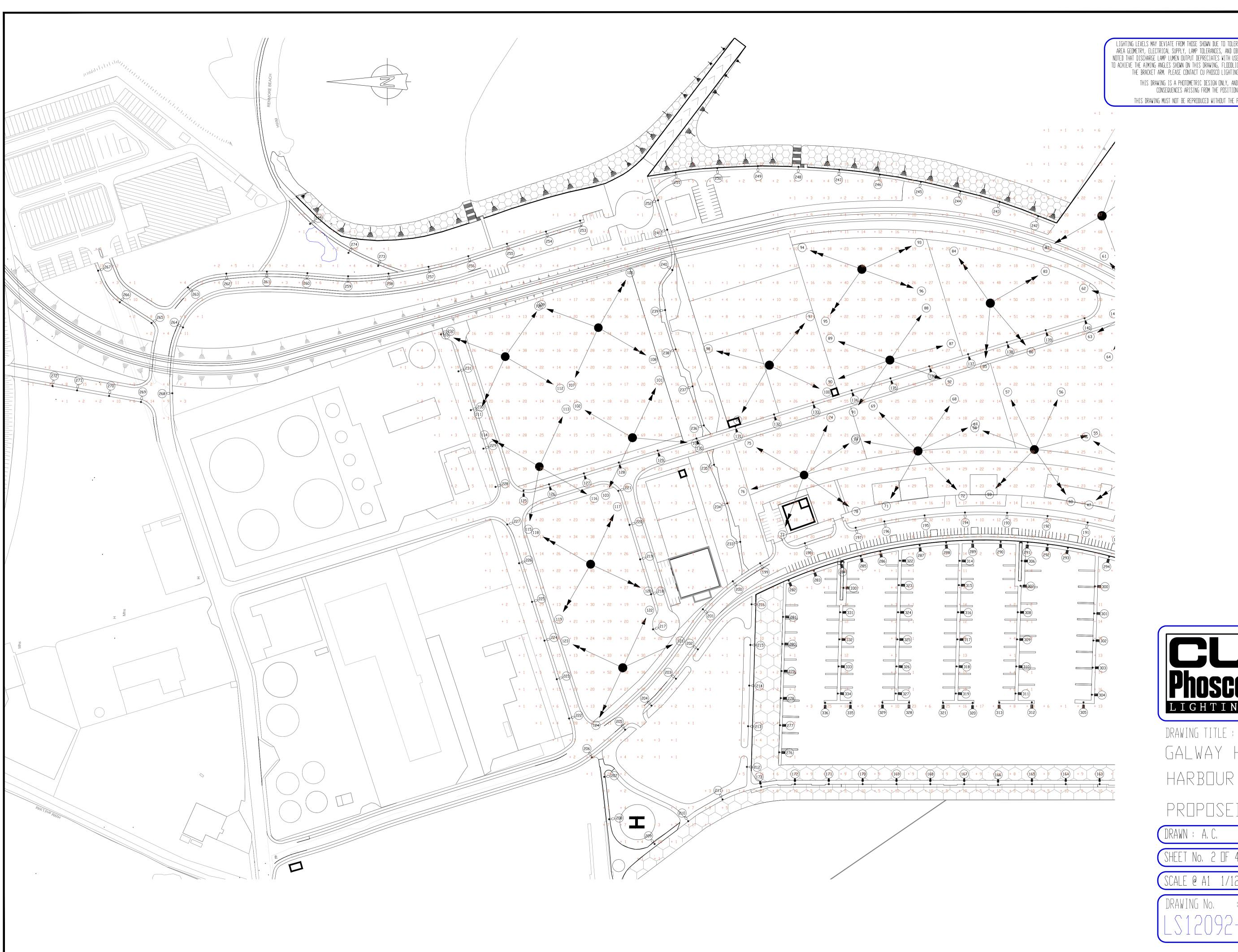
TO ACHIEVE THE AIMING ANGLES SHOWN ON THIS DRAWING, FLOODLIGHTS MAY NEED TO BE MOUNTED ABOVE AND BELOW THE BRACKET ARM. PLEASE CONTACT CU PHOSCO LIGHTING IF MORE INFORMATION IS REQUIRED.
