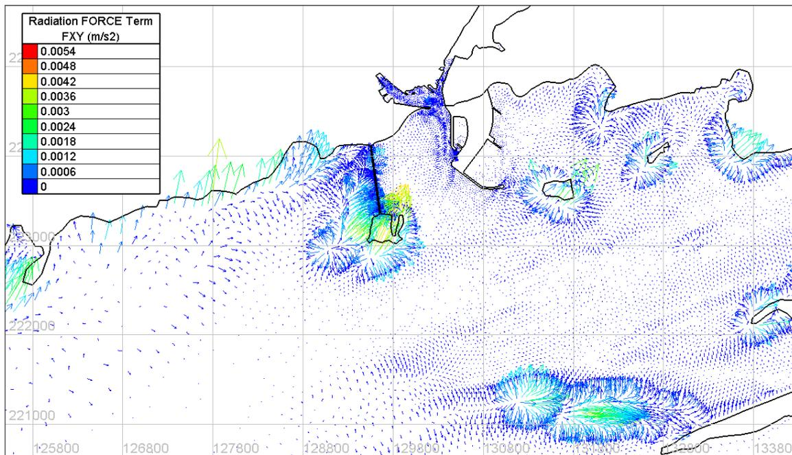
Figure 4.5.2 Radiation Force Vectors for Proposed Case
