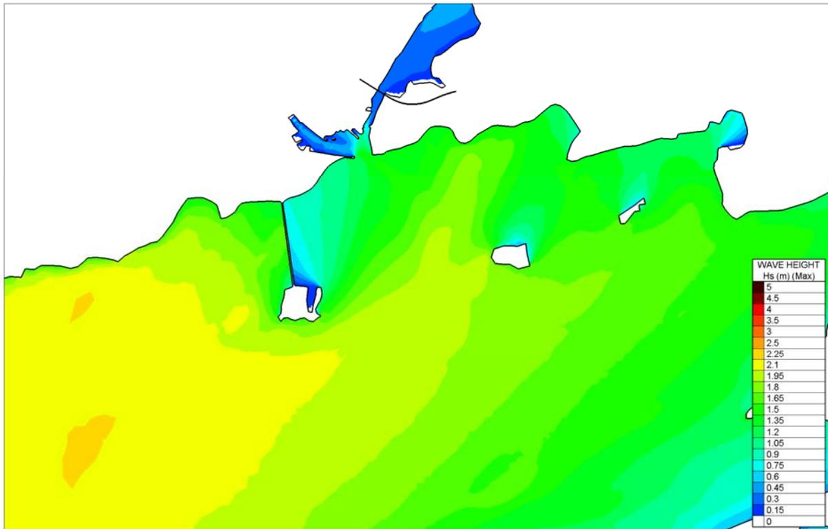
Figure 4.4.17 Computed Significant Wave heights for Local South Storm Winds - Existing
