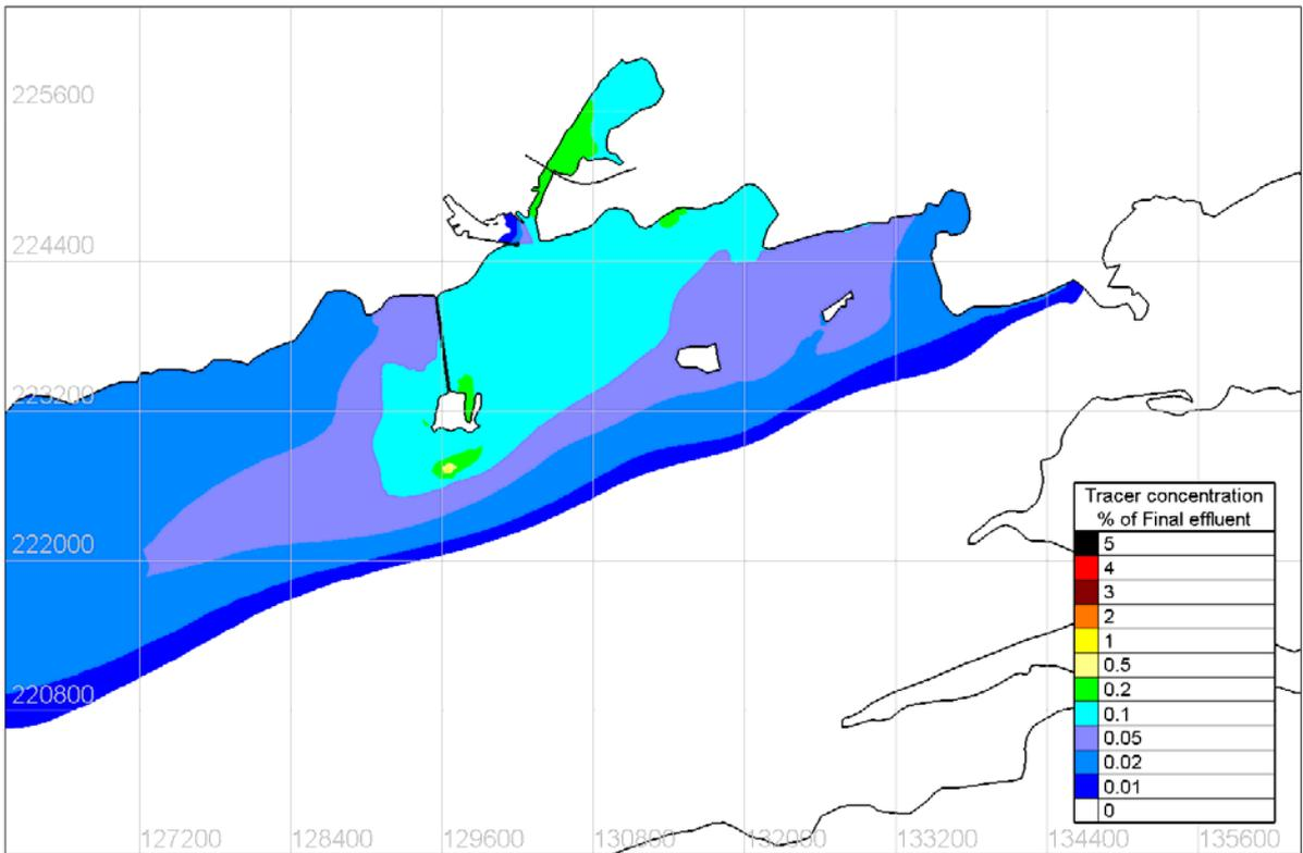
Figure 4.8.33 Tidal mean tracer concentration under SSW 15m/s wind conditions – Existing Case
