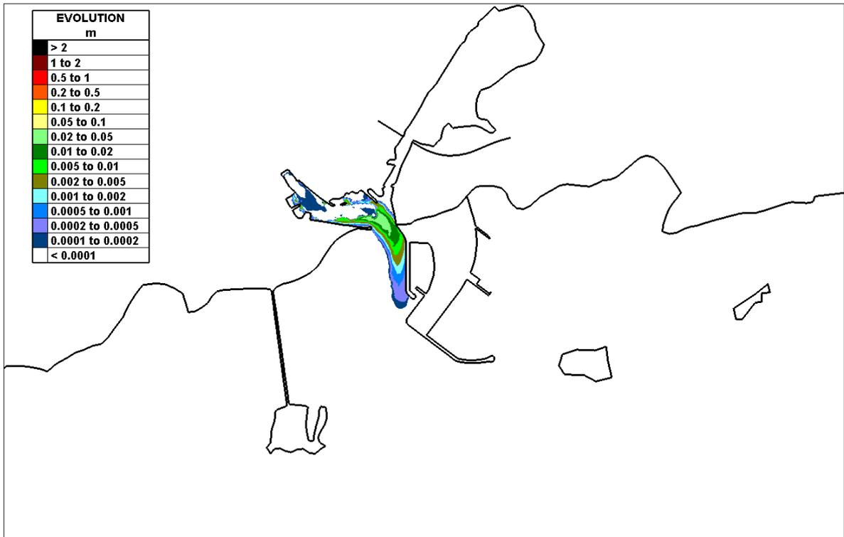
Figure 4.1.7 Deposition of a Corrib fine sand under median flows at the end of 15 days - Proposed Case
