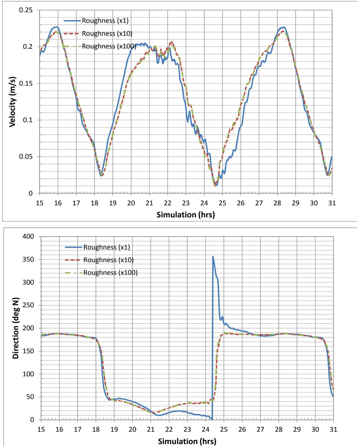
Figure 4.6.10 Sensitivity of Velocities to Roughness factor at Site 4
