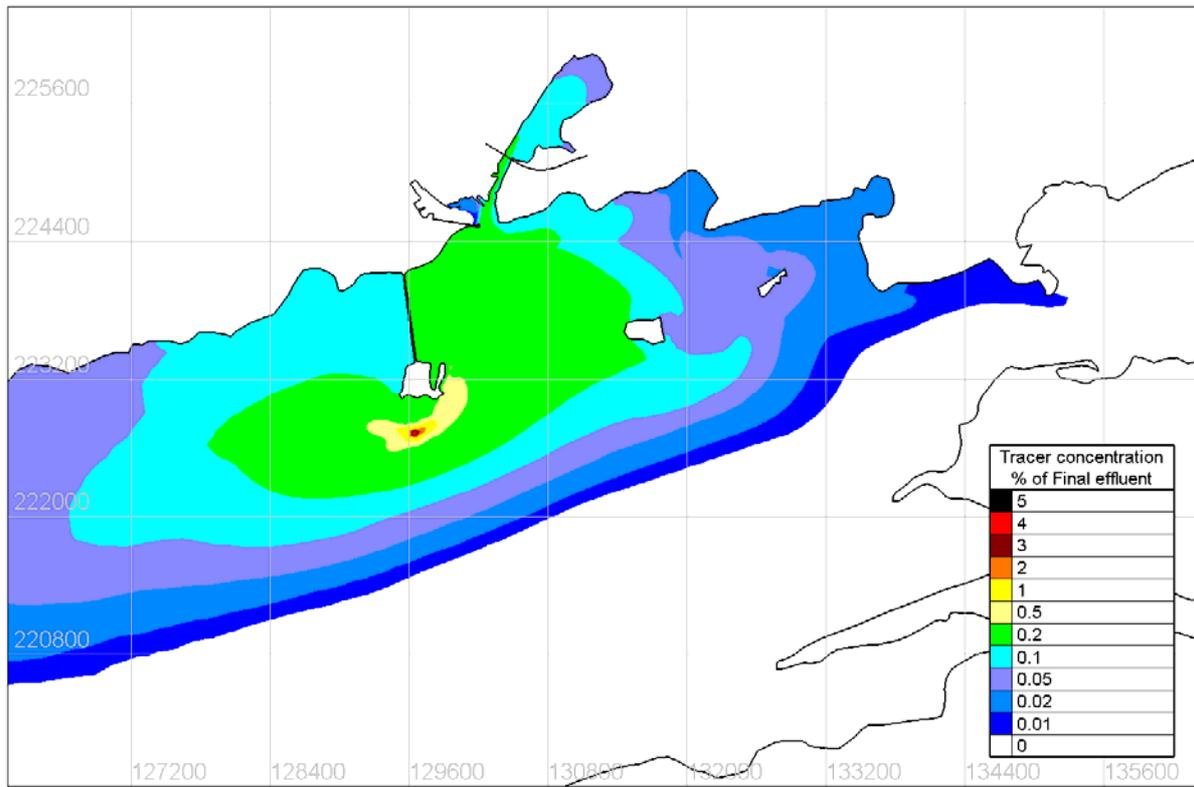
Figure 4.8.19 Maximum surface concentration of Tracer under South 5m/s wind conditions– Existing
