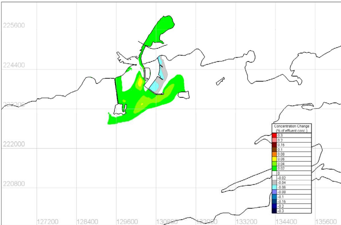
Figure 4.8.42 Predicted change in tidal mean tracer concentration – S 15m/s Wind Condition
