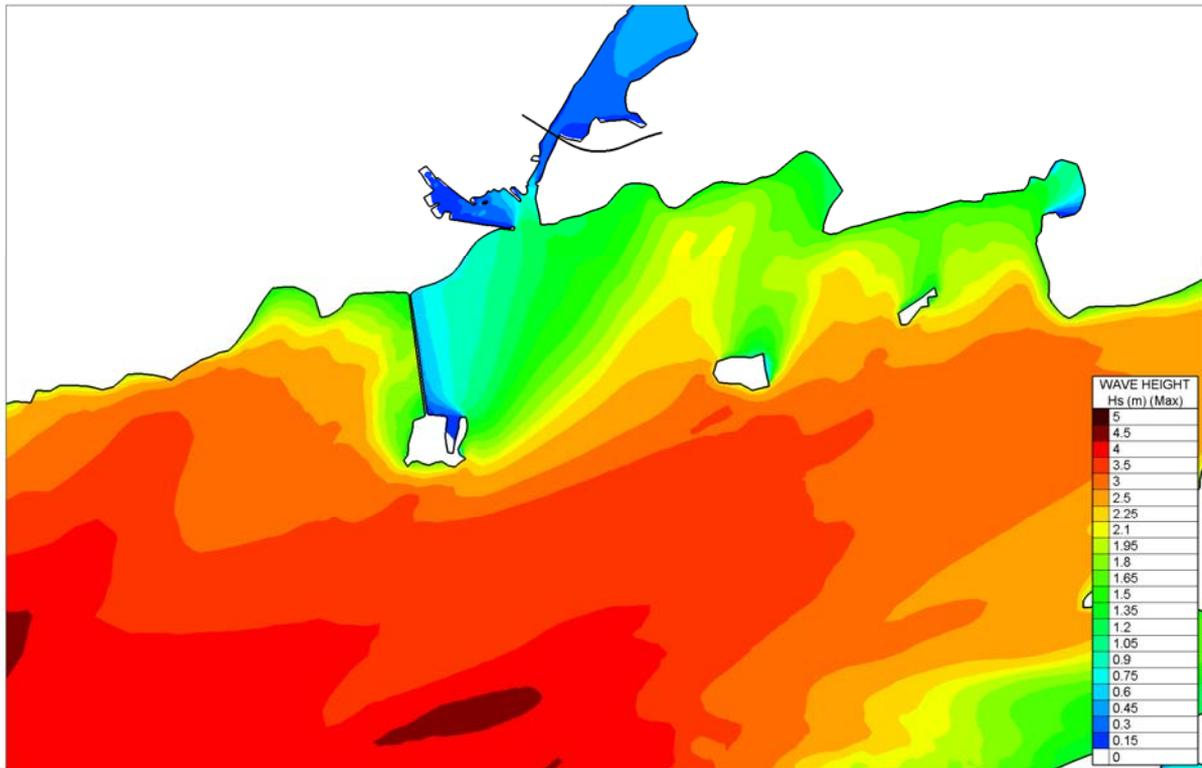
Figure 4.4.5 Computed Significant Wave heights for Atlantic Storm and SW
