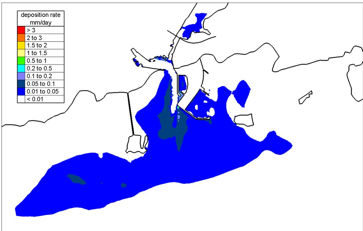
**Figure 4.1.13** Computed depositional rates of a River Corrib fine silt under Winter flood flows (1 %-ile 272cume) - Proposed Case.
