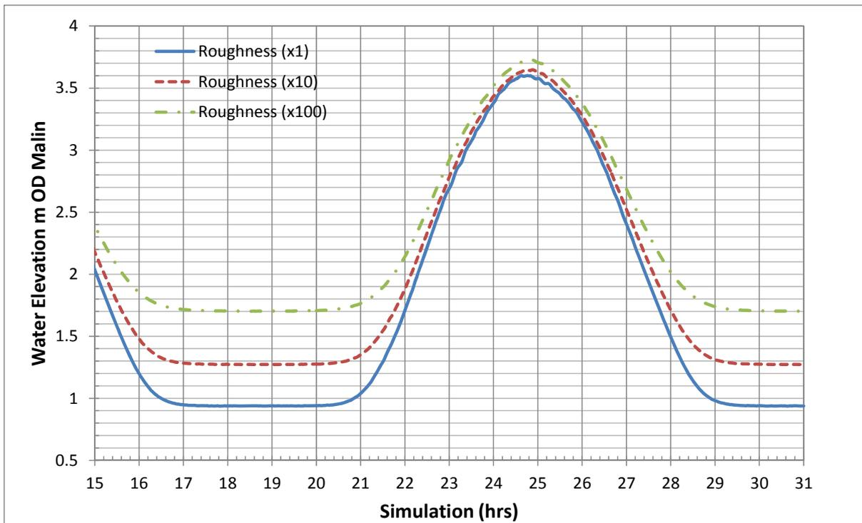
Figure 4.6.2 Sensitivity of elevation to Roughness factor at Site 1
