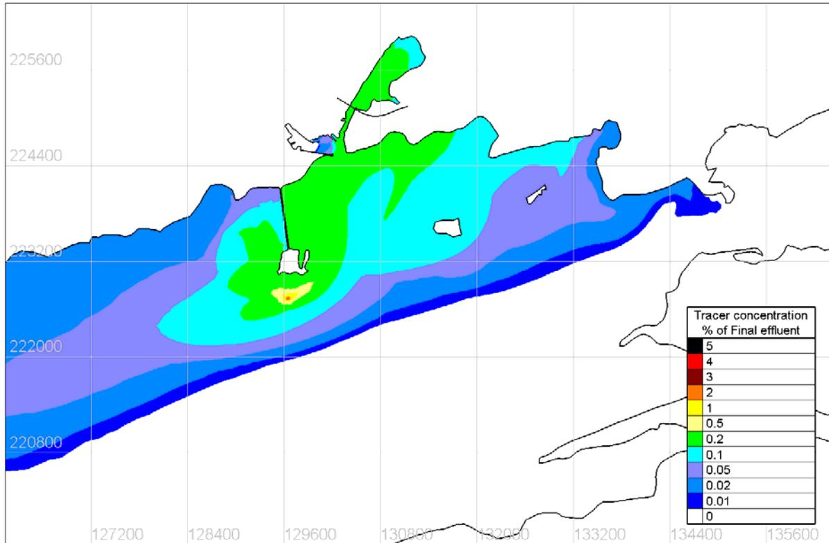
Figure 4.8.31 Maximum surface concentration of Tracer under SSW 15m/s wind conditions– Existing
