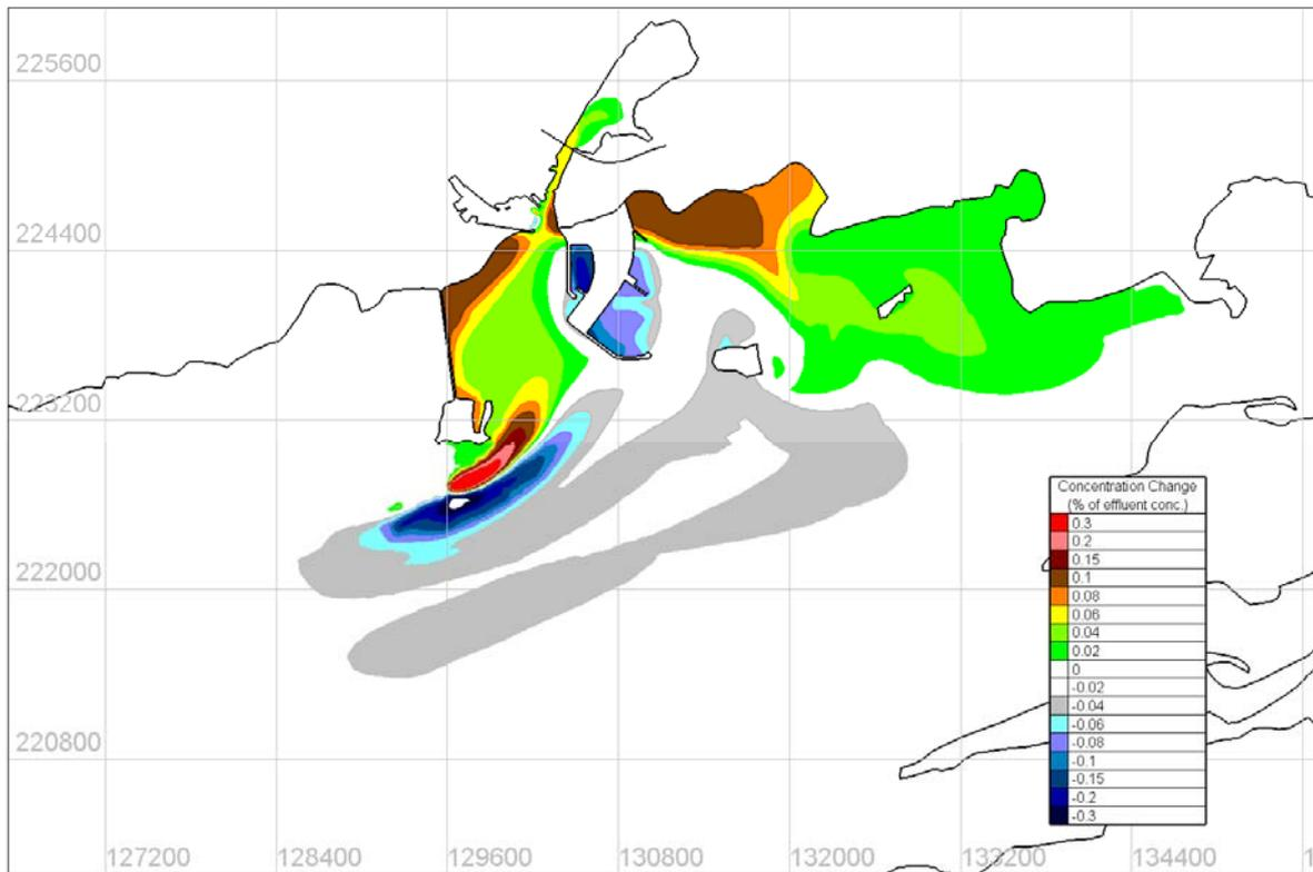
Figure 4.8.5 Predicted change in maximum surface tracer concentration – Calm Wind Conditions
