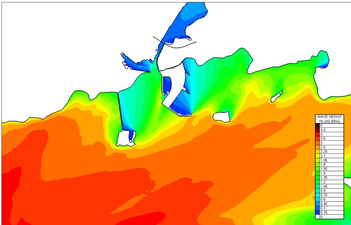
Figure 4.4.8 Computed Significant Wave heights for Atlantic Storm and SSW Storm Winds - Proposed
