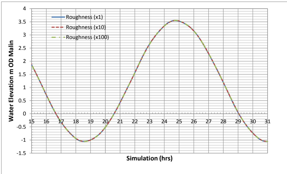
Figure 4.6.4 Sensitivity of elevation to Roughness factor at Site 3
