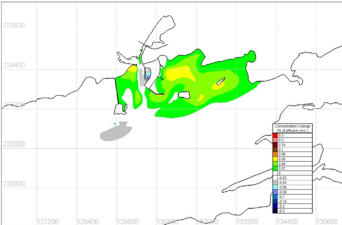
Figure 4.8.24 Predicted change in tidal mean tracer concentration – South 5m/s Wind Condition
