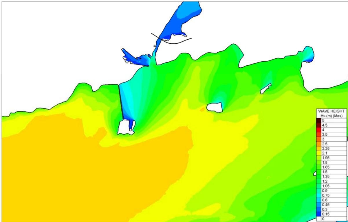
Figure 4.4.15 Computed Significant Wave heights for Local SSW Storm Winds - Existing
