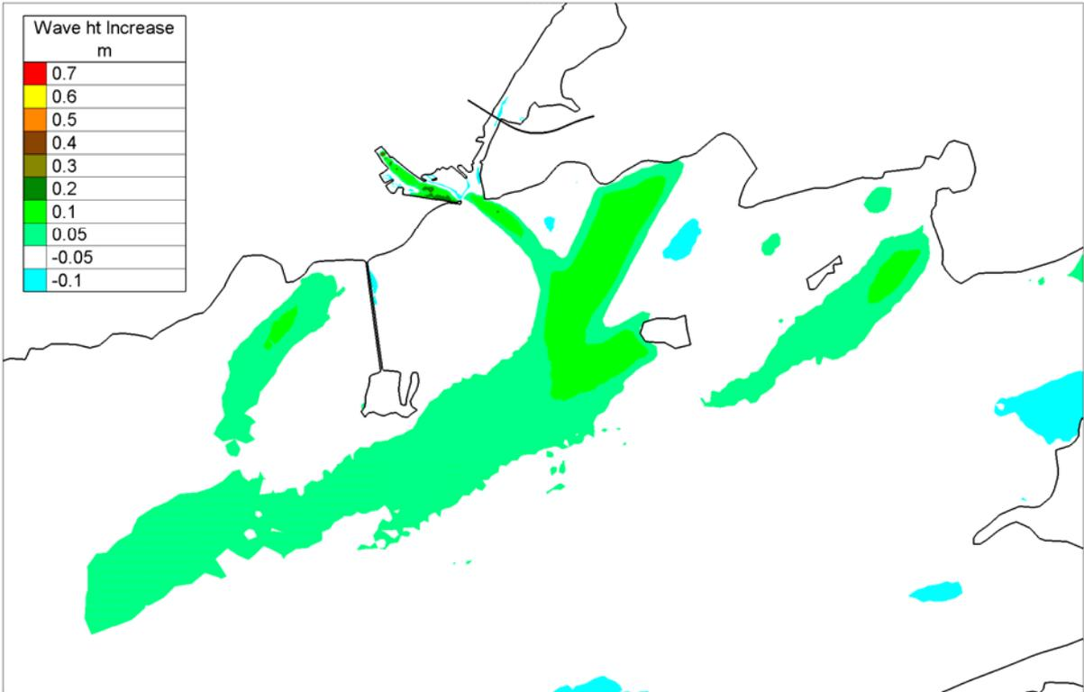
Figure 4.3.15 Difference Plot showing the effect of Tidal velocities on Wave height for South Storm wind conditions - Existing
