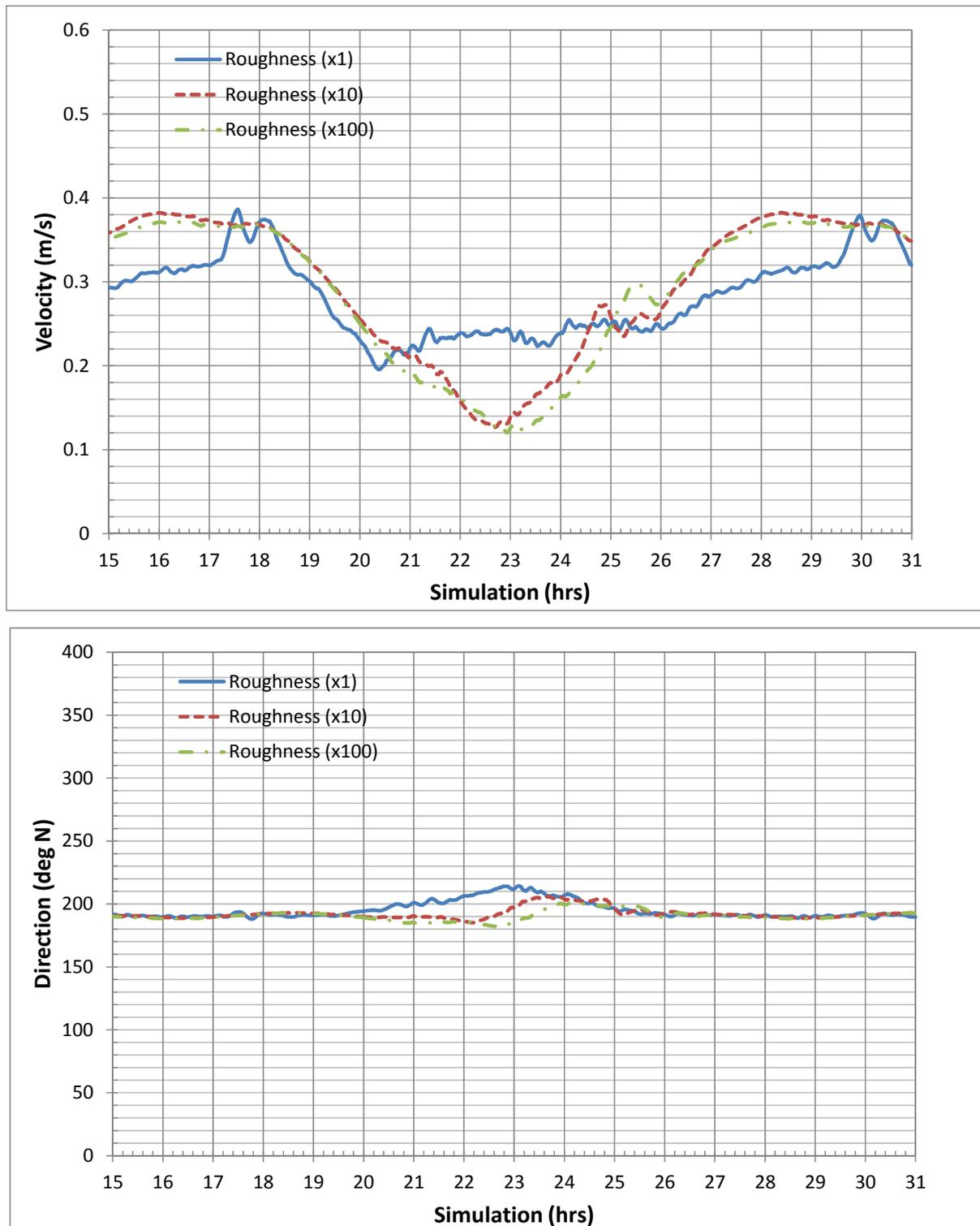
Figure 4.6.8 Sensitivity of Velocities to Roughness factor at Site 2
