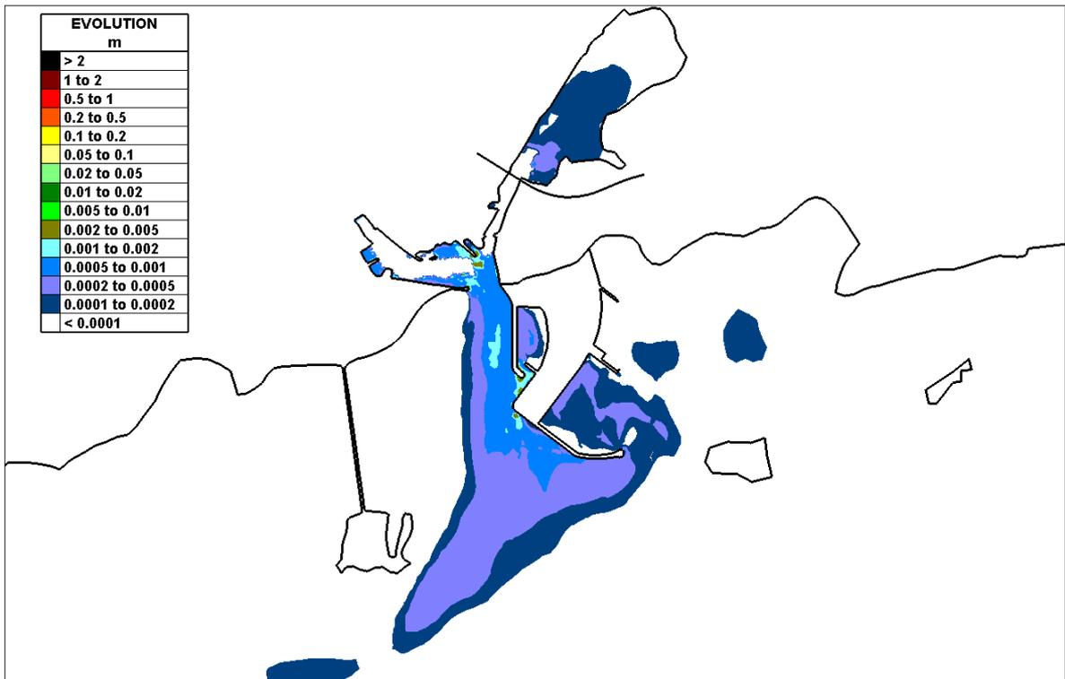
Figure 4.1.3 Deposition of a Corrib silt under median flows at the end of 15 days - Proposed Case (the white area within the Claddagh Basin and Lough Atalia channel is self-cleansing).
