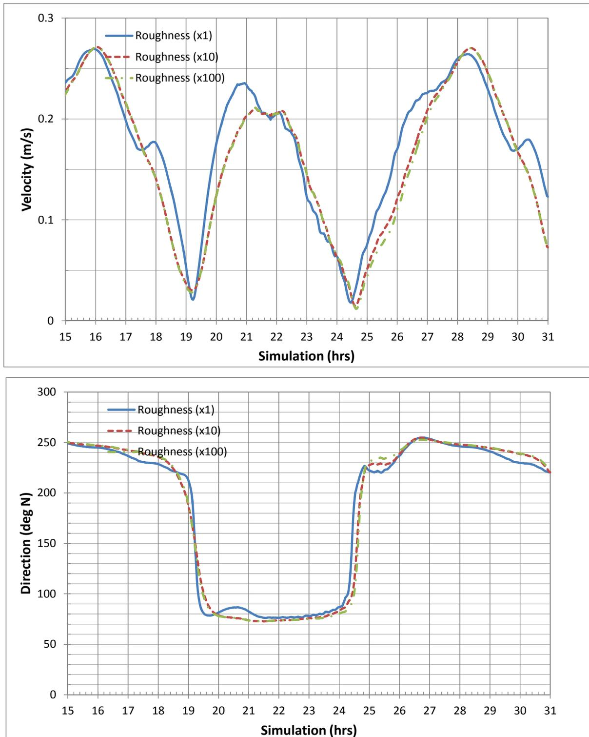
Figure 4.6.9 Sensitivity of Velocities to Roughness factor at Site 3
