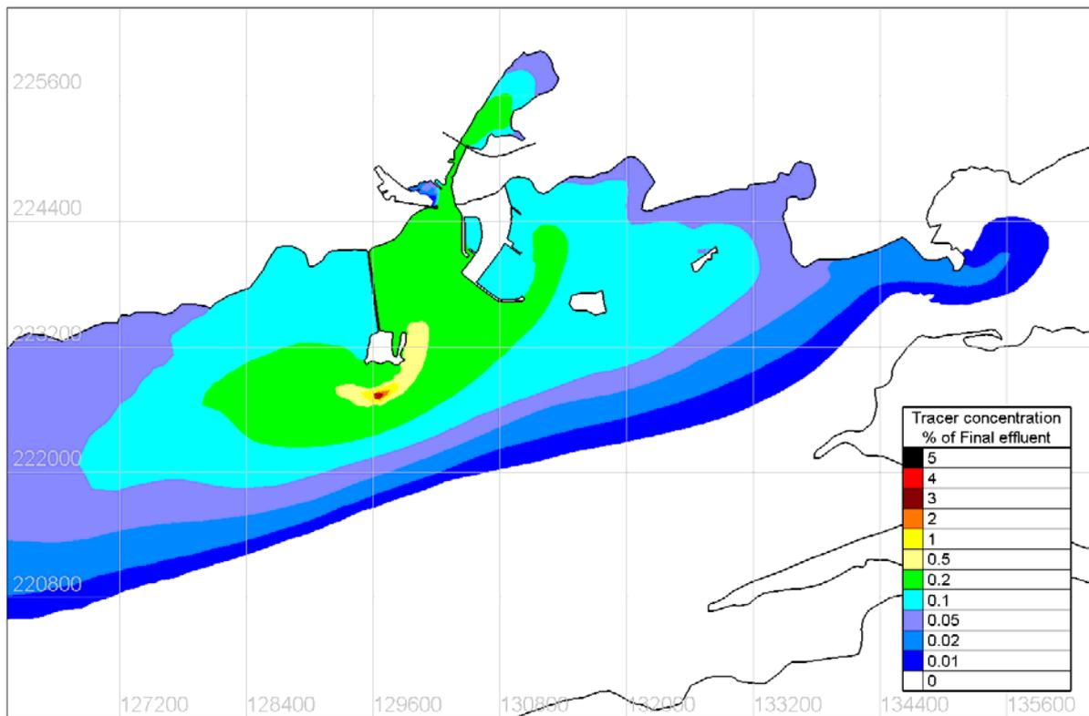
Figure 4.8.20 Maximum surface concentration of Tracer under South 5m/s wind conditions– Proposed
