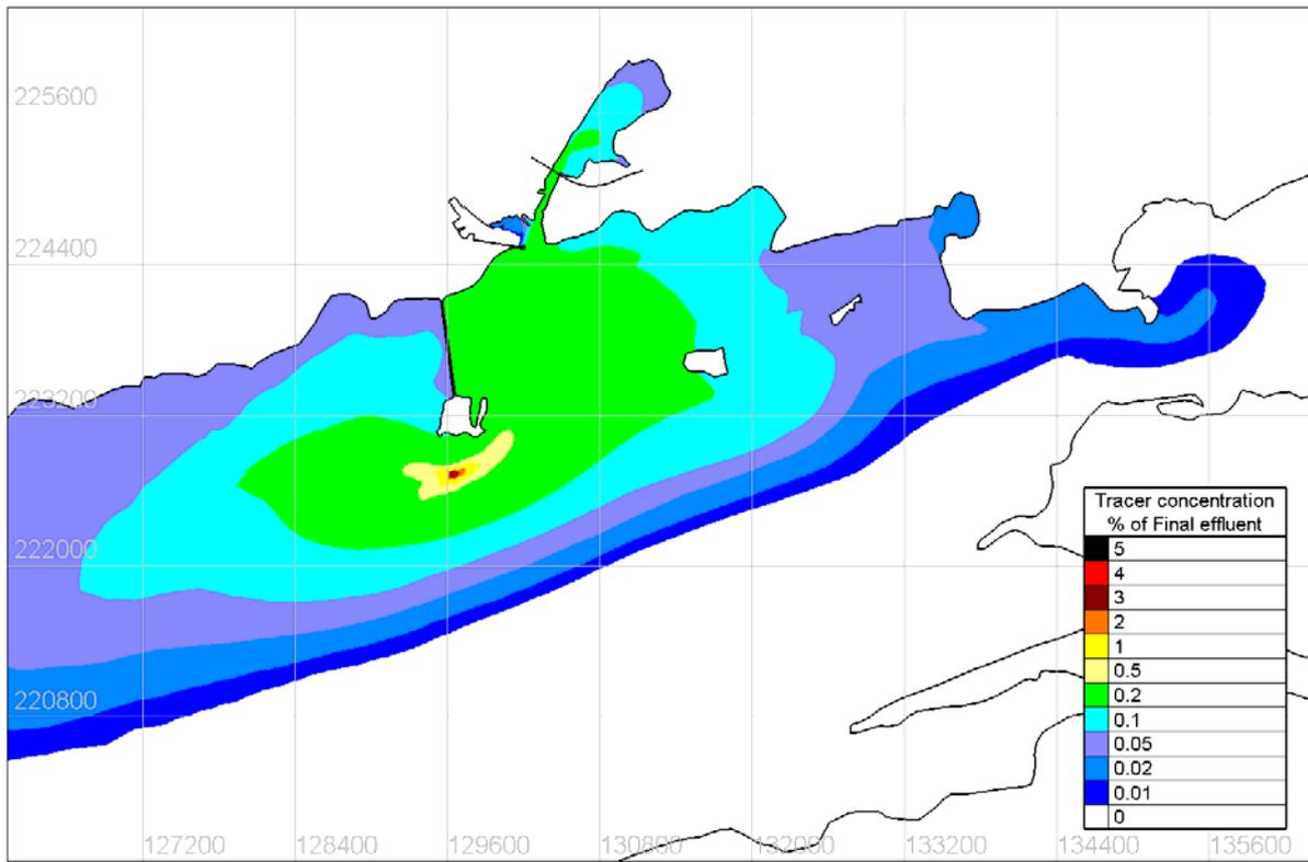
Figure 4.8.13 Maximum surface concentration of Tracer under SSW 5m/s wind conditions– Existing
