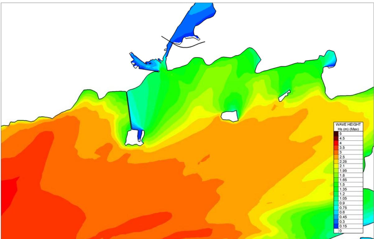
Figure 4.3.14 Predicted Wave Climate for South storm winds with tidal velocities included - Existing
