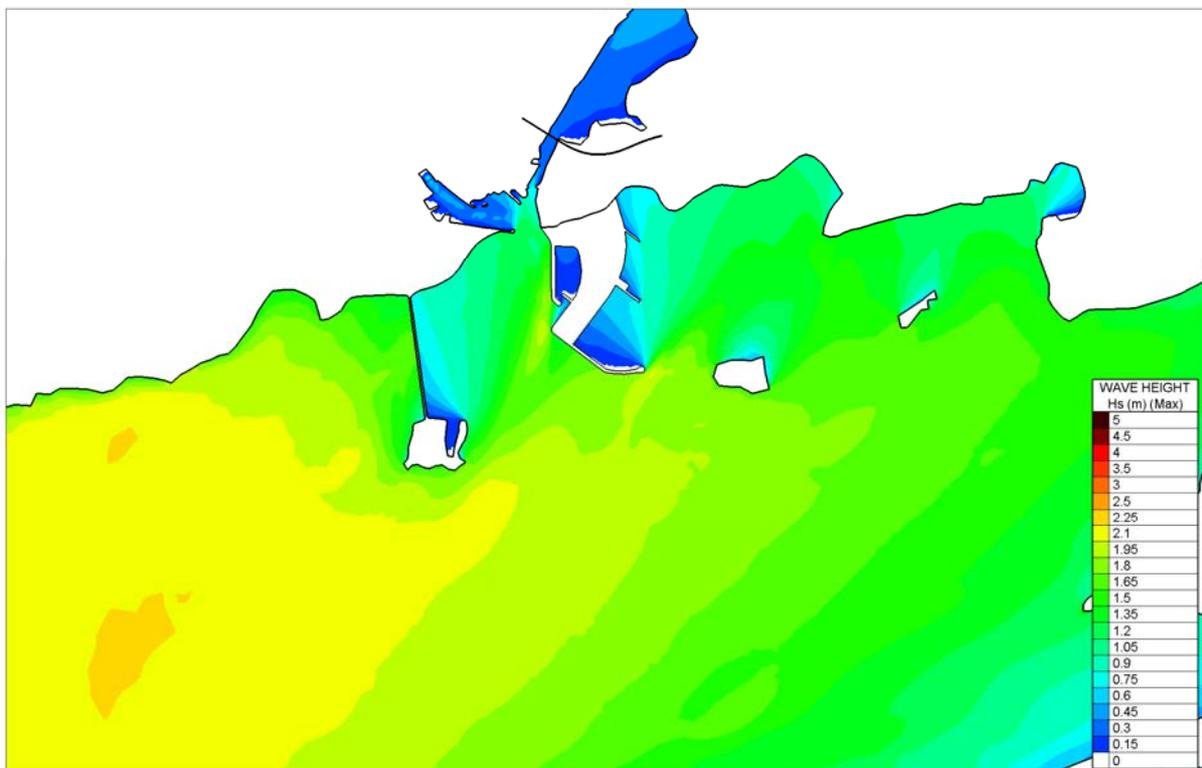
Figure 4.4.18 Computed Significant Wave heights for Local South Storm Winds - Proposed
