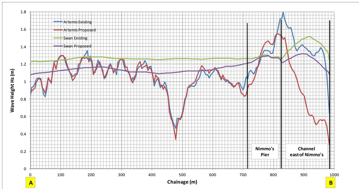
Figure 4.4.42 Computed maximum wave heights for all onshore directions West to ESE along Section A-B (refer to Figure 4.43) showing the SWAN and ARTEMIS Wave Climate model results for Southpark Shoreline and Corrib Entrance.
