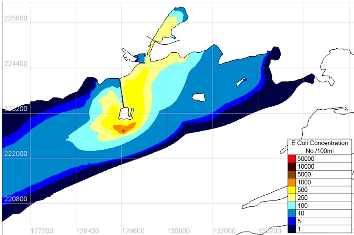
Figure 4.8.46 Maximum faecal coliform surface concentration of Tracer under SSW 15m/s wind conditions– Existing
