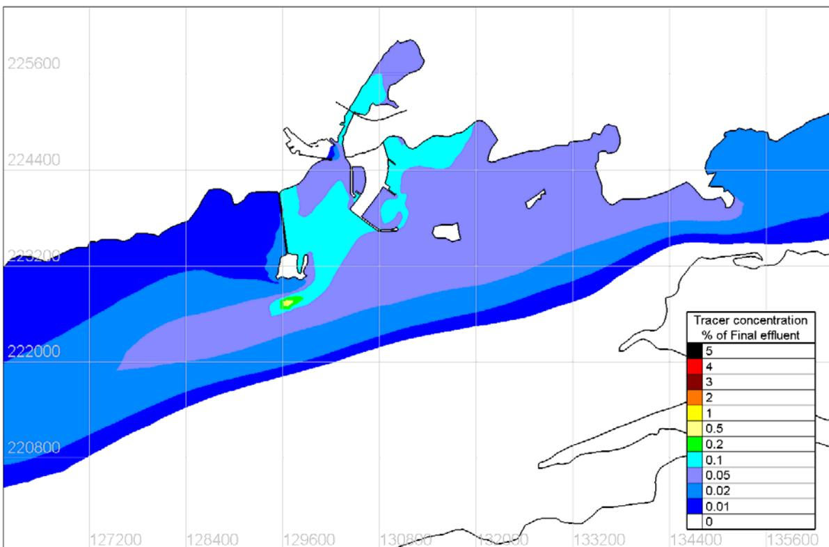
Figure 4.8.28 Tidal mean tracer concentration under SW 15m/s wind conditions – Proposed Case
