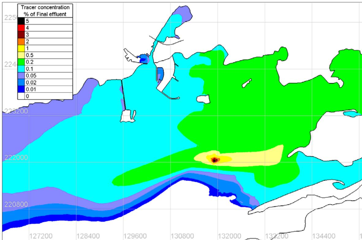
Figure 4.8.56 Maximum surface concentration of Tracer under S 15m/s wind conditions– Proposed
