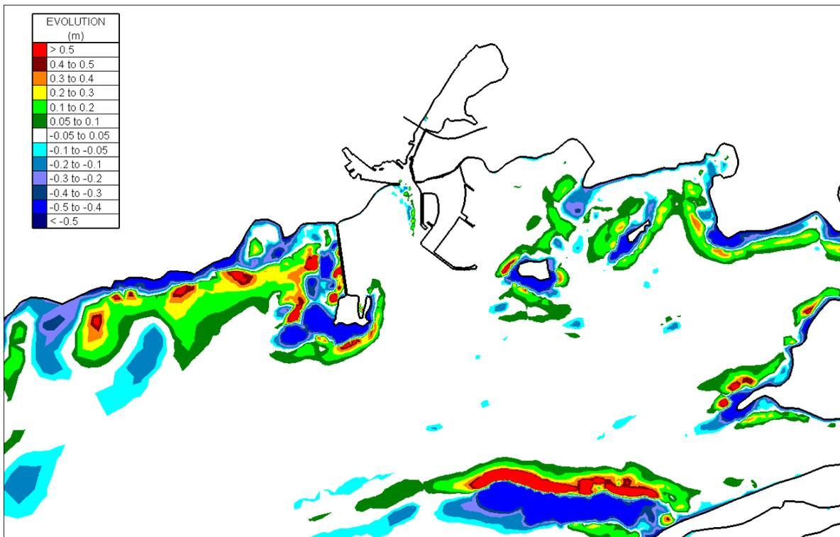
Figure 4.1.19 South Storm Waves Simulation modelling a fine sand - Proposed Case
