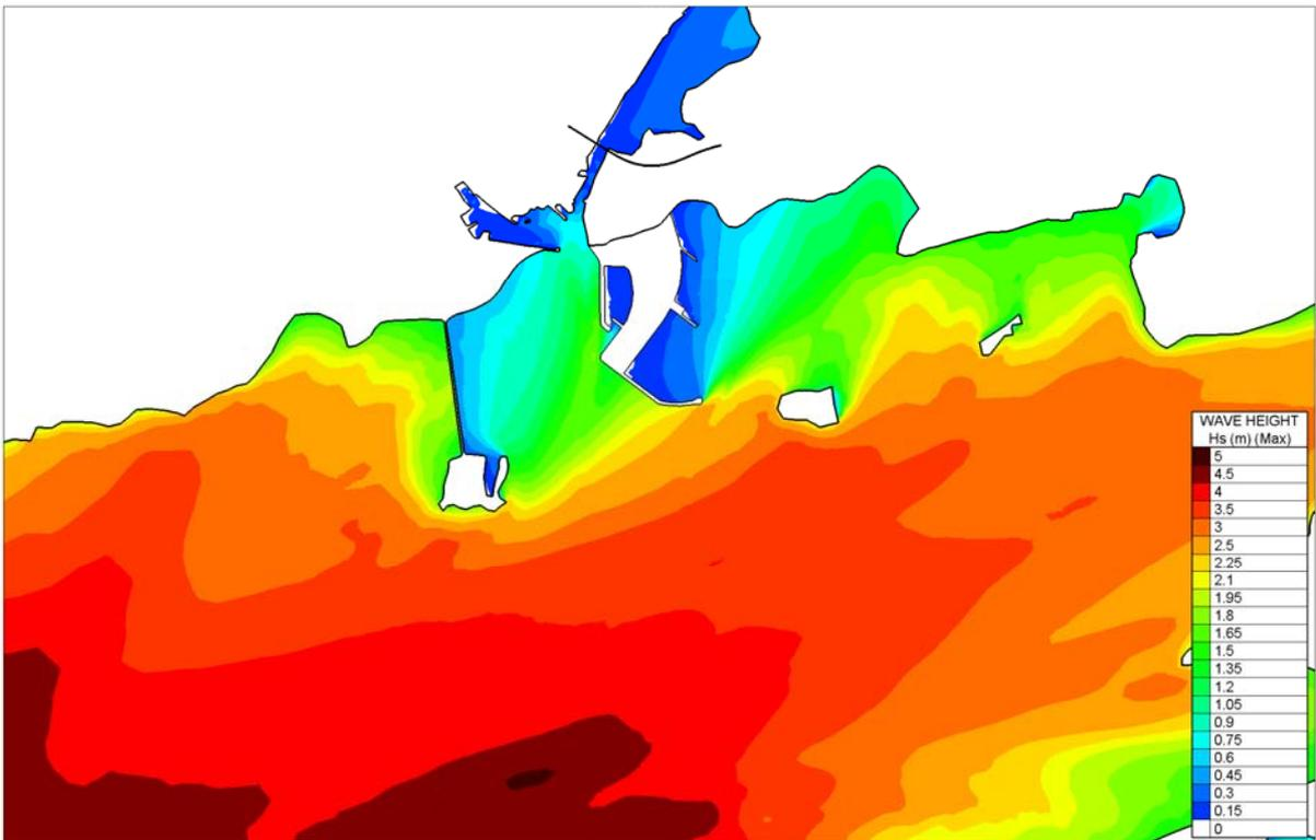
Figure 4.4.2 Computed Significant Wave heights for Atlantic Storm and West Storm Winds - Proposed
