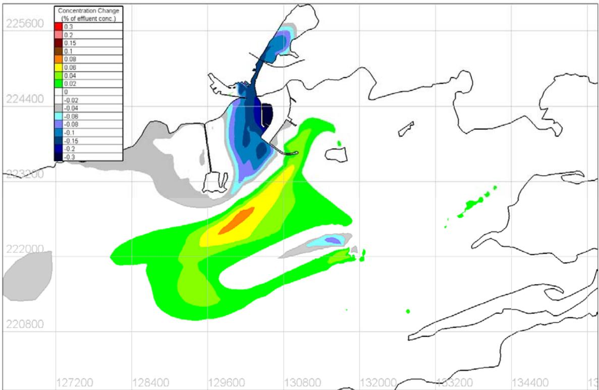
Figure 4.8.65 Predicted change in maximum surface tracer concentration – SE 15m/s Wind Conditions
