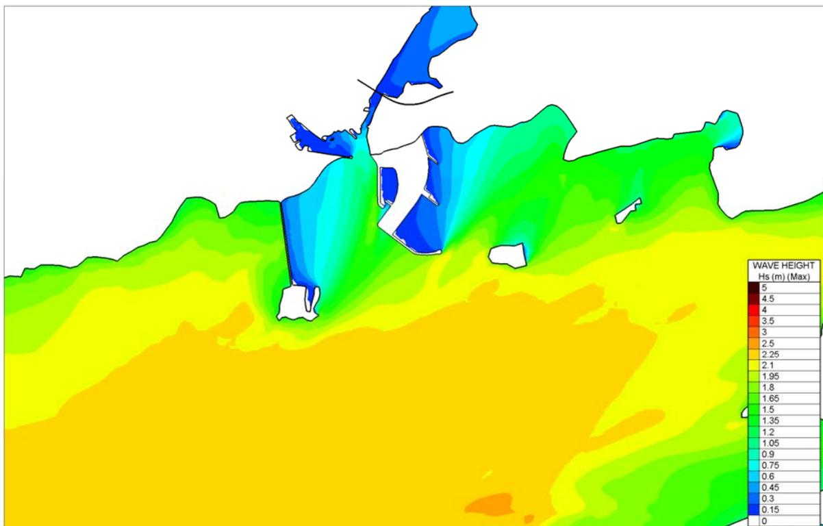
Figure 4.4.12 Computed Significant Wave heights for Local WSW Storm Winds - Proposed
