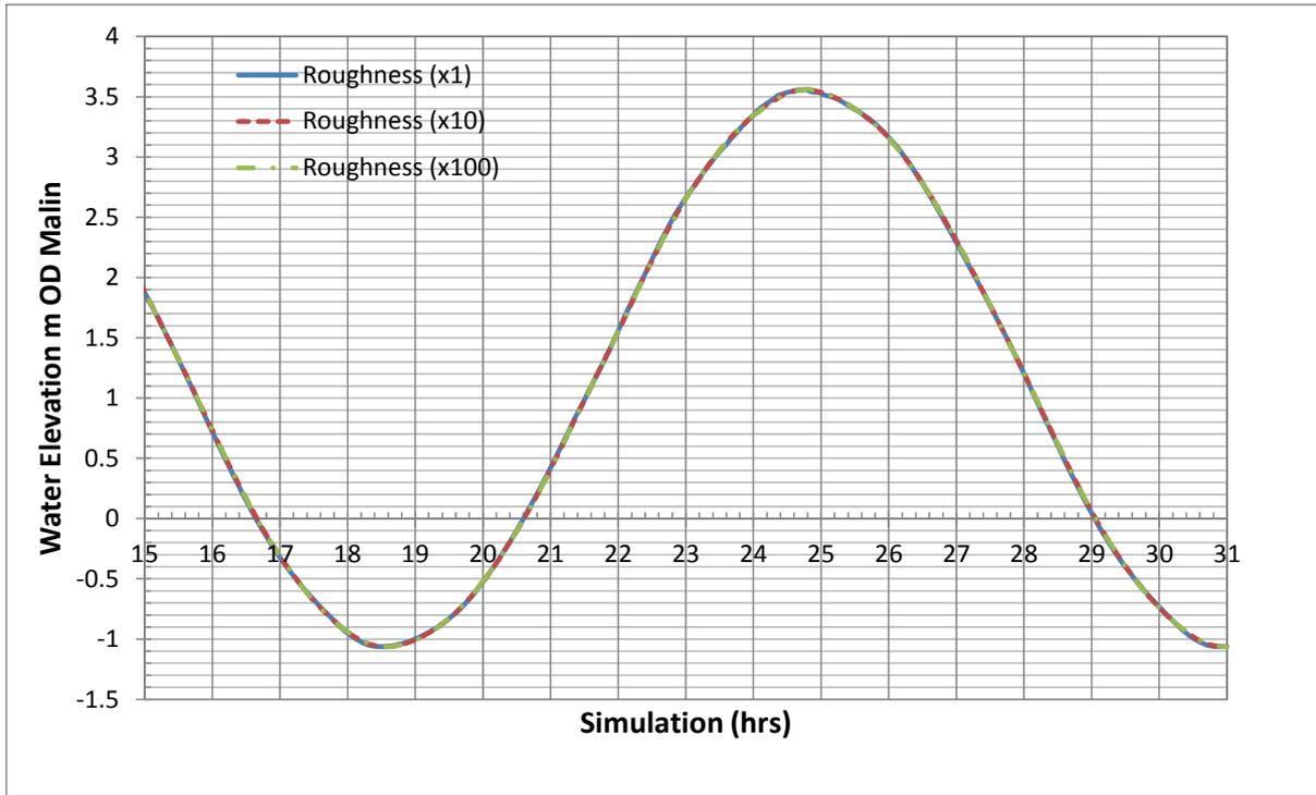
Figure 4.6.6 Sensitivity of elevation to Roughness factor at Site 5
