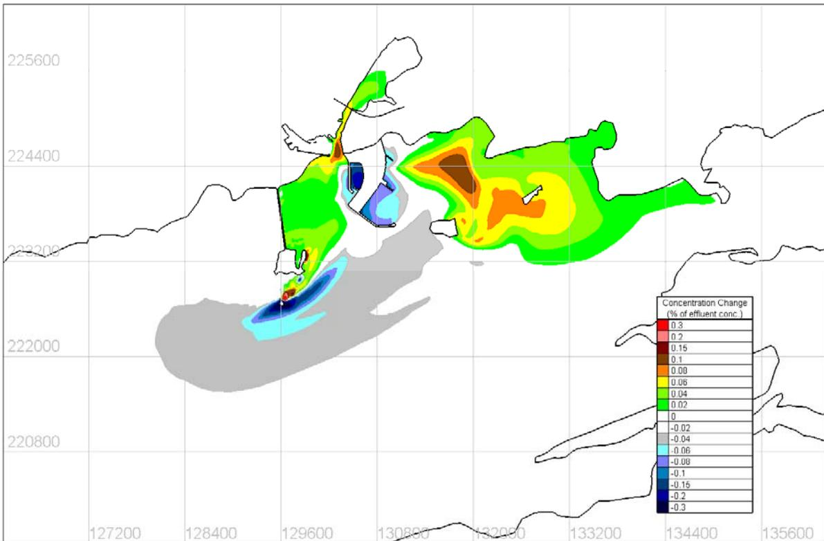
Figure 4.8.23 Predicted change in maximum surface tracer concentration – South 5m/s Wind Conditions
