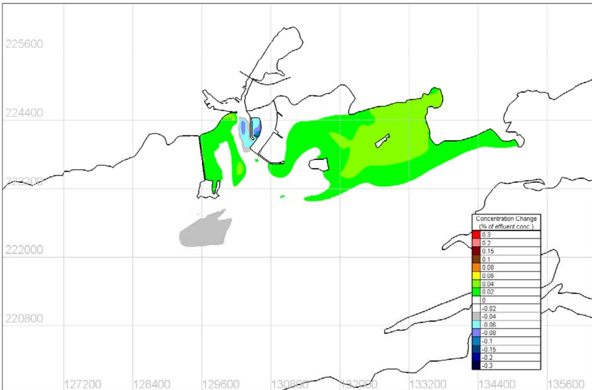
Figure 4.8.18 Predicted change in tidal mean tracer concentration – SSW 5m/s Wind Condition
