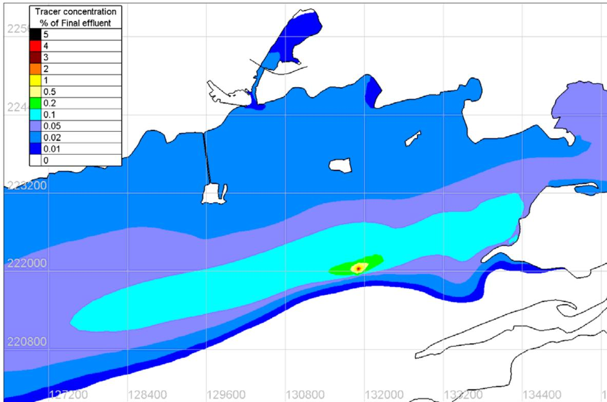
Figure 4.8.51 Tidal mean tracer concentration under SW 15m/s wind conditions – Existing Case
