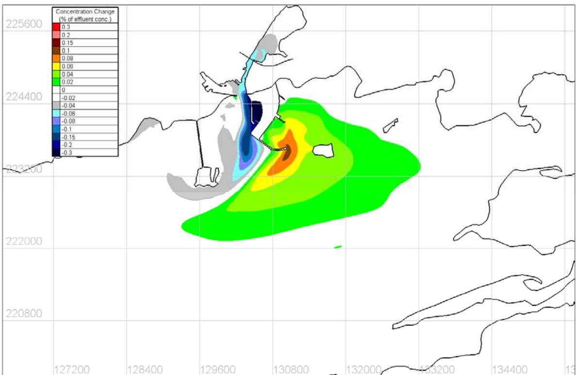
Figure 4.8.66 Predicted change in tidal mean tracer concentration – SE 15m/s Wind Condition
