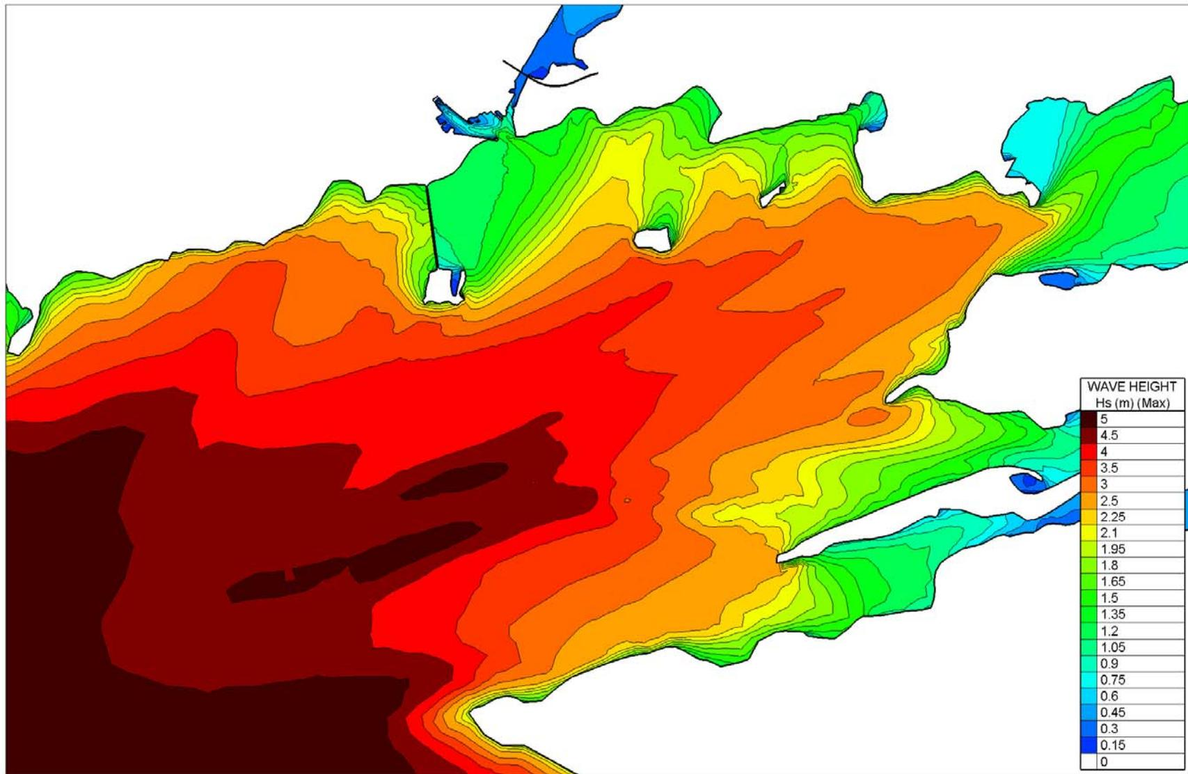
Figure 4.4.37 Computed Maximum Significant Wave Heights – Existing Case (all on shore directions W to ESE combined local and Atlantic storm swell wave climate runs)
