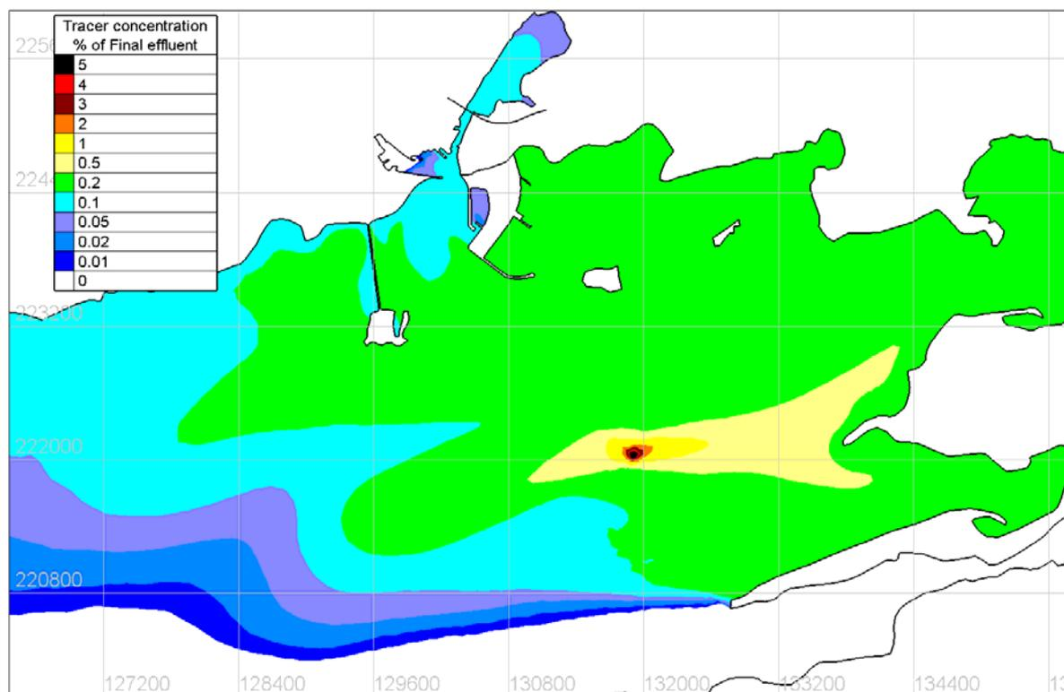
**Figure 4.8.62 Maximum surface concentration of Tracer under SE 15m/s wind conditions— Proposed**
