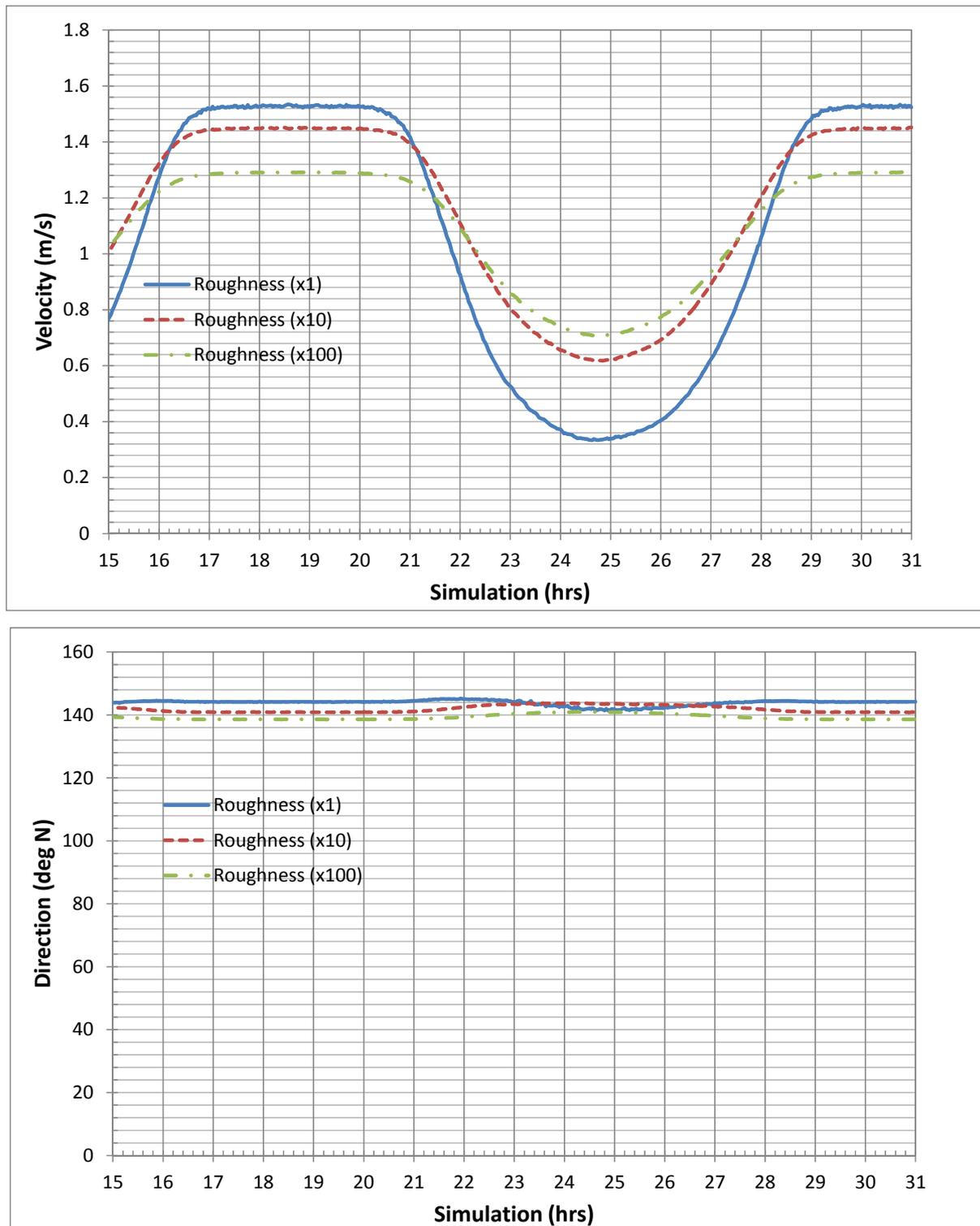
Figure 4.6.7 Sensitivity of Velocities to Roughness factor at Site 1
