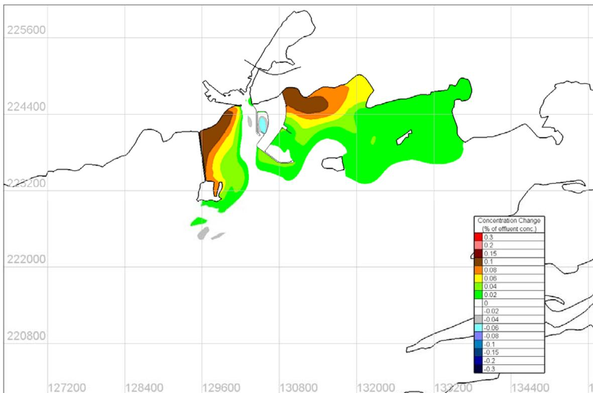
Figure 4.8.6 Predicted change in tidal mean tracer concentration – Calm Wind Conditions
