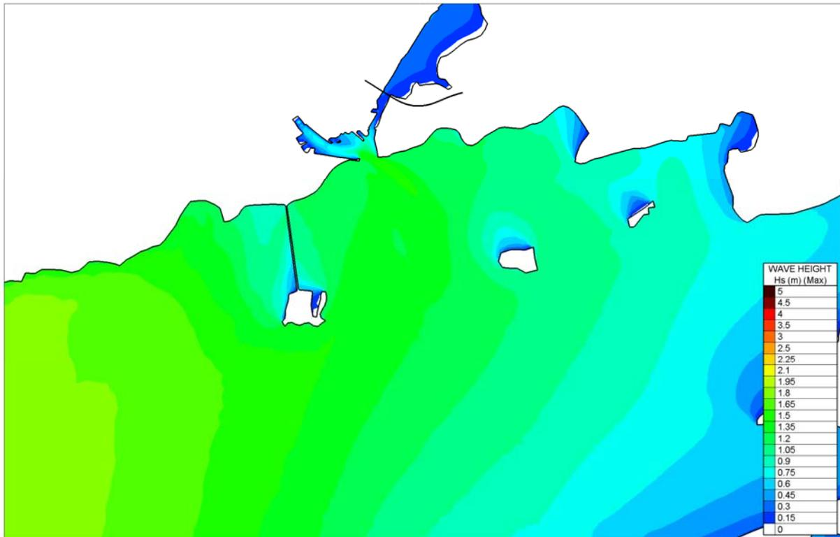
Figure 4.4.21 Computed Significant Wave heights for Local SE Storm Winds - Proposed
