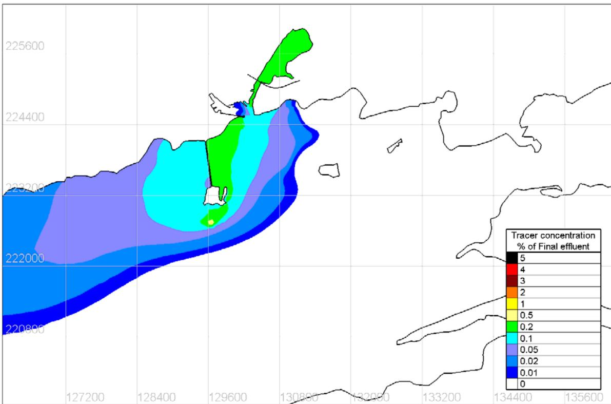
Figure 4.8.39 Tidal mean tracer concentration under S 15m/s wind conditions – Existing Case
