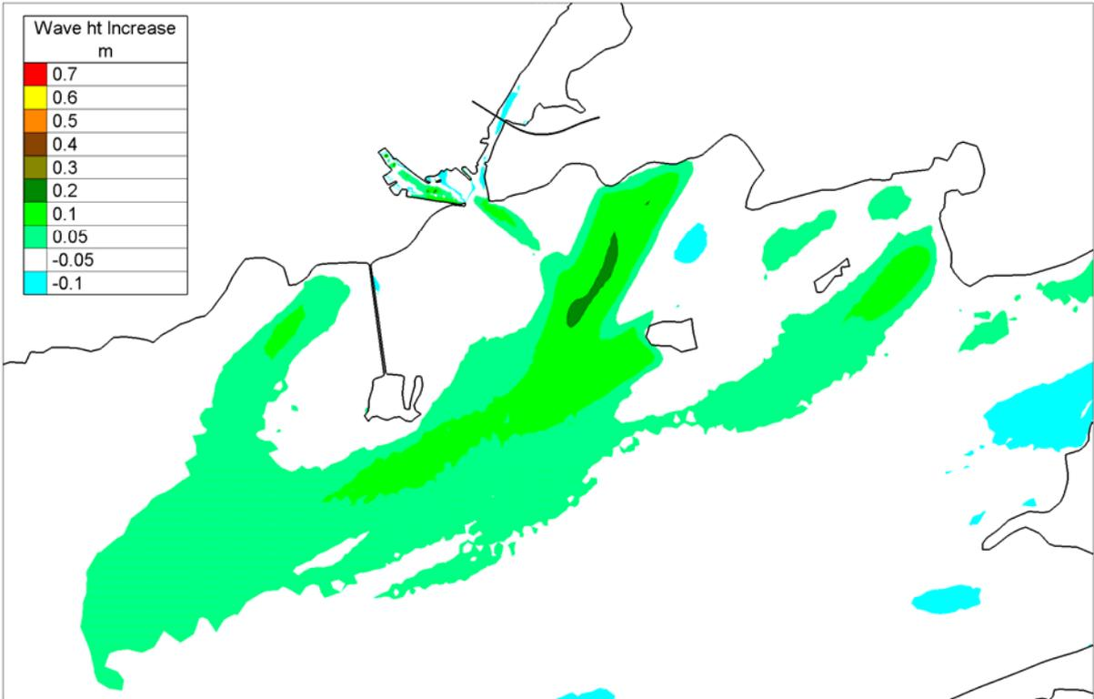
Figure 4.3.12 Difference Plot showing the effect of Tidal velocities on Wave height for SSW Storm wind conditions - Existing
