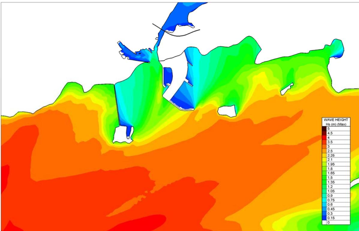
Figure 4.3.5 Predicted Wave Climate for SSW storm Wind with tidal velocities included - Proposed
