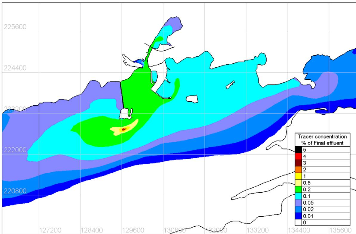
Figure 4.8.8 Maximum surface concentration of Tracer under under SW 5m/s wind conditions– Proposed
