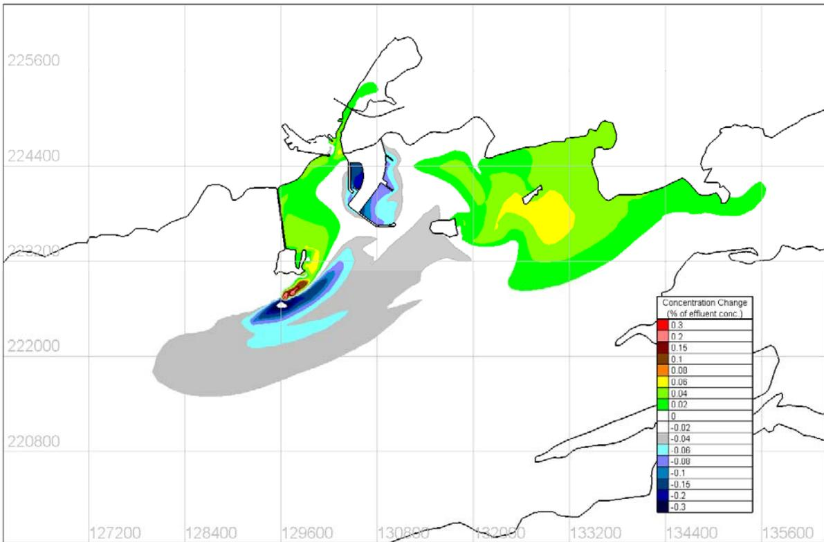
Figure 4.8.17 Predicted change in maximum surface tracer concentration – SSW 5m/s Wind Conditions
