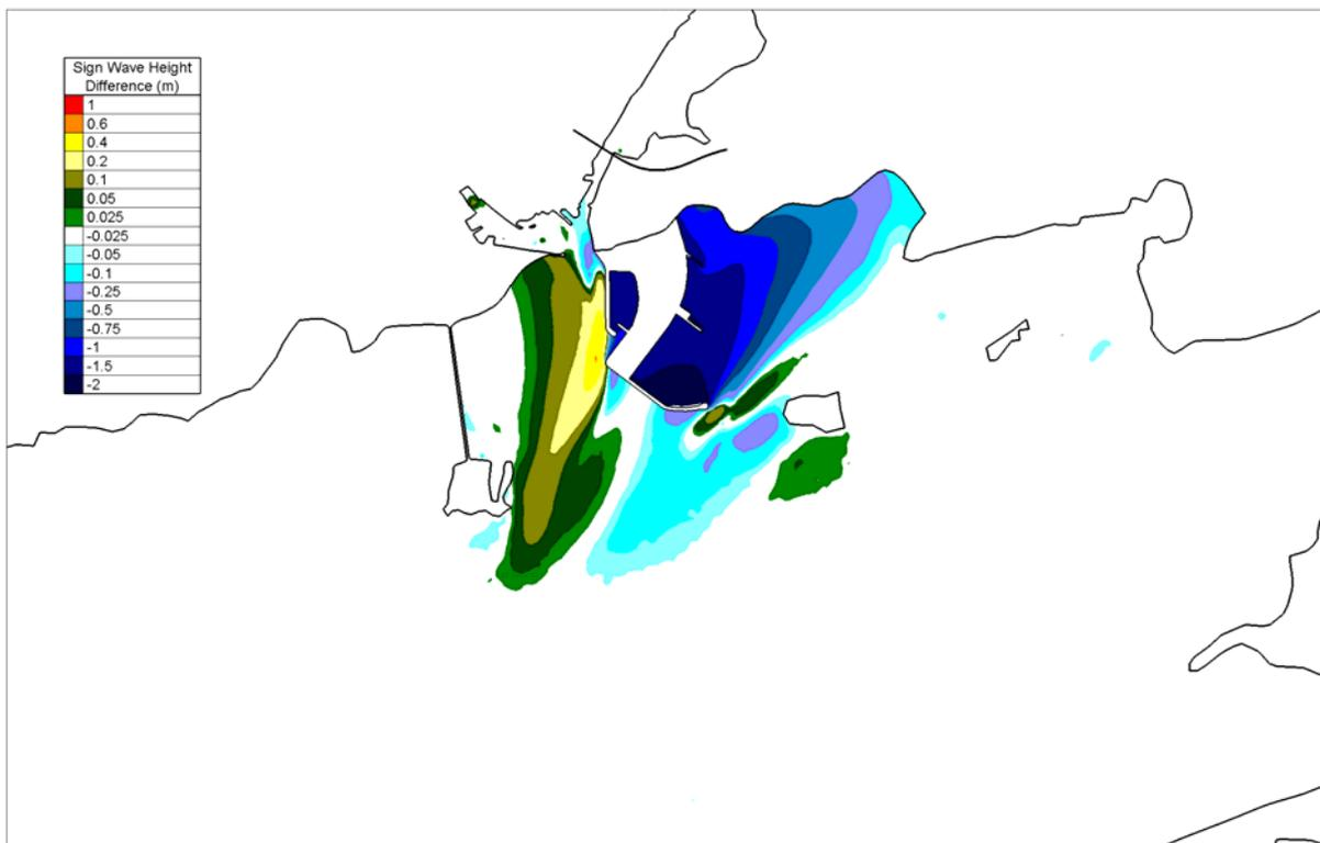
Figure 4.4.32 Difference Plot between Existing and Proposed Significant Wave heights for Local SSW Storm Winds
