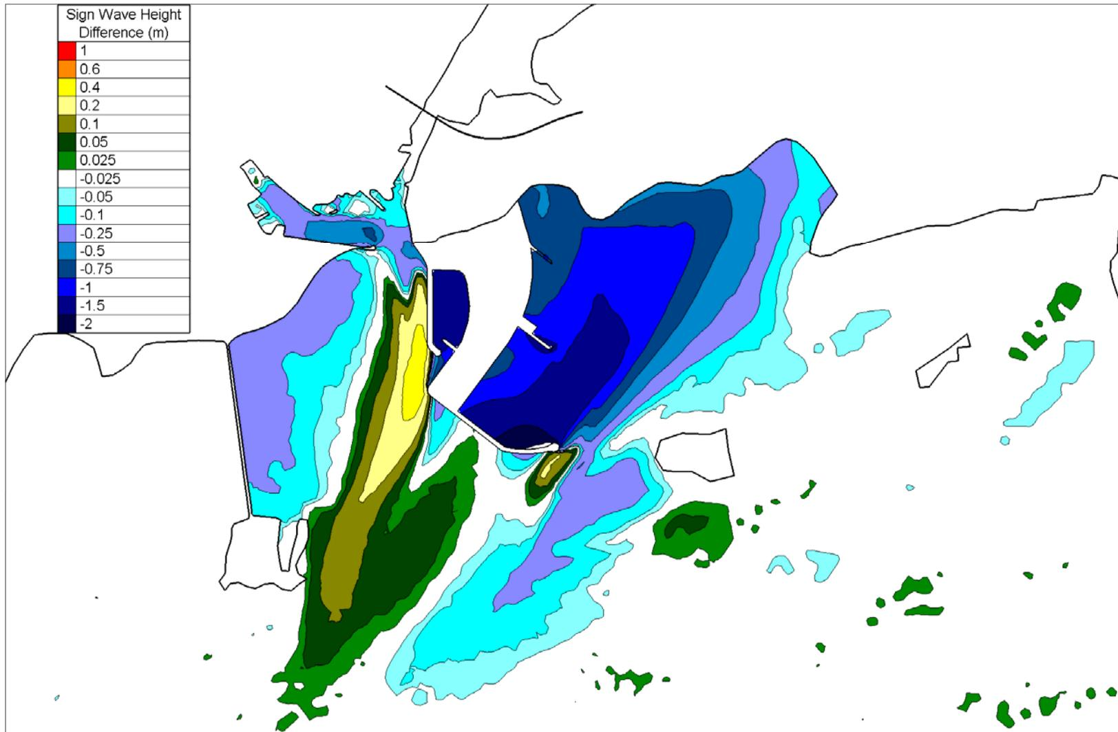
Figure 4.9.3 Difference plot of maximum predicted Wave heights existing and Proposed Wave climate for all onshore directions (West to ESE)
