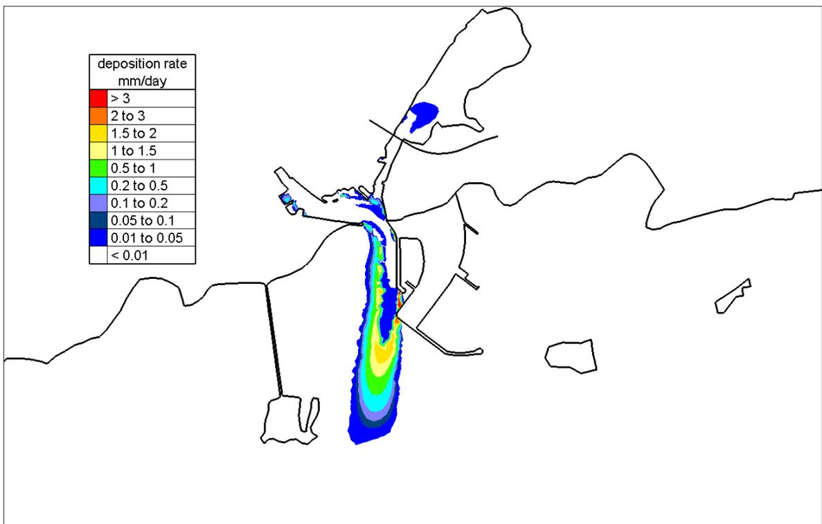
Figure 4.1.17 Computed depositional rates of a River Corrib fine sand under Winter flood flows (1-%ile 272cumec) - Proposed Case
