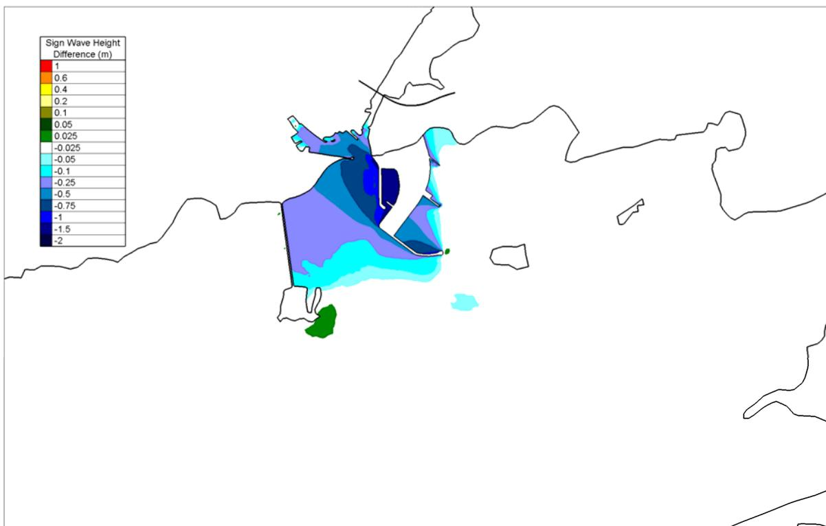
Figure 4.4.36 Difference Plot between Existing and Proposed Significant Wave heights for Local ESE Storm Winds
