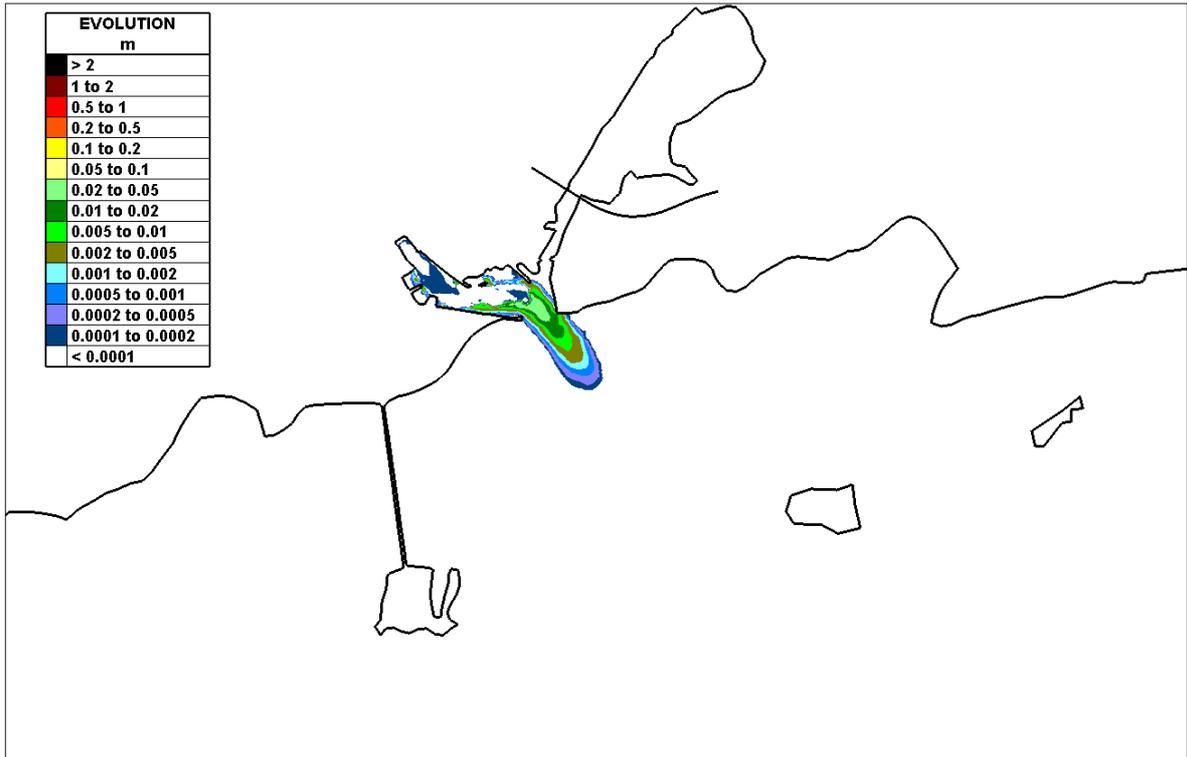
Figure 4.1.6 Deposition of Corrib fine sand under median flows at the end of 15 days - Existing Case
