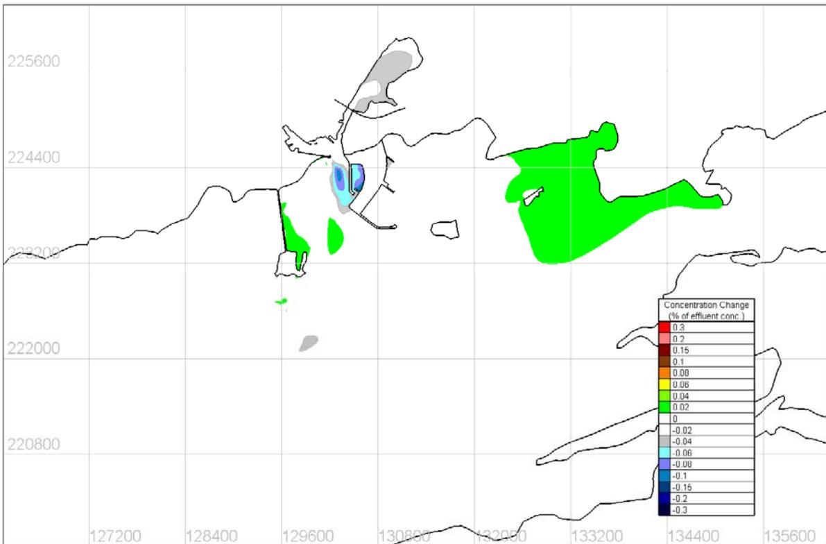
Figure 4.8.12 Predicted change in tidal mean tracer concentration – SW 5m/s Wind Condition
