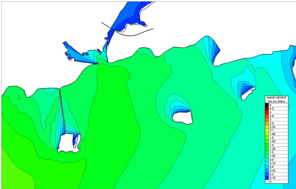
Figure 4.3.16 Predicted Wave Climate for local SE storm wind waves without tidal velocities included - Existing
