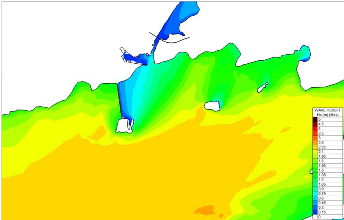
Figure 4.4.11 Computed Significant Wave heights for Local WSW Storm Winds - Existing
