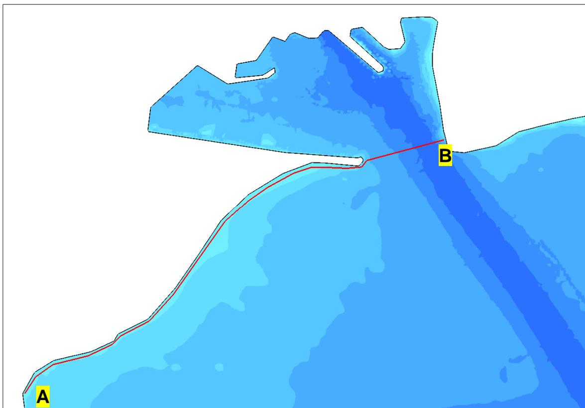
Figure 4.4.43 Shoreline Section A-B along Southpark, Nimmo's Pier and entrance to Galway Docks / Claddagh Basin.
