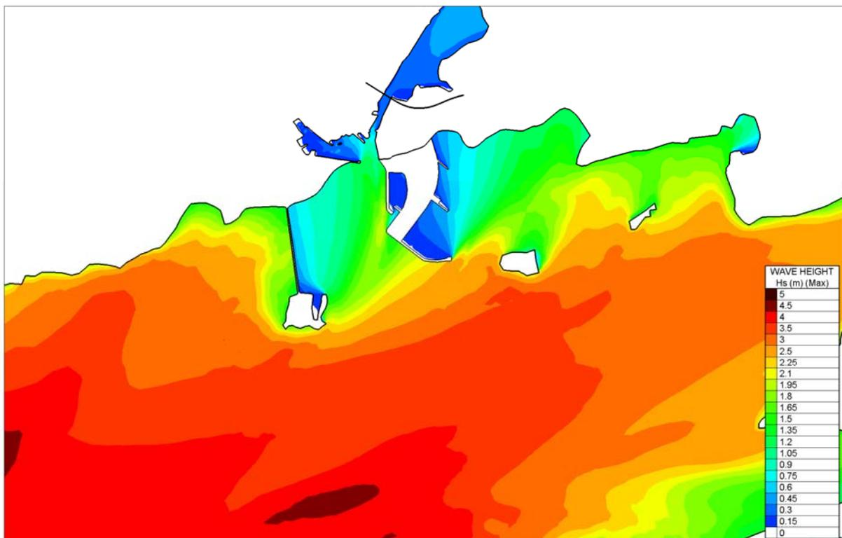
Figure 4.4.6 Computed Significant Wave heights for Atlantic Storm and SW
