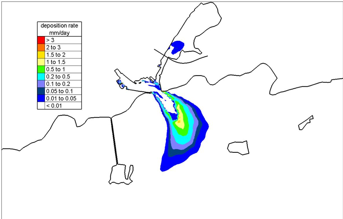
Figure 4.1.16 Computed depositional rates of a River Corrib fine sand under Winter flood flows (1-%ile 272cumec) - Existing Case.
