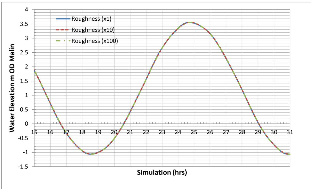
Figure 4.6.5 Sensitivity of elevation to Roughness factor at Site 4
