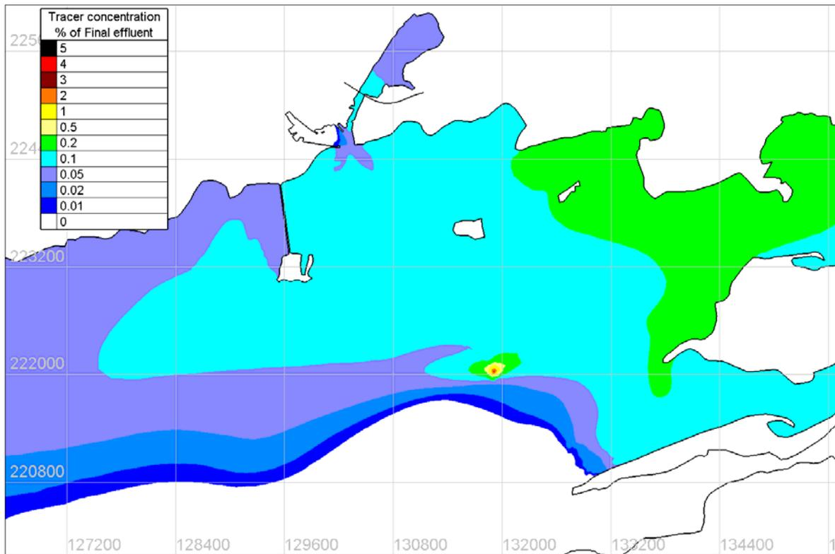
Figure 4.8.57 Tidal mean tracer concentration under S 15m/s wind conditions – Existing Case
