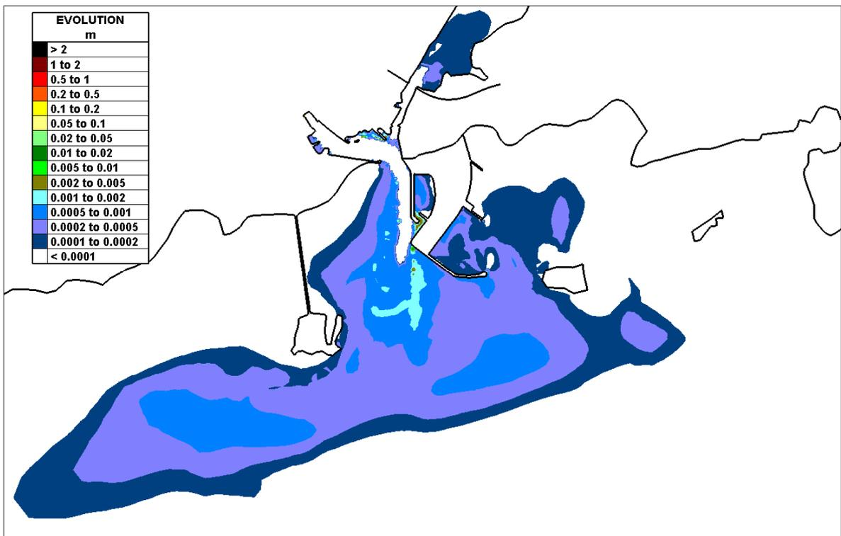
Figure 4.1.11 Deposition of a Corrib fine silt under winter flows (272cume) at the end of 15 days Simulation - Proposed Case
