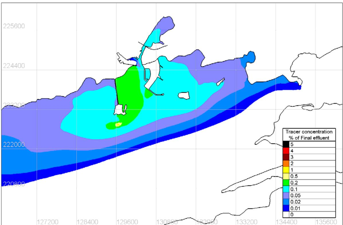
Figure 4.8.22 Tidal mean tracer concentration under South 5m/s wind conditions – Proposed Case
