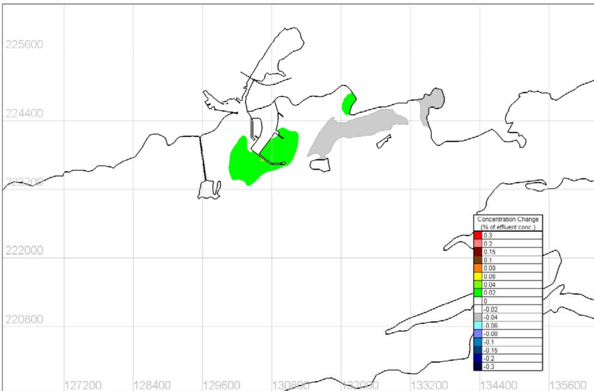
Figure 4.8.30 Predicted change in tidal mean tracer concentration – SW 15m/s Wind Condition
