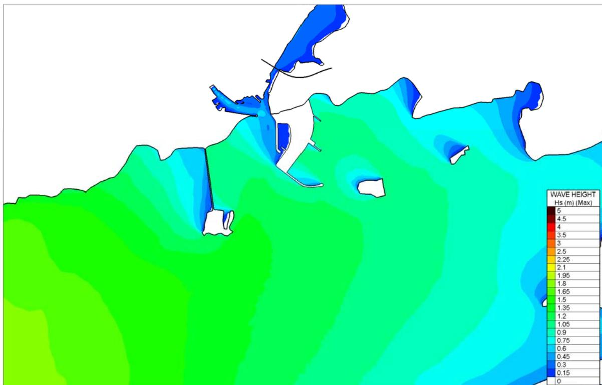
Figure 4.4.24 Computed Significant Wave heights for Local ESE Storm Winds - Proposed
