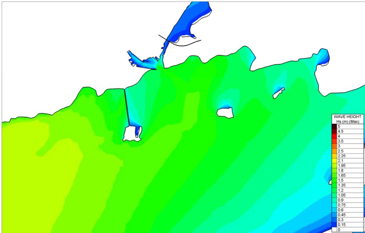
Figure 4.4.19 Computed Significant Wave heights for Local SSE Storm Winds - Existing
