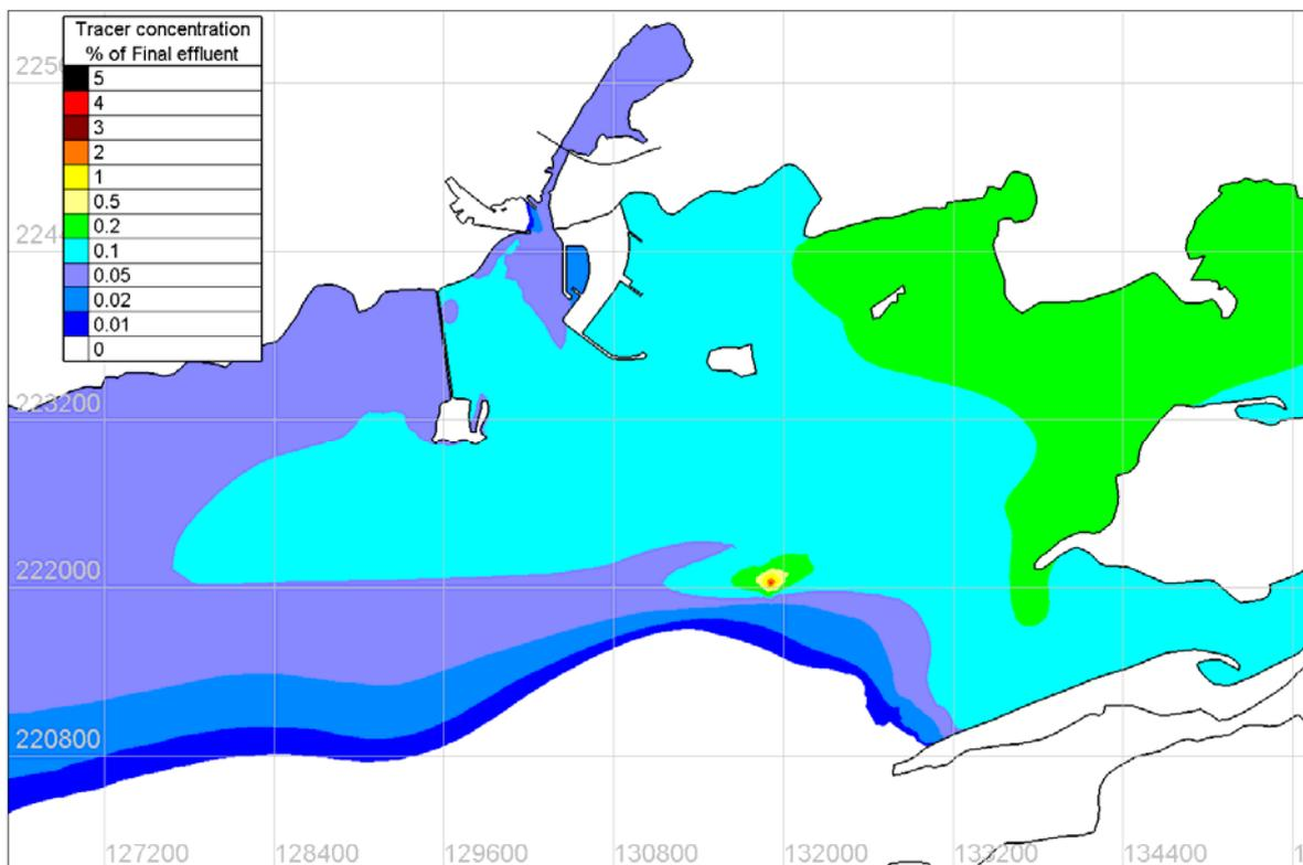
Figure 4.8.58 Tidal mean tracer concentration under S 15m/s wind conditions – Proposed Case
