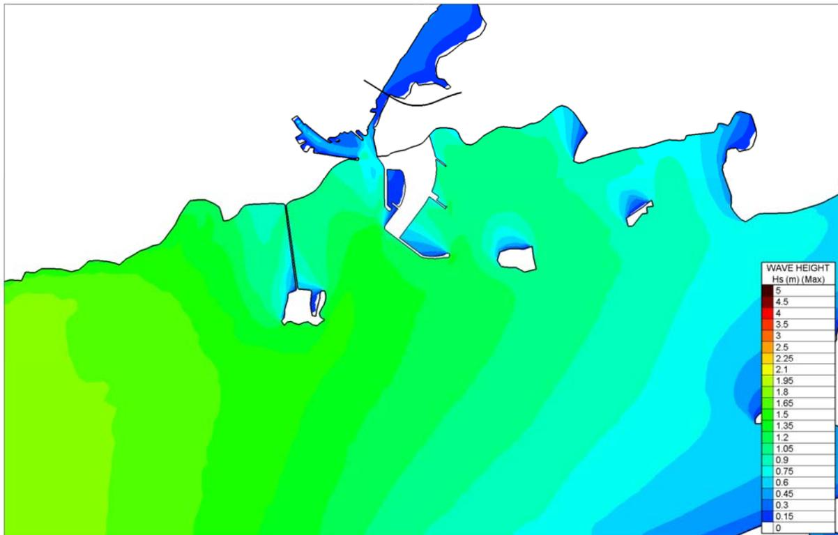
Figure 4.4.22 Computed Significant Wave heights for Local SE Storm Winds - Proposed
