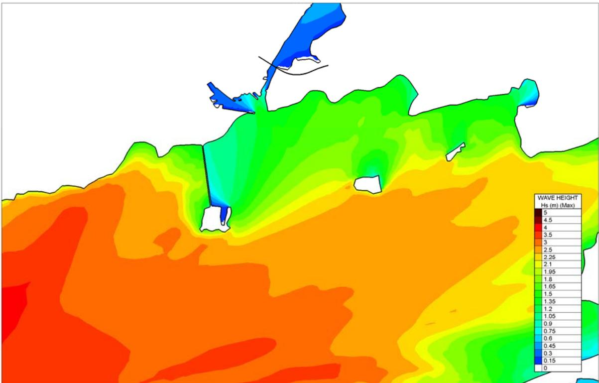
Figure 4.3.13 Predicted Wave Climate for South storm winds without including tidal velocities - Existing
