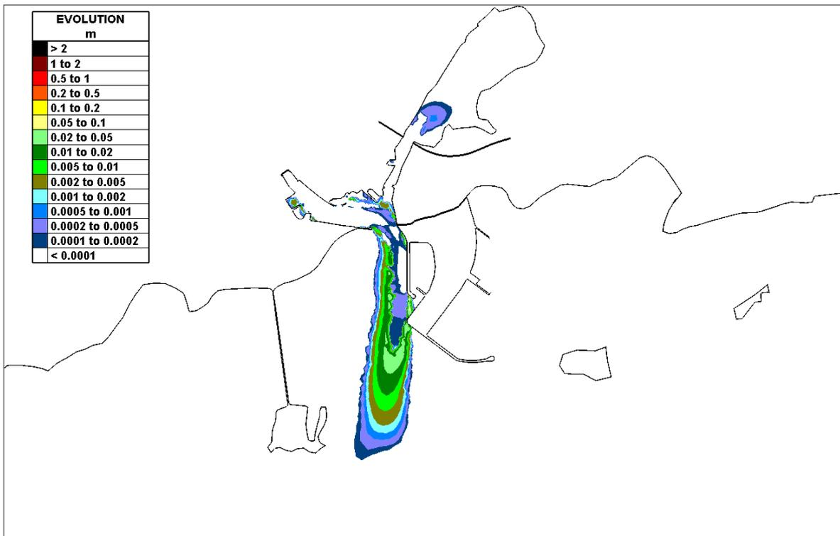
Figure 4.1.15 Deposition of a Corrib fine sand under winter flows (272cumec) at the end of 15 days Simulation - Proposed Case
