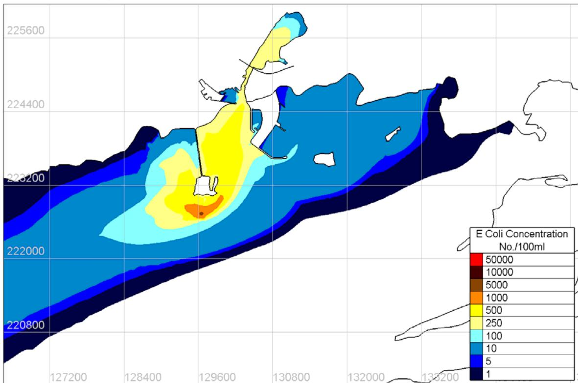
Figure 4.8.47 Maximum surface coliform concentration of Tracer under SSW 15m/s wind conditions– Proposed
