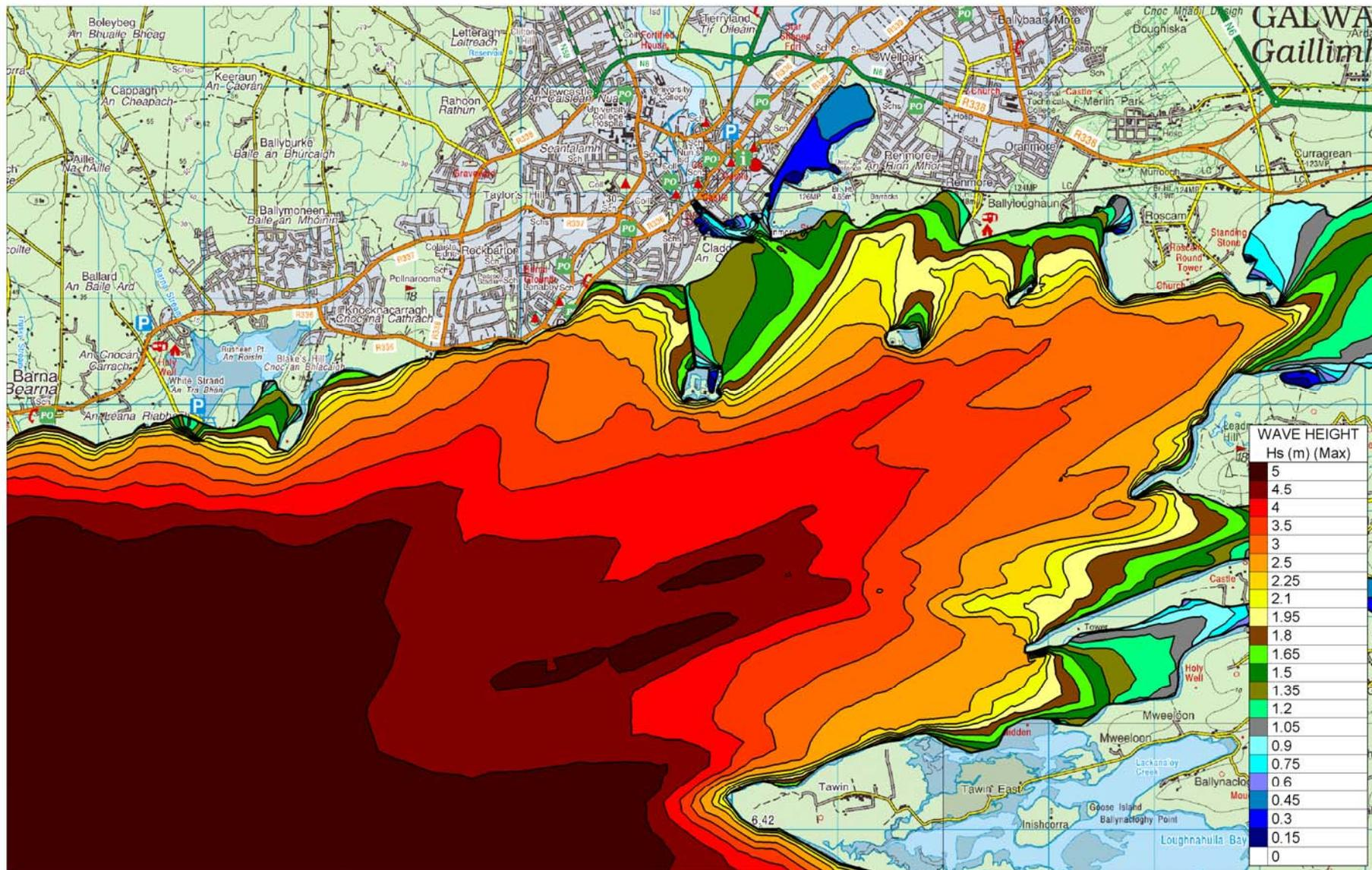
Figure 4.9.1 Shows maximum wave heights within the bay, existing case
