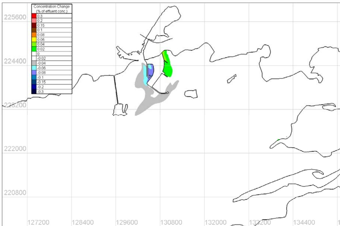
Figure 4.8.60 Predicted change in tidal mean tracer concentration – S 15m/s Wind Condition
