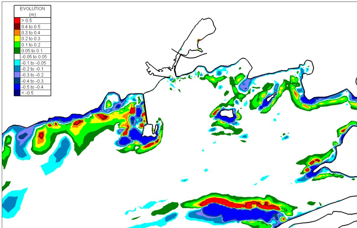
Figure 4.1.18 South Storm Waves Simulation modelling a fine sand - Existing Case
