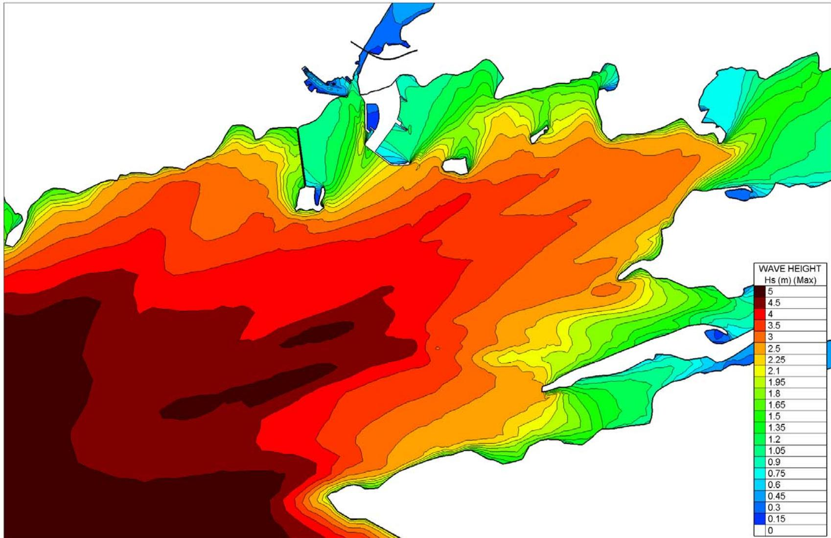
Figure 4.4.38 Computed Maximum Significant Wave Heights – Proposed Harbour Case (all on shore directions W to ESE combined local and Atlantic storm swell wave climate runs)
