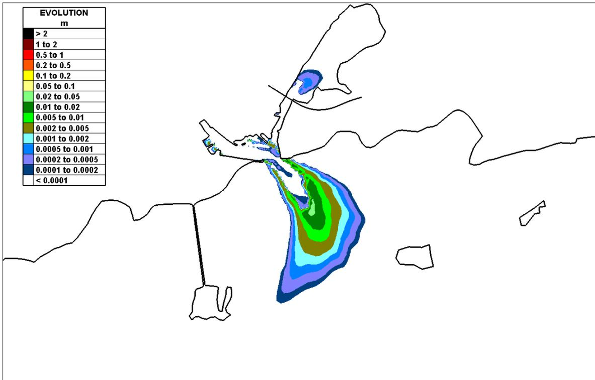
Figure 4.1.14 Deposition of a Corrib fine sand under winter flows (272cumec) at the end of 15 days Simulation - Existing Case
