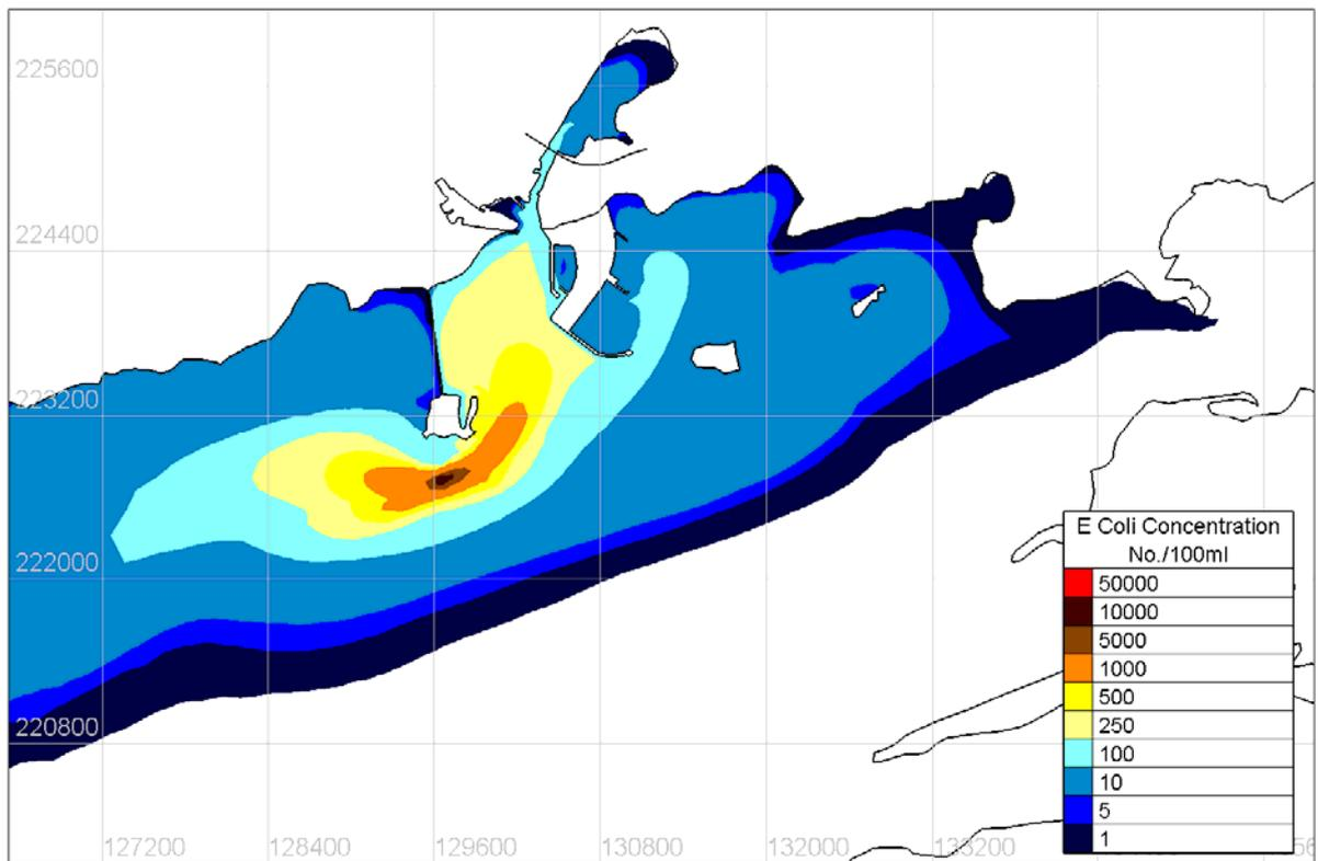
Figure 4.8.44 Maximum faecal coliform surface concentration under Calm wind conditions– Proposed
