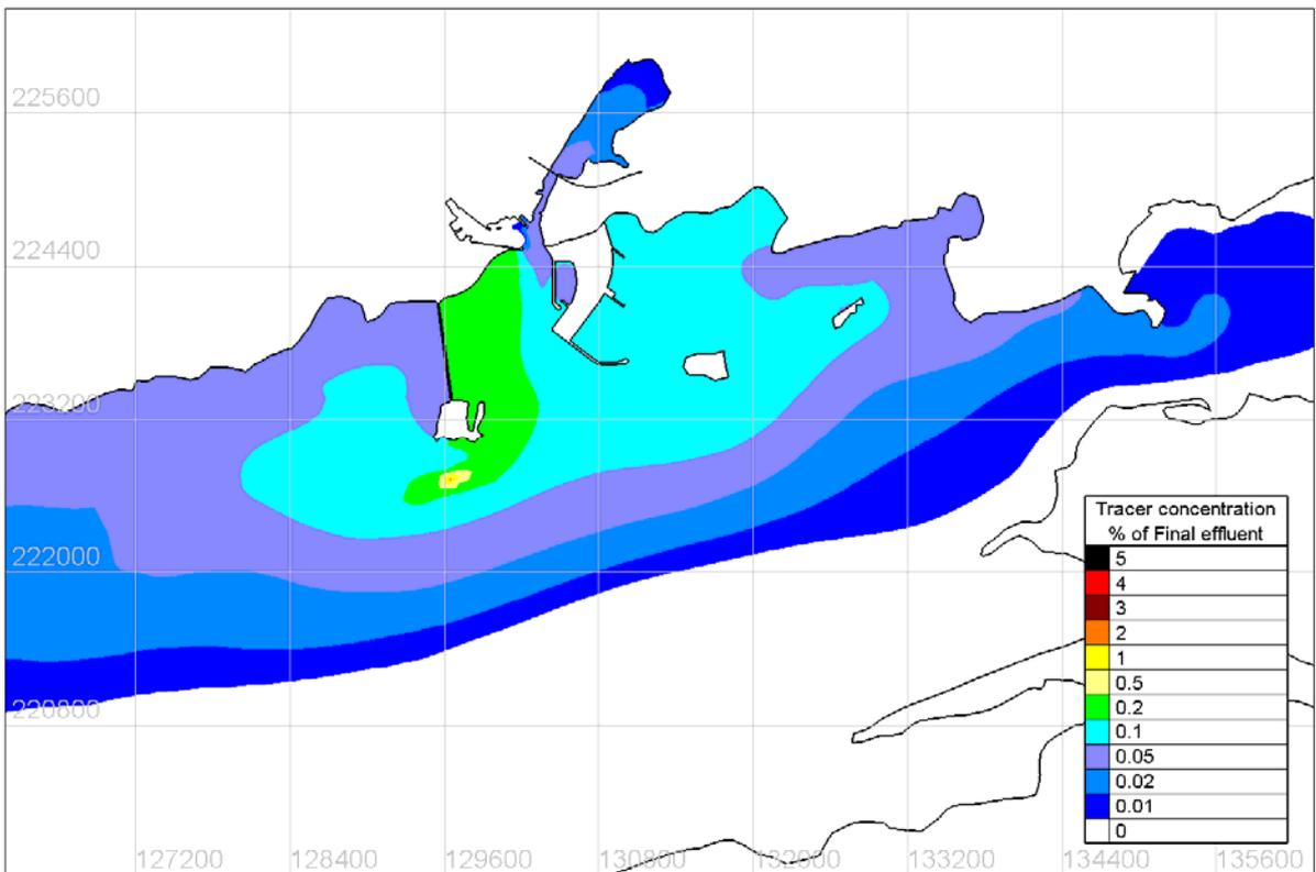
Figure 4.8.4 Tidal mean tracer concentration under calm wind conditions – Proposed Case
