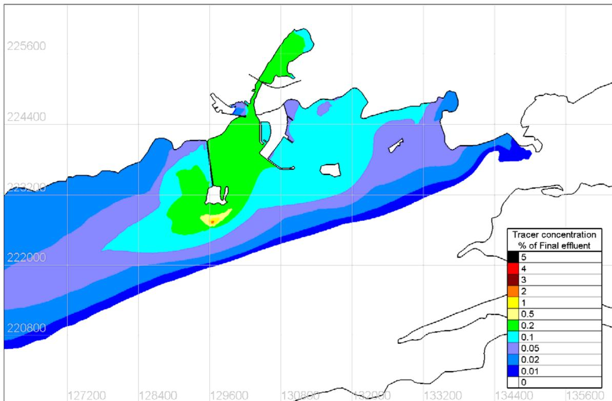
Figure 4.8.32 Maximum surface concentration of Tracer under SSW 15m/s wind conditions– Proposed
