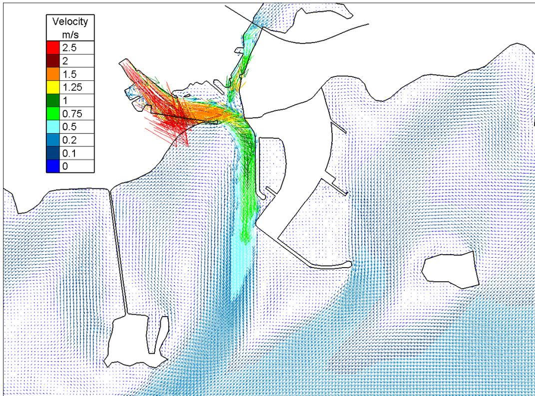
Figure 4.3.1 Snapshot of opposing flow and tidal velocities for Corrib 100year flood flow and spring tides with the Harbour Development
