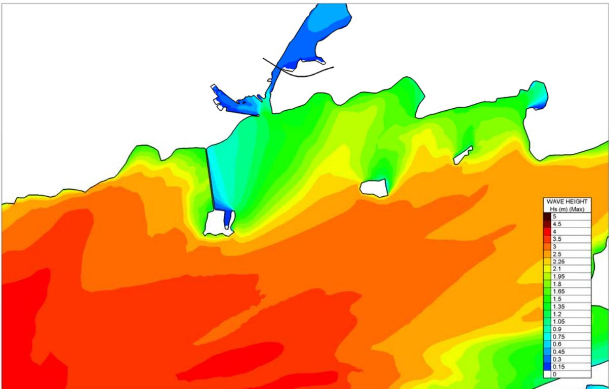
Figure 4.3.11 Predicted Wave Climate for SSW storm Wind with tidal velocities included - Existing
