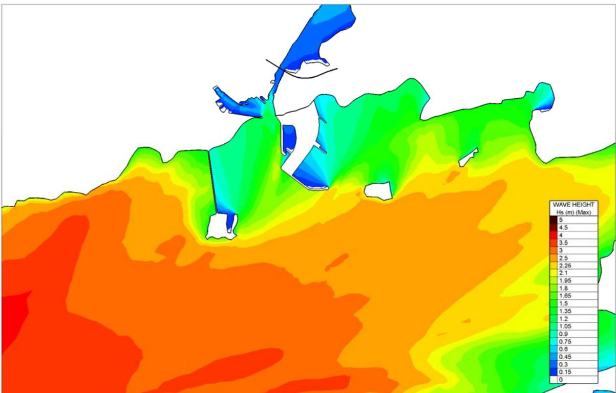
Figure 4.3.8 Predicted Wave Climate for South storm winds with tidal velocities included - Proposed
