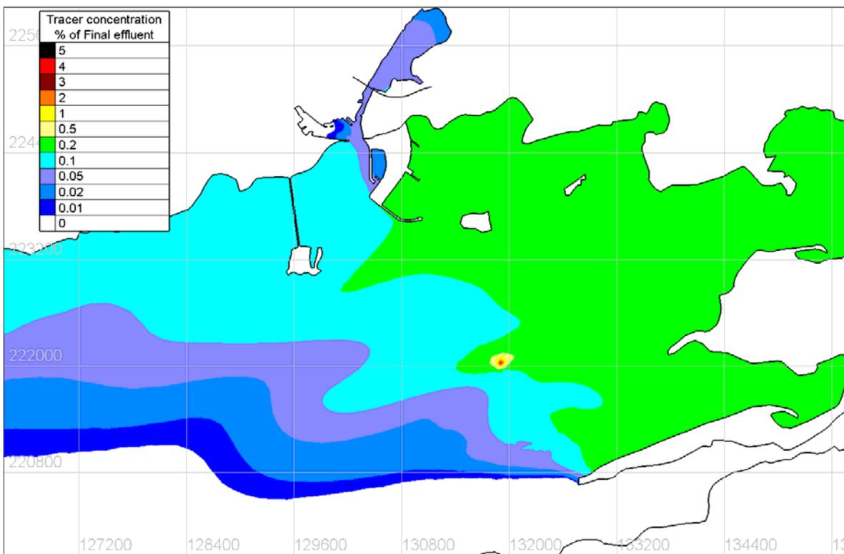
Figure 4.8.64 Tidal mean tracer concentration under SE 15m/s wind conditions – Proposed Case
