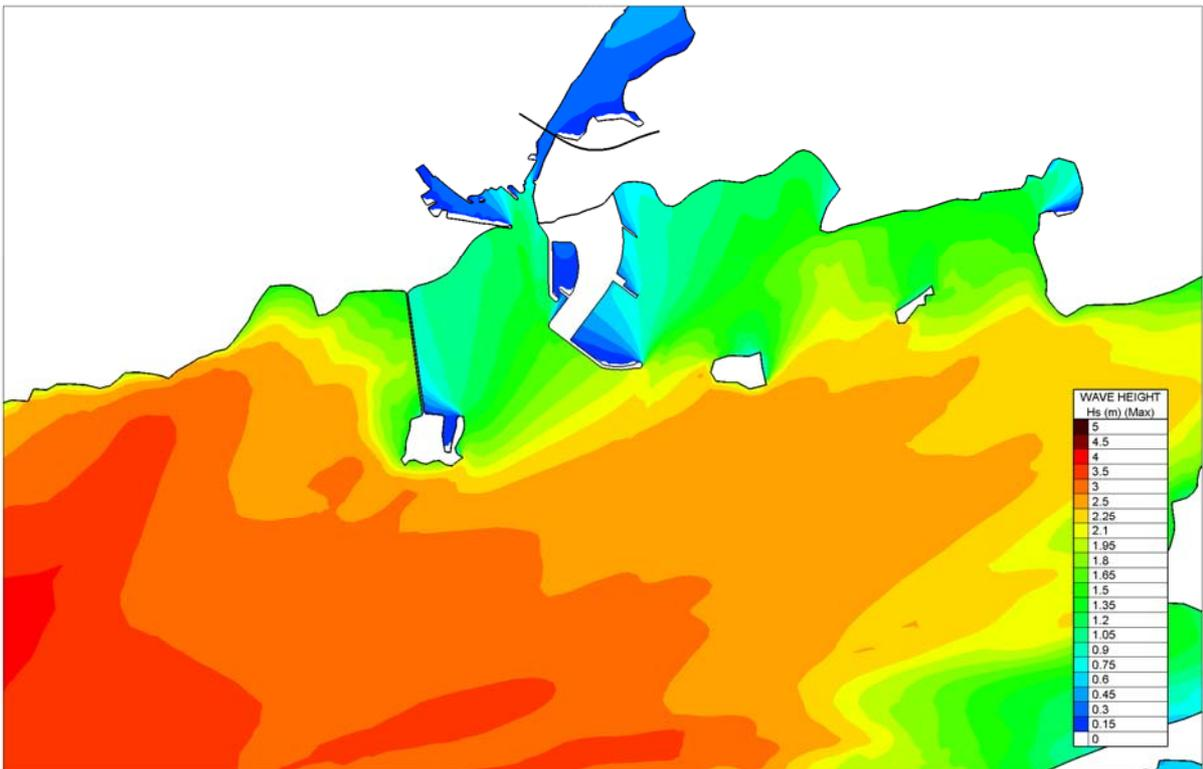
Figure 4.3.7 Predicted Wave Climate for South storm winds without including tidal velocities - Proposed
