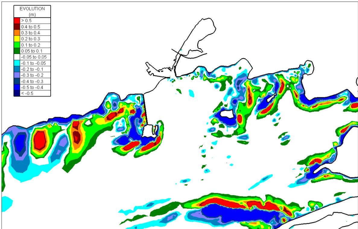
Figure 4.1.20 Southwest Storm Waves Simulation modelling a fine sand - Existing Case
