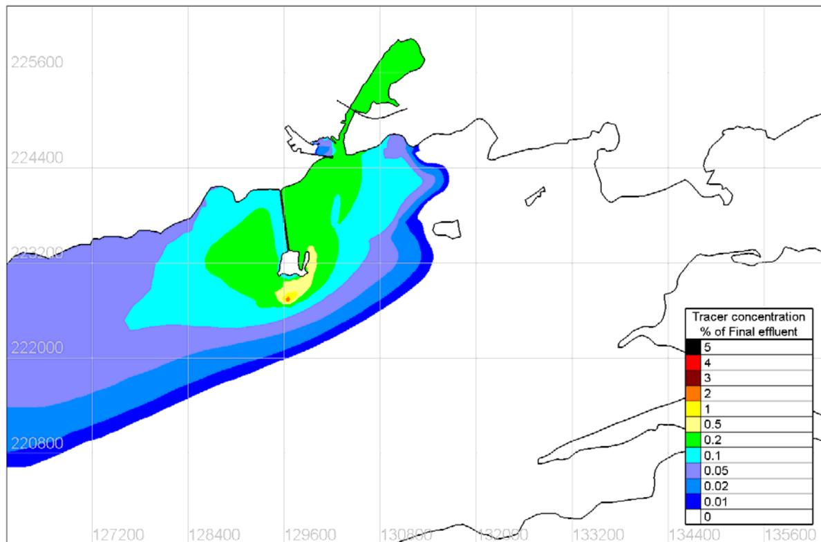
Figure 4.8.37 Maximum surface concentration of Tracer under S 15m/s wind conditions– Existing
