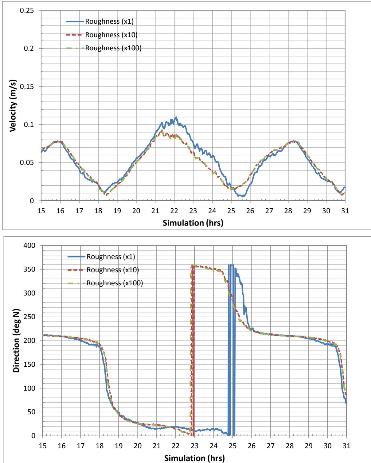
Figure 4.6.11 Sensitivity of Velocities to Roughness factor at Site 5
