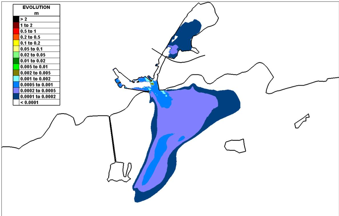
Figure 4.1.2 Deposition of a Corrib silt under median flows at the end of 15 days - Existing Case (the white area within the Claddagh Basin and Lough Atalia channel is self-cleansing).
