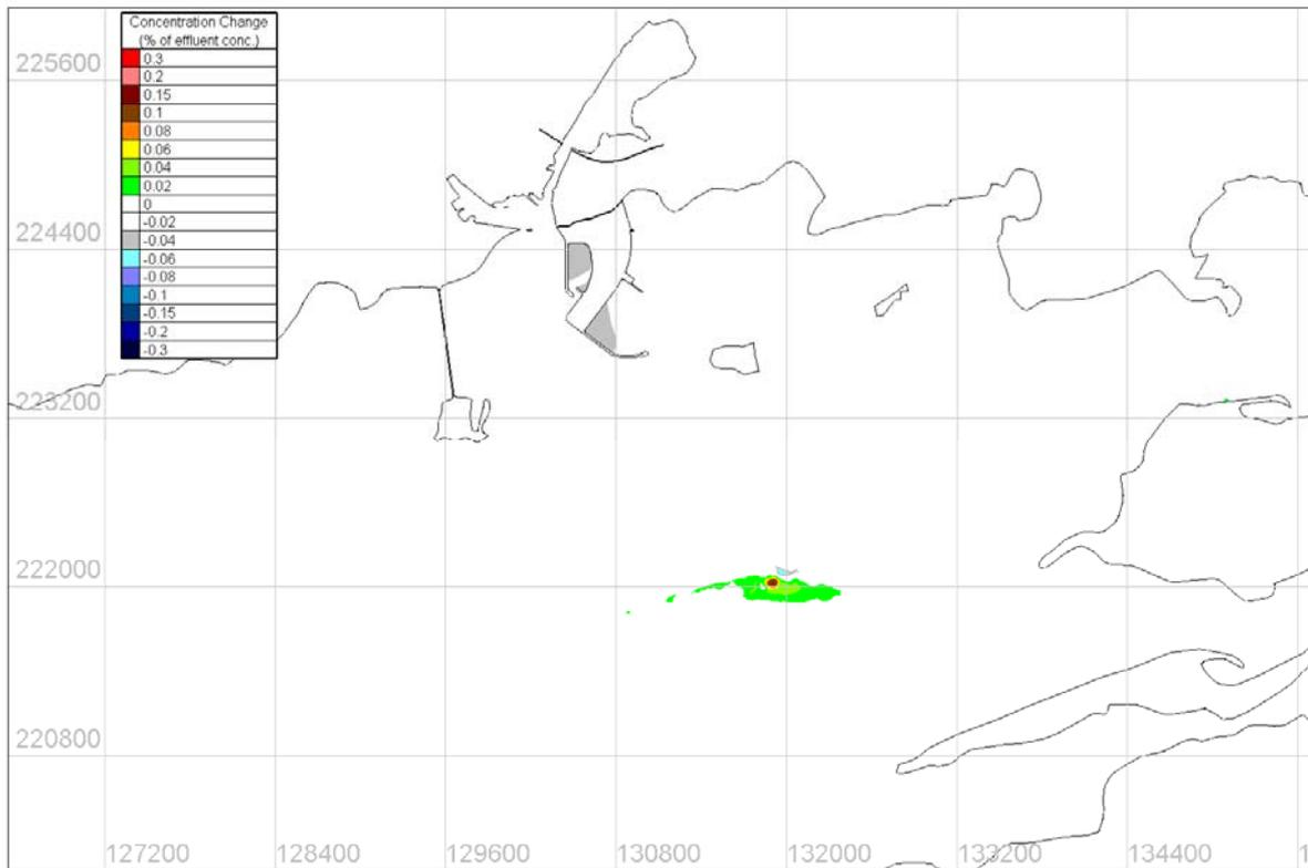
Figure 4.8.53 Predicted change in maximum surface tracer concentration – SW 15m/s Wind Conditions
