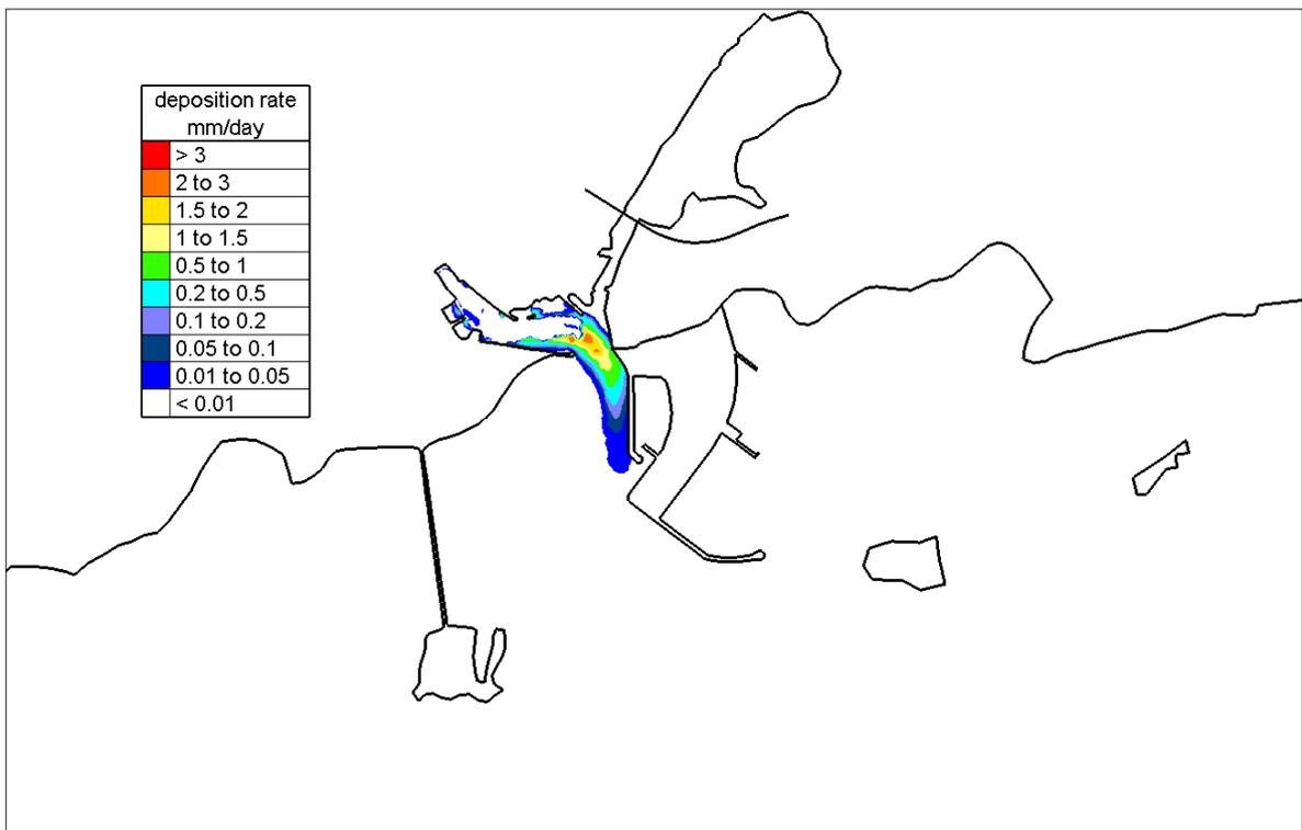
Figure 4.1.9 Computed depositional rates of a River Corrib fine sand under median flows - Proposed Case
