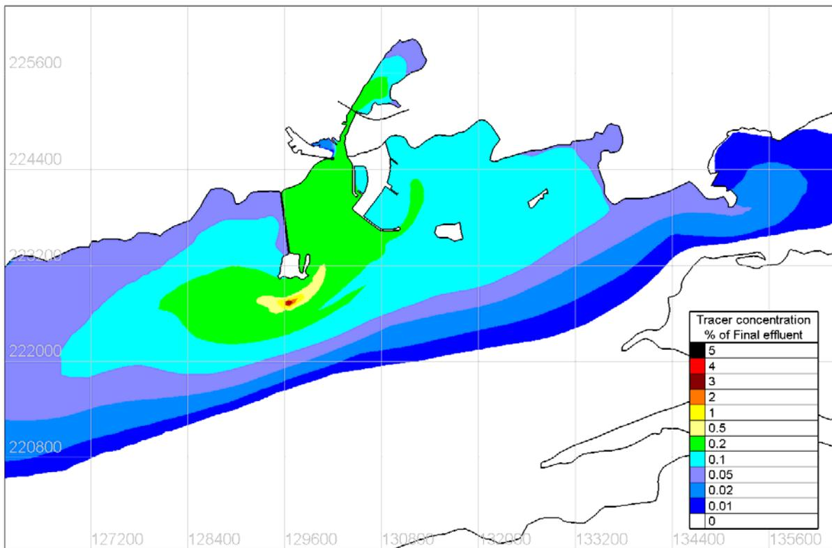
Figure 4.8.14 Maximum surface concentration of Tracer under SSW 5m/s wind conditions– Proposed
