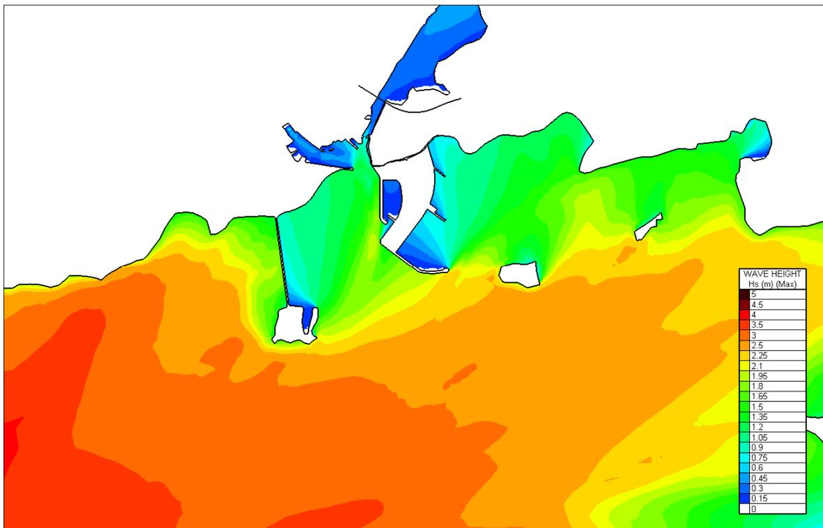
Figure 4.4.10 Computed Significant Wave heights for Atlantic Storm and South Storm Winds - Proposed
