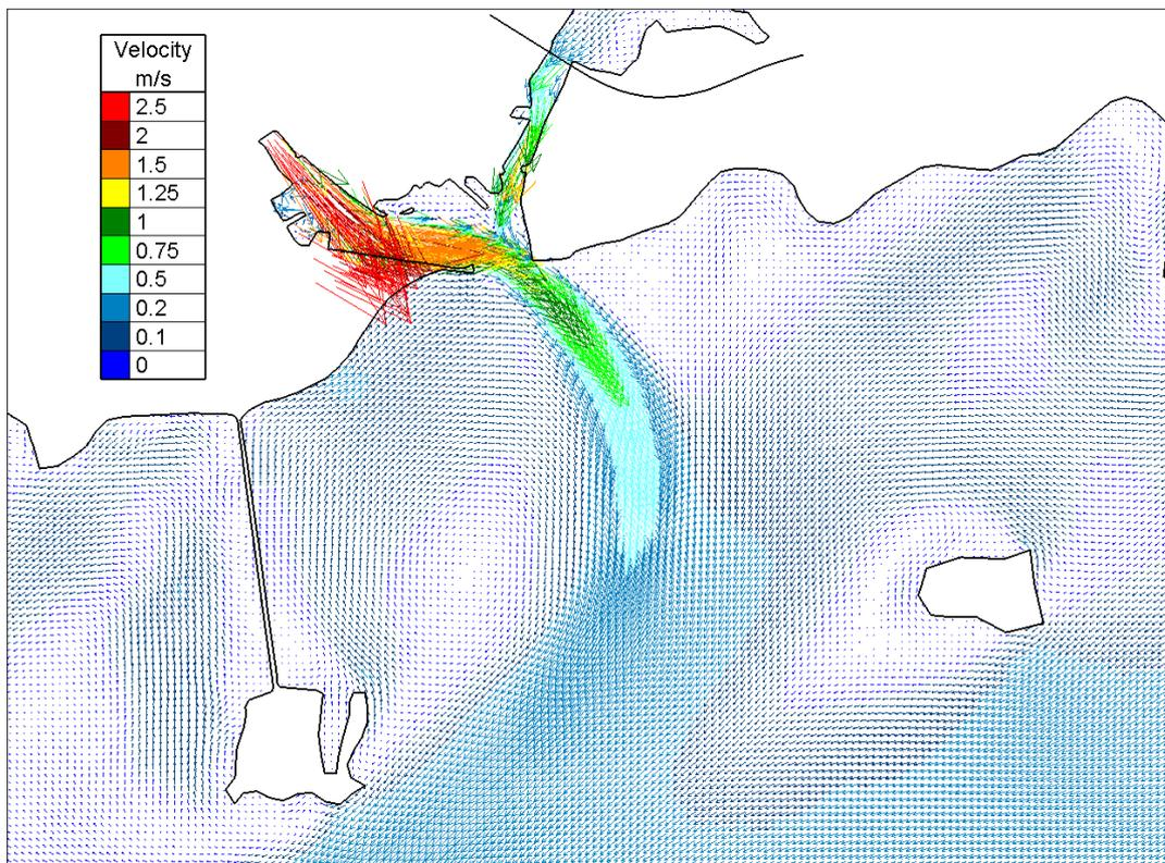
Figure 4.3.2 Snapshot of opposing flow and tidal velocities for Corrib 100year flood flow and spring tides without the Harbour Development (existing Case)
