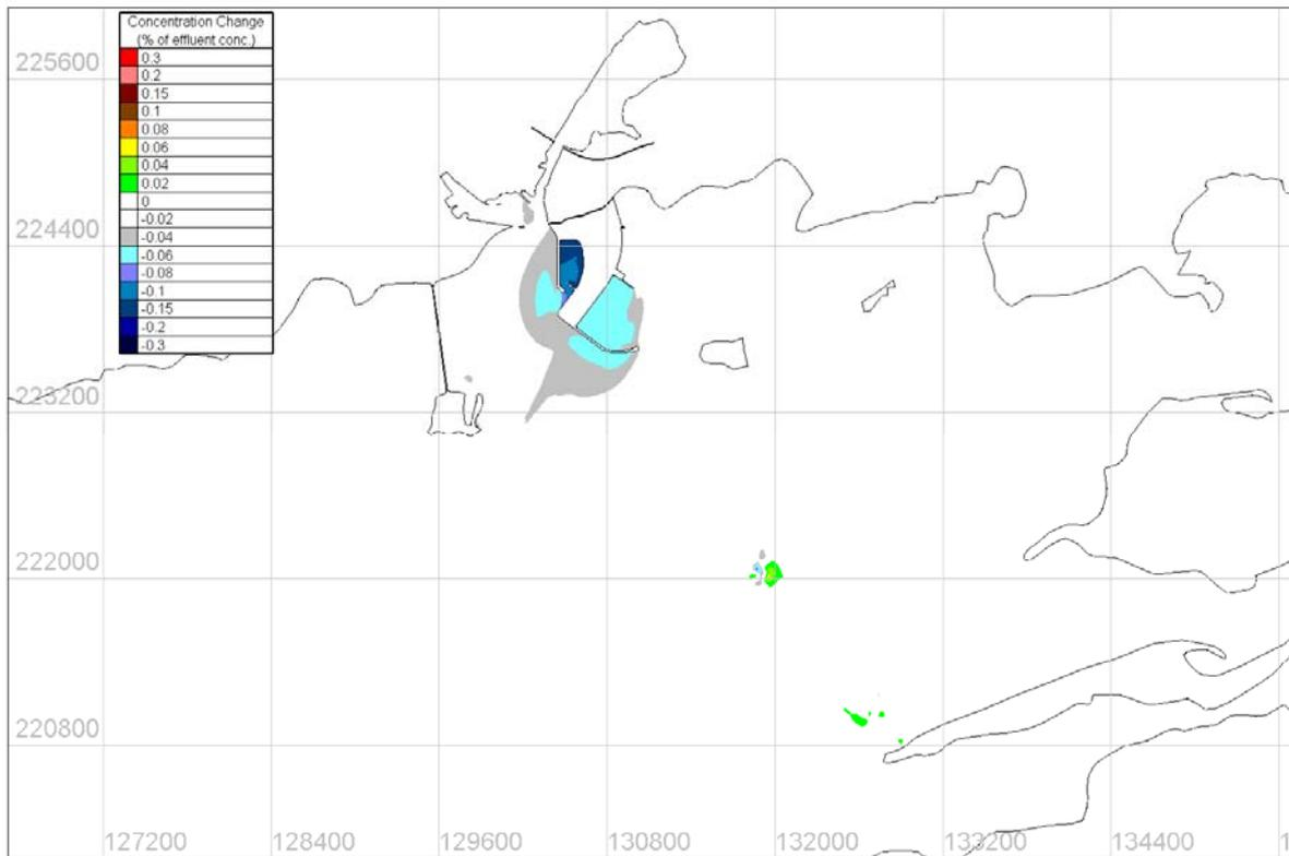
Figure 4.8.59 Predicted change in maximum surface tracer concentration – S 15m/s Wind Conditions
