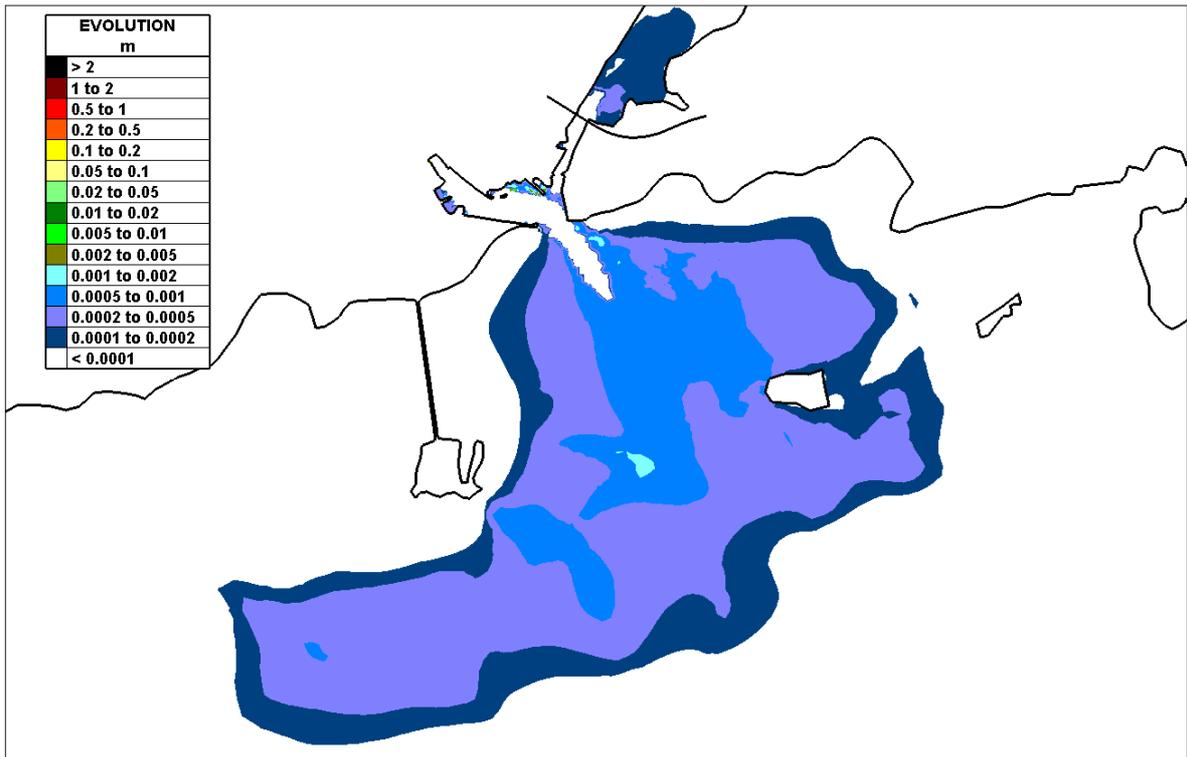
Figure 4.1.10 Deposition of a Corrib fine silt under winter flows (272cume) at the end of 15 days Simulation - Existing Case
