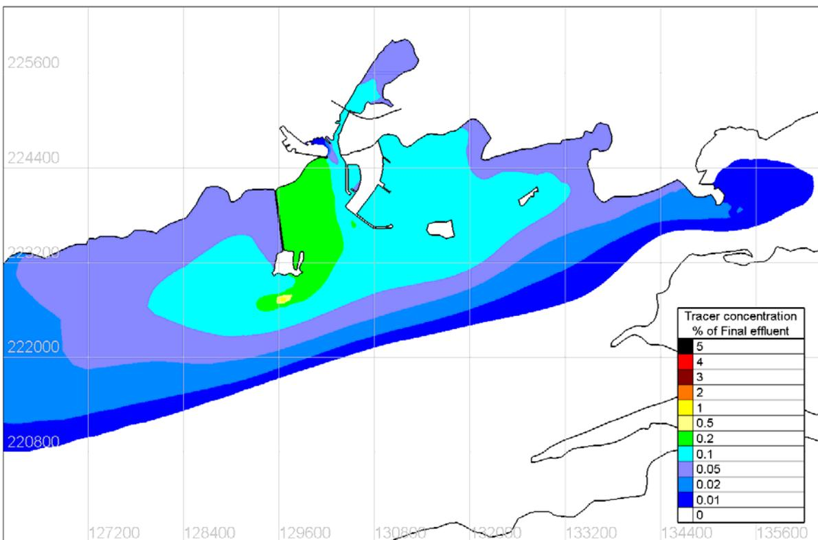
Figure 4.8.16 Tidal mean tracer concentration under SSW 5m/s wind conditions – Proposed Case
