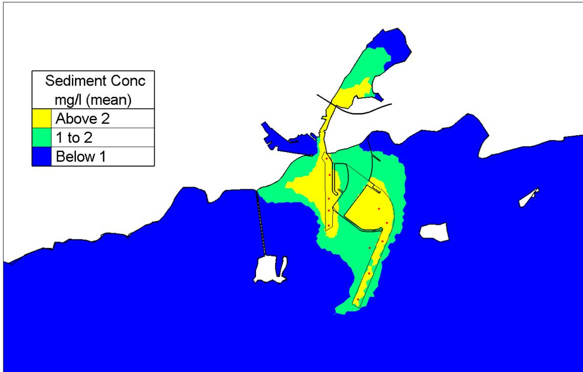
Figure 4.1.22 Capital Dredge Sediment concentrations extrapolation from sediment transport results from EIS Figures 8.4.42 to 8.4.49 and 8.4.51 to 8.4.57 representing the unmitigated case
