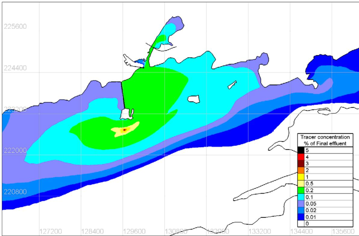
Figure 4.8.7 Maximum surface concentration of Tracer under under SW 5m/s wind conditions– Existing
