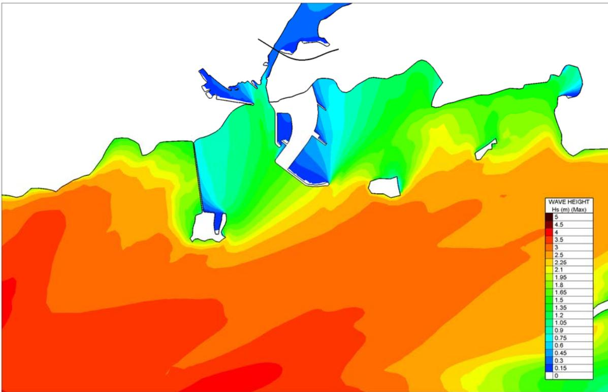
Figure 4.3.4 Predicted Wave Climate for SSW storm Wind without including tidal velocities - Proposed
