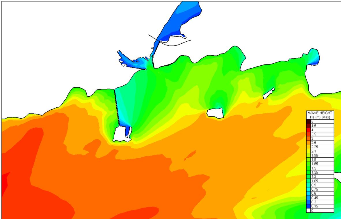
Figure 4.4.9 Computed Significant Wave heights for Atlantic Storm and South Storm Winds - Existing
