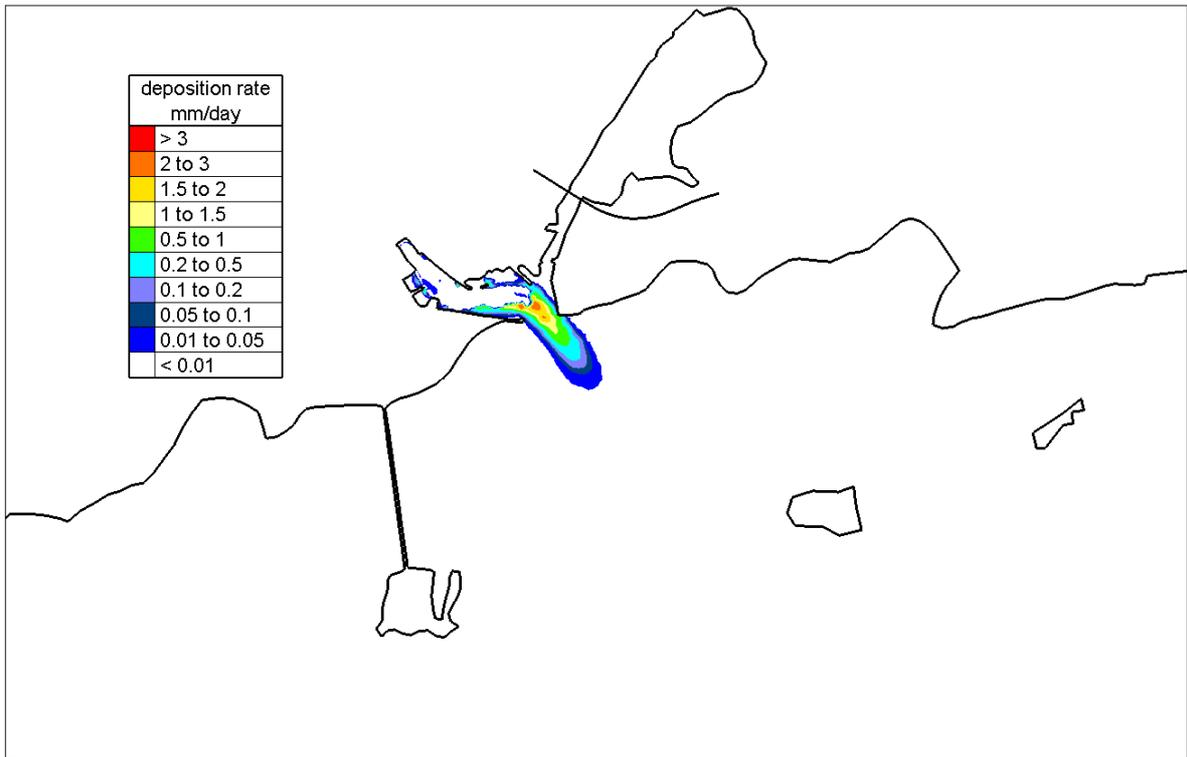
Figure 4.1.8 Computed Depositional Rates of a River Corrib fine sand under median flows - Existing Case
