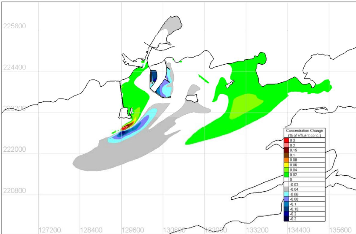
Figure 4.8.11 Predicted change in maximum surface tracer concentration – SW 5m/s Wind Conditions
