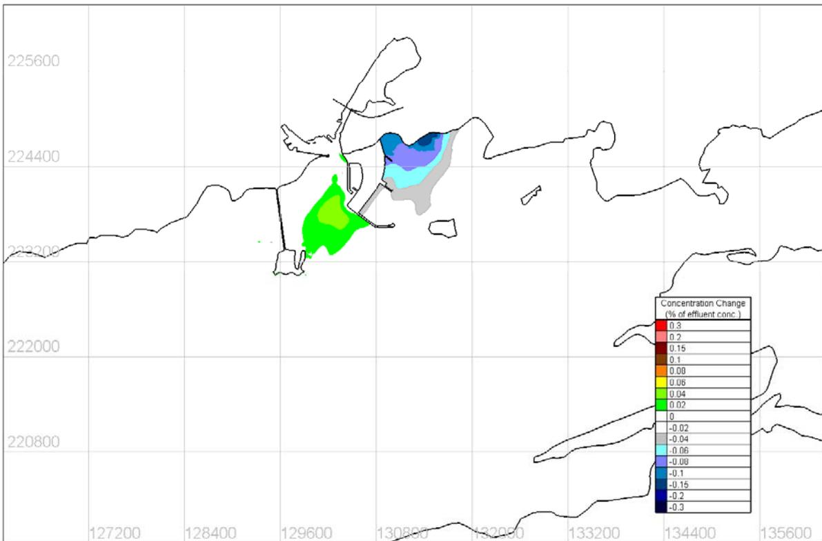
Figure 4.8.36 Predicted change in tidal mean tracer concentration – SSW 15m/s Wind Condition
