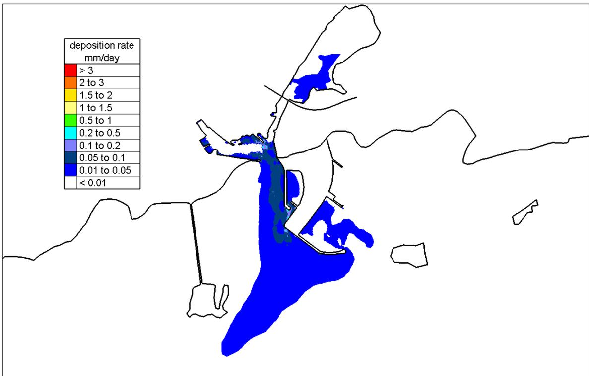
Figure 4.1.5 Computed Depositional Rates of River Corrib fine silt under median flows for Proposed Case.
