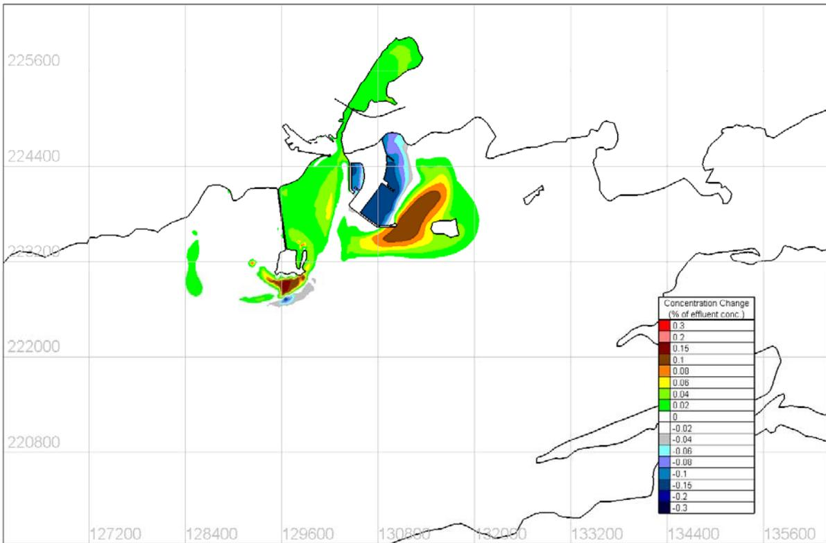
Figure 4.8.41 Predicted change in maximum surface tracer concentration – S 15m/s Wind Conditions
