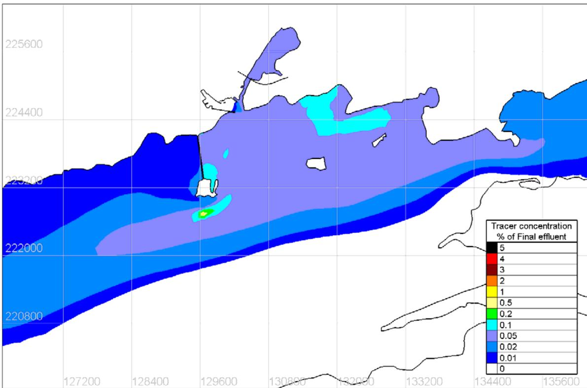
Figure 4.8.27 Tidal mean tracer concentration under SW 15m/s wind conditions – Existing Case
