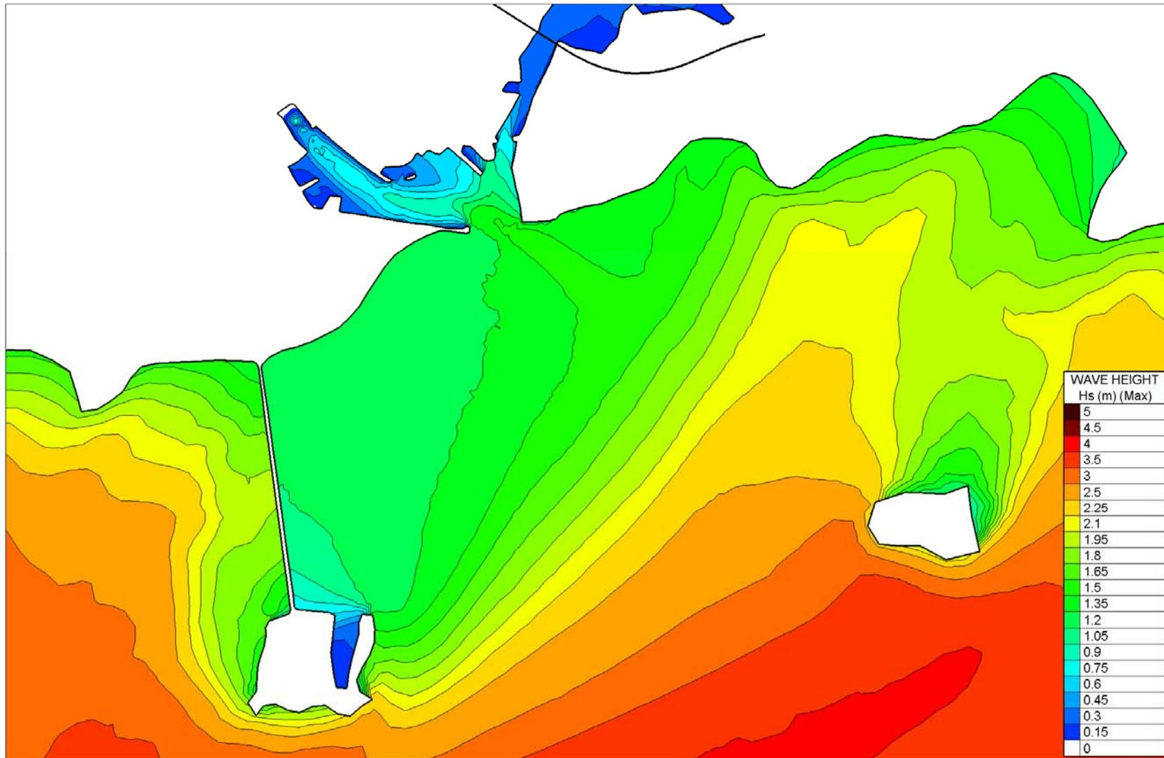
Figure 4.4.39 Computed Maximum Significant Wave Heights – Existing Case (all on shore directions W to ESE) – Harbour Area (Close up of Fig 4.4.37).
