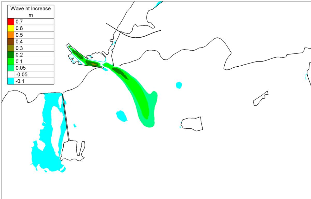
Figure 4.3.18 Difference Plot showing the effect of Tidal velocities on Wave height for SE Storm Wind Waves - Existing
