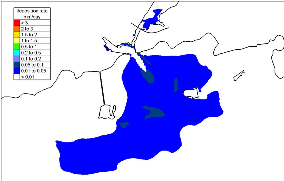
**Figure 4.1.12** Computed depositional rates of a River Corrib fine silt under Winter flood flows (1%-ile 272cume) - Existing Case.
