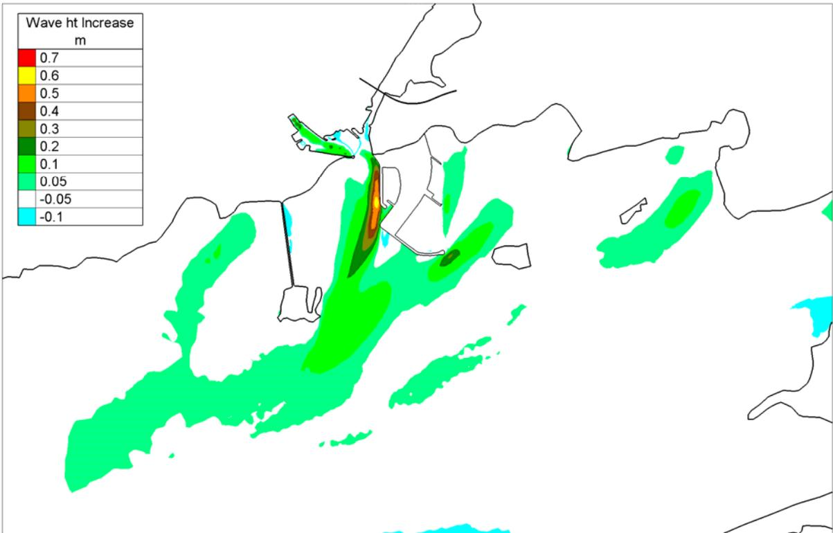
Figure 4.3.9 Difference Plot showing the effect of Tidal velocities on Wave height for South Storm wind conditions - Proposed
