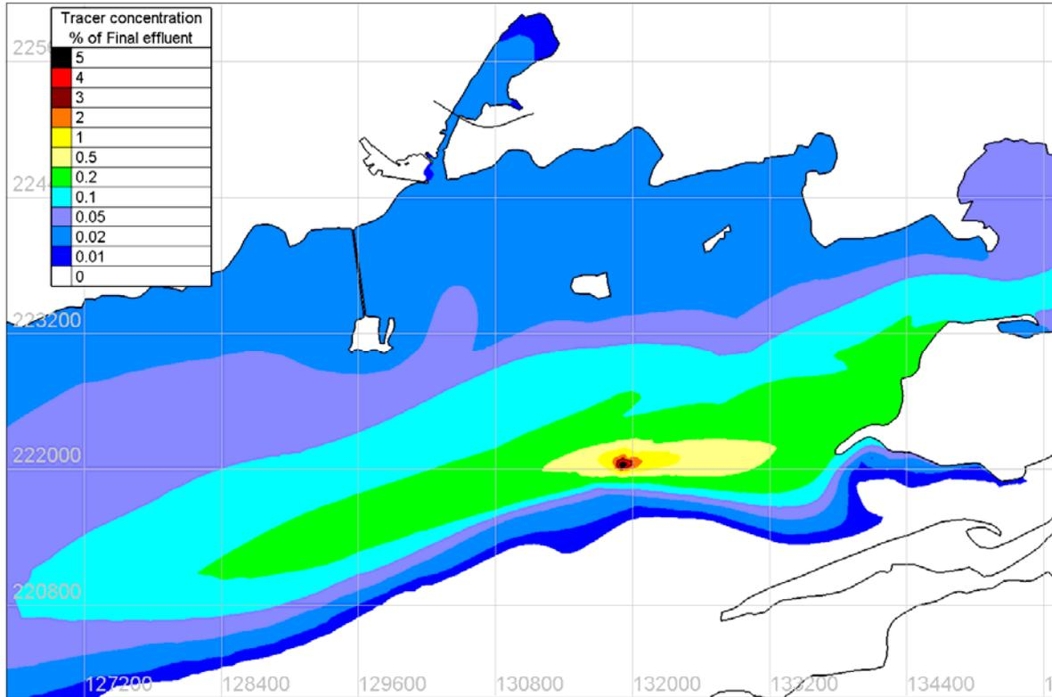
Figure 4.8.49 Maximum surface concentration of Tracer under SW 15m/s wind conditions– Existing
