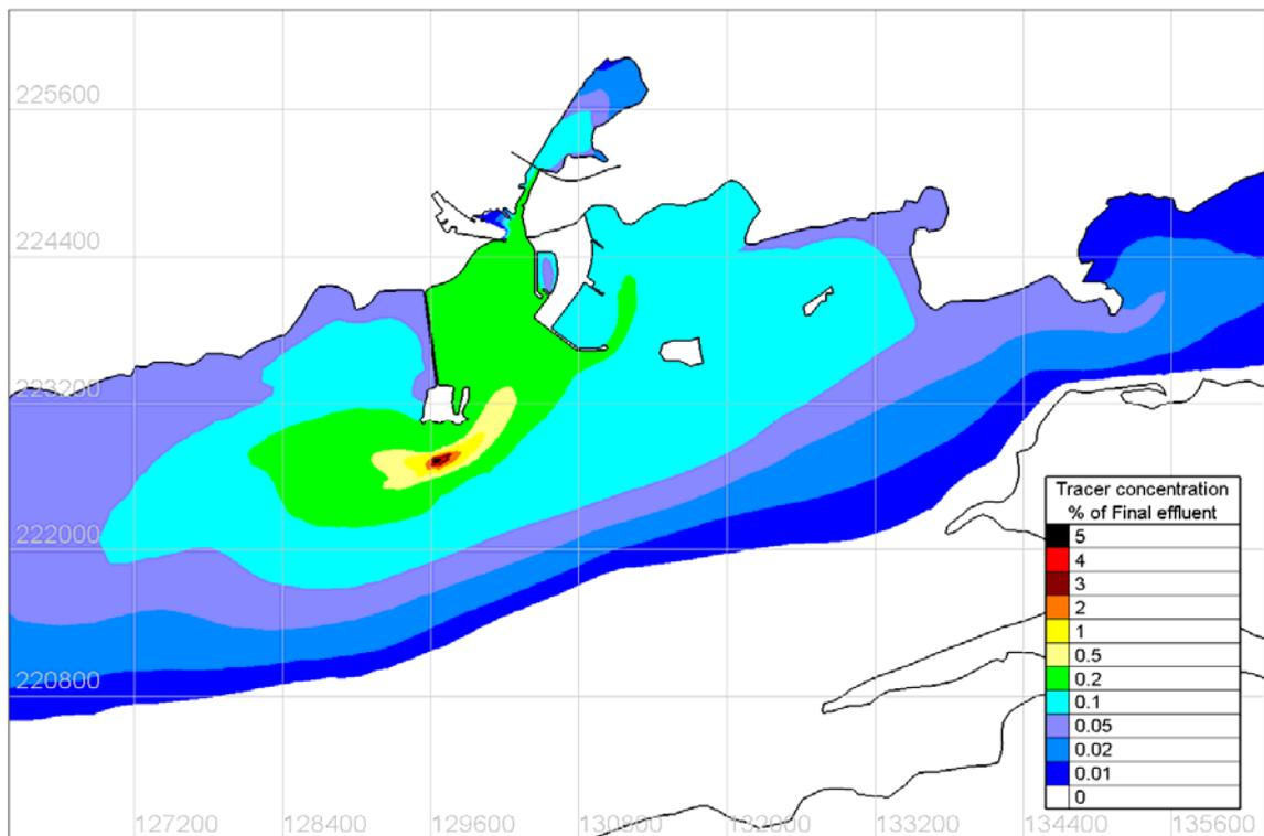
Figure 4.8.2 Maximum surface concentration of Tracer under calm wind conditions – Proposed Case
