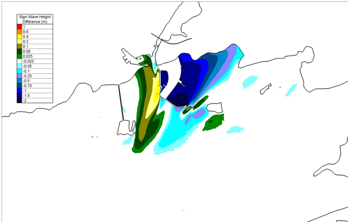
Figure 4.4.31 Difference Plot between Existing and Proposed Significant Wave heights for Local SW Storm Winds
