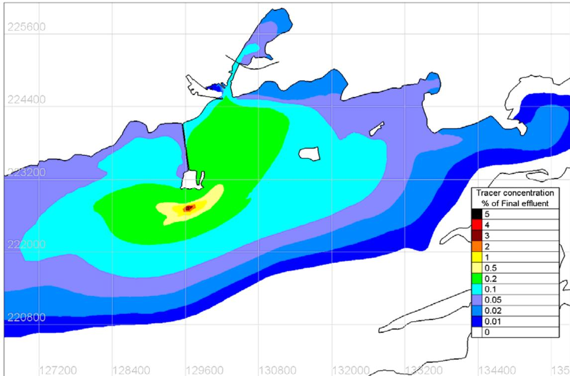
Figure 4.8.1 Maximum surface concentration of Tracer under calm wind conditions – Existing Case
