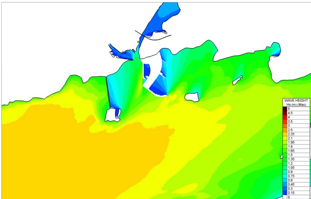
Figure 4.4.16 Computed Significant Wave heights for Local SSW Storm Winds - Proposed
