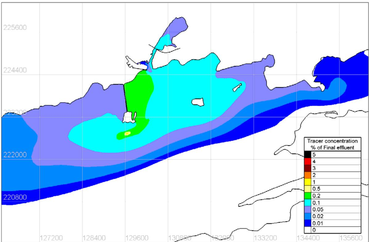
Figure 4.8.9 Tidal mean tracer concentration under SW 5m/s wind conditions – Existing Case
