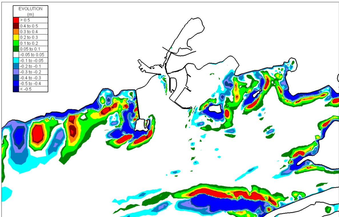
Figure 4.1.21 Southwest Storm Waves Simulation modelling a fine sand - Existing Case
