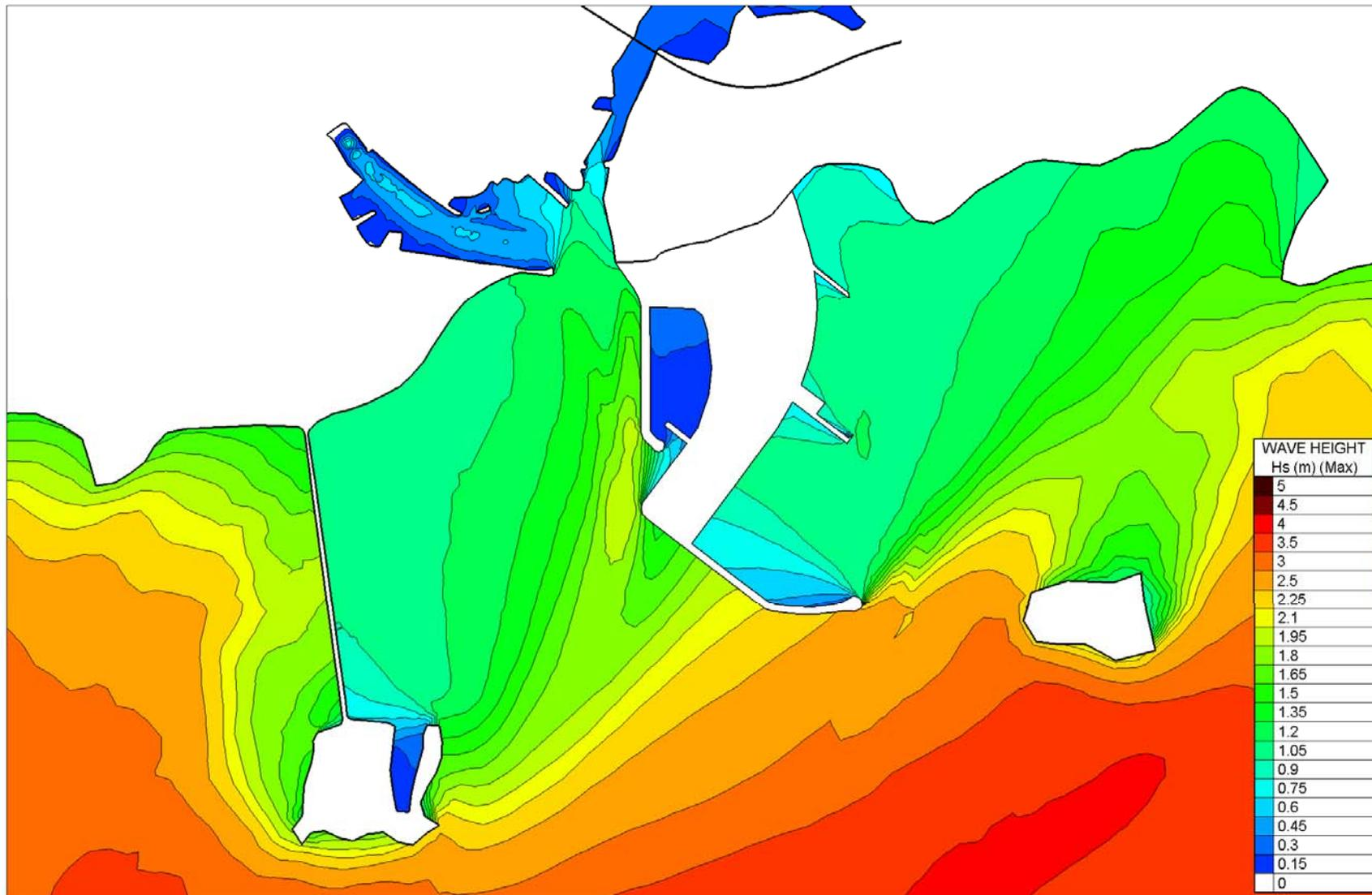
Figure 4.4.40 Computed Maximum Significant Wave Heights – Proposed Case (all on shore directions W to ESE) – Harbour Area (Close up of Fig 4.4.38).
