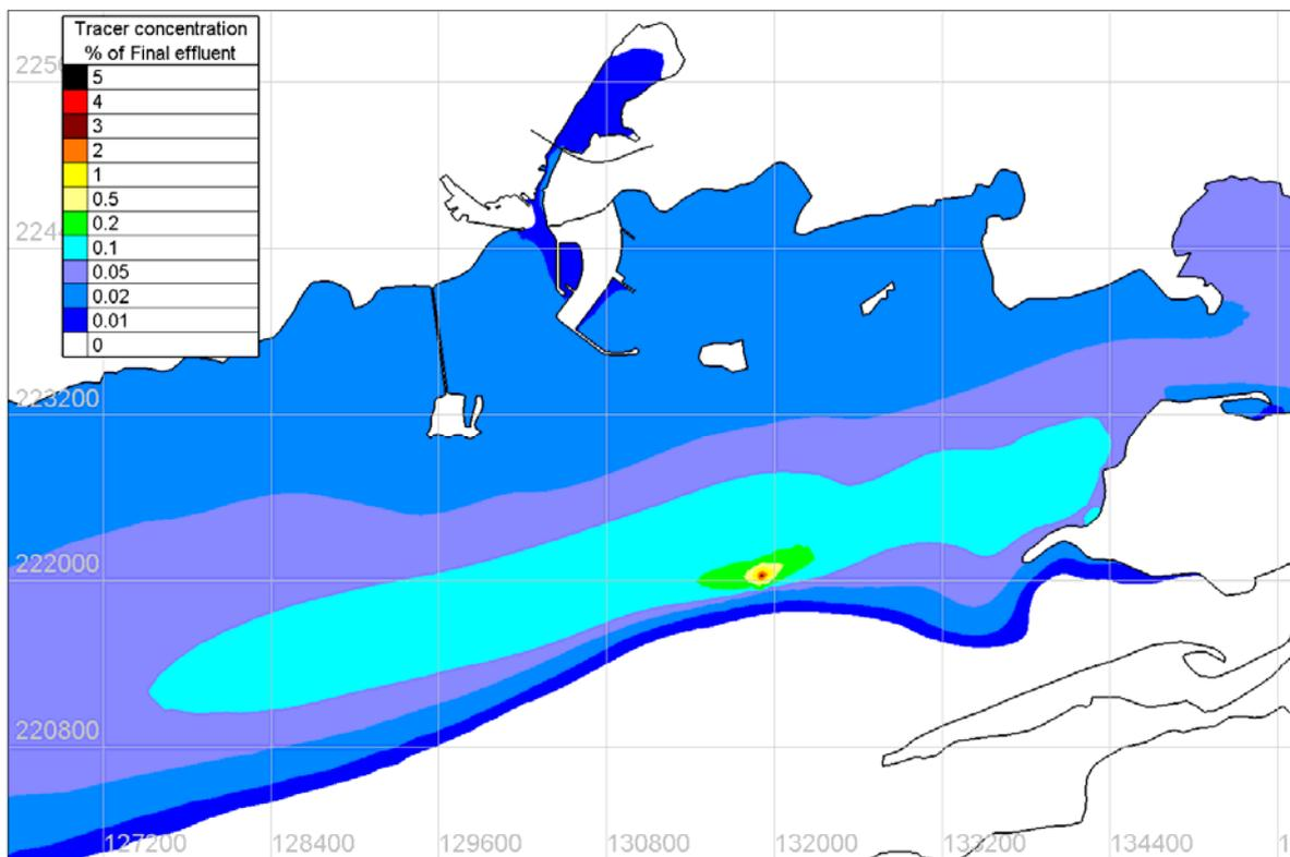
Figure 4.8.52 Tidal mean tracer concentration under SW 15m/s wind conditions – Proposed Case
