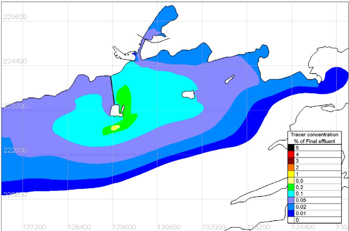
Figure 4.8.3 Tidal mean tracer concentration under calm wind conditions – Existing Case
