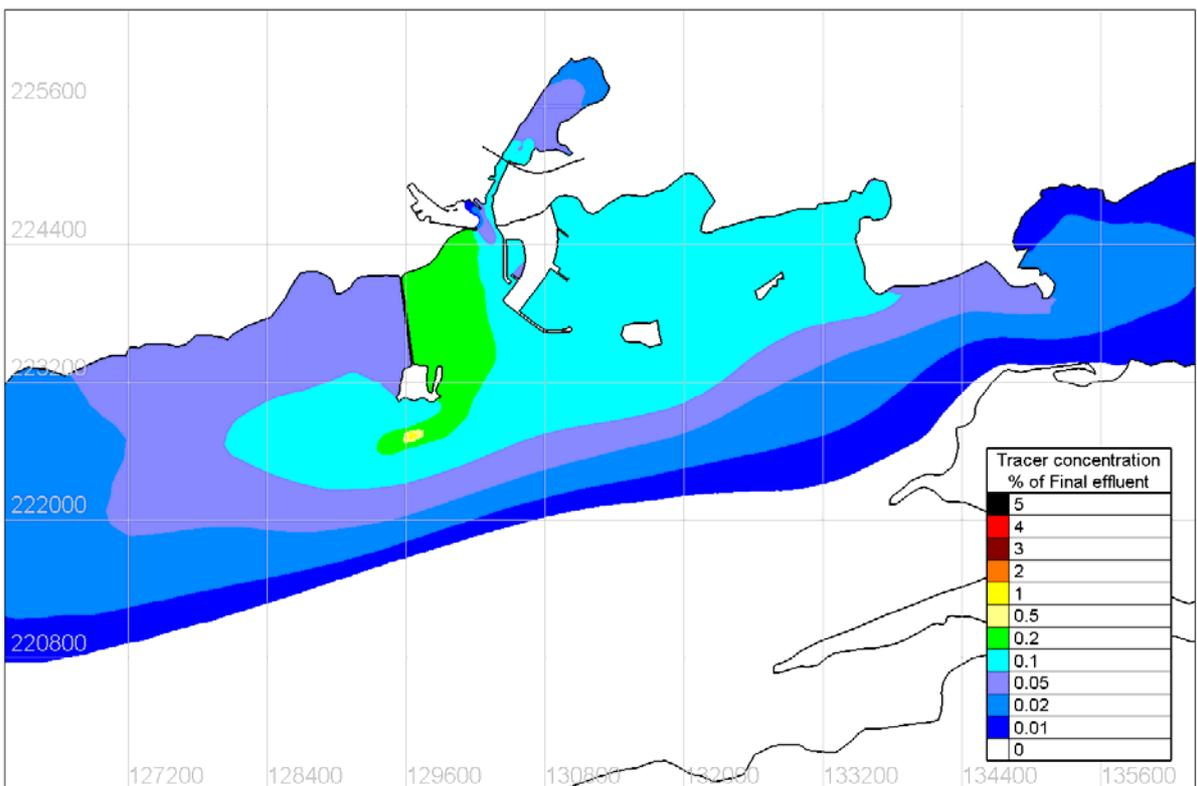
Figure 4.8.10 Tidal mean tracer concentration under SW 5m/s wind conditions – Proposed Case
