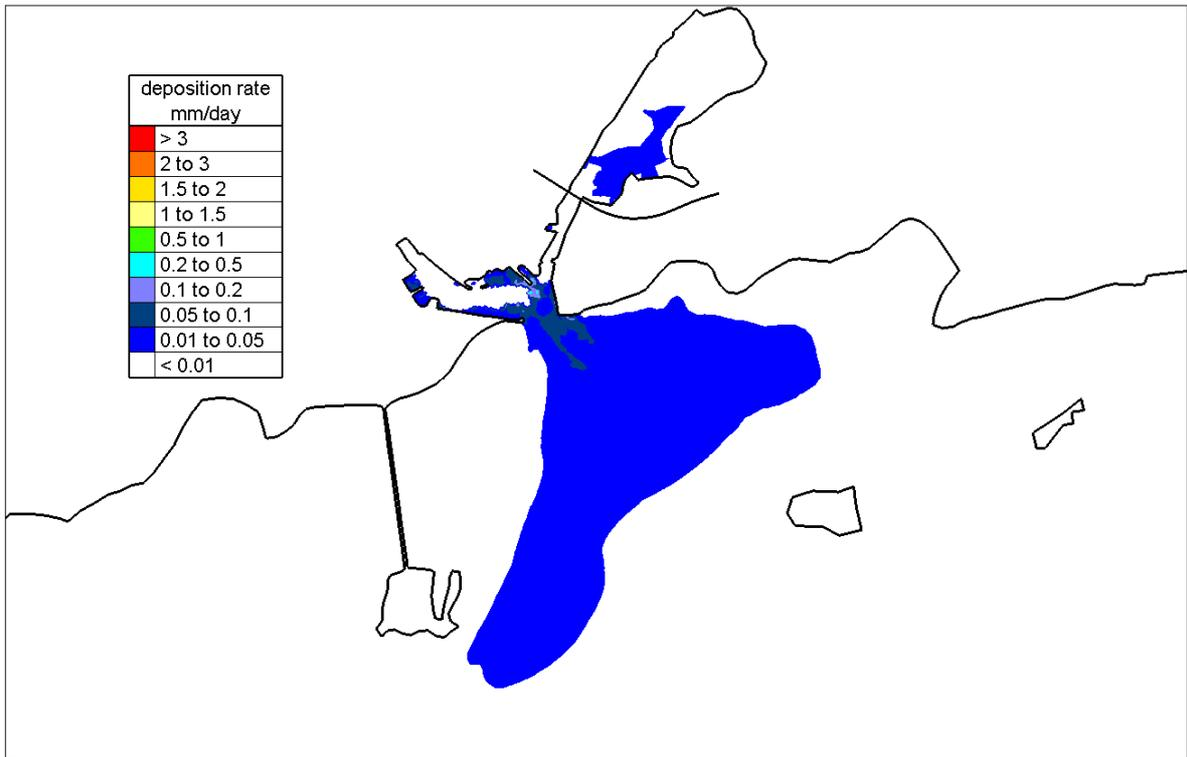
Figure 4.1.4 Computed Depositional Rates of a River Corrib fine silt under median flows for Existing Case
