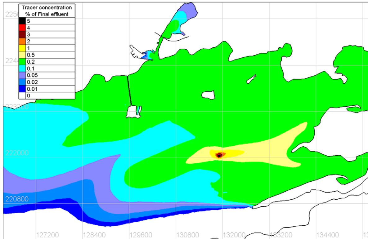
**Figure 4.8.61 Maximum surface concentration of Tracer under SE 15m/s wind conditions— Existing**
