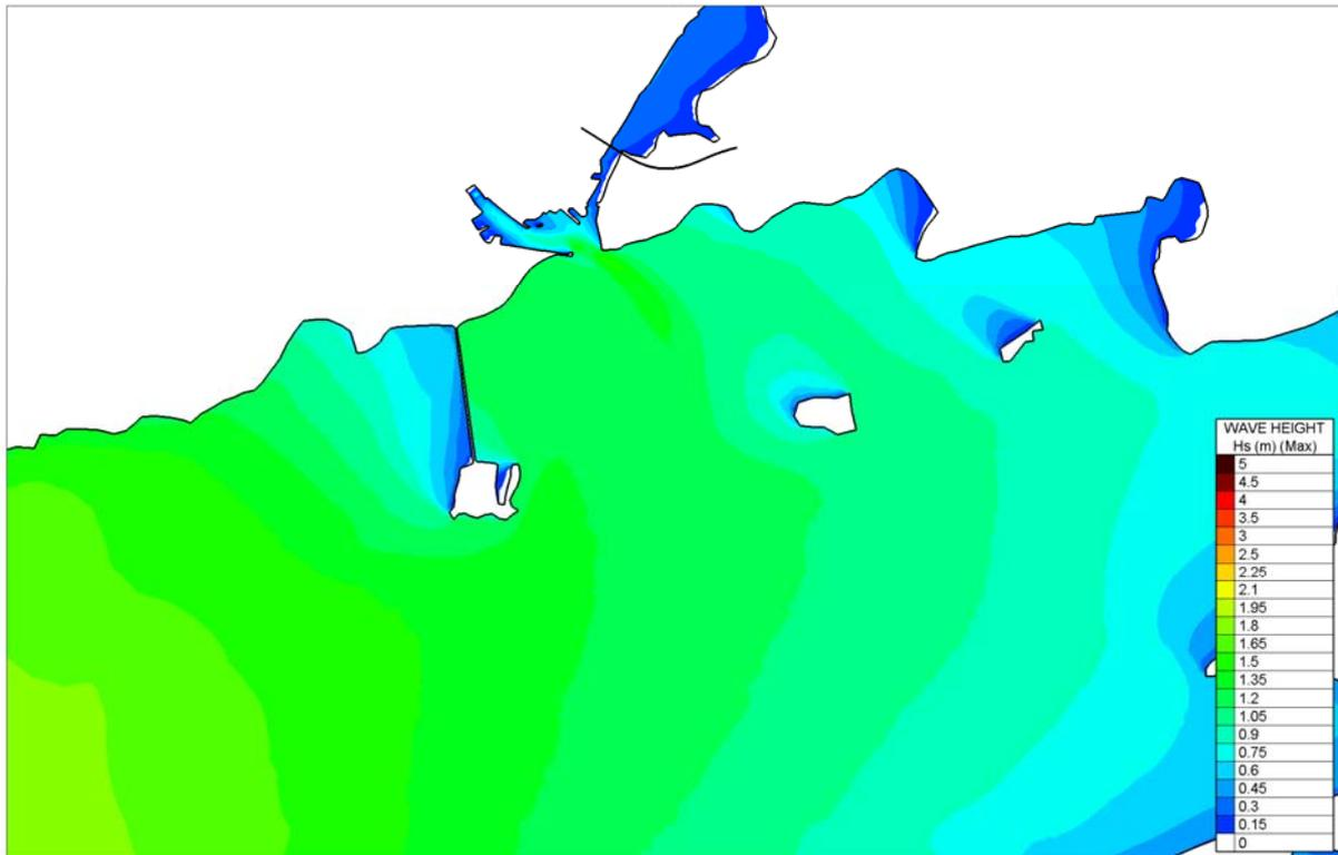
Figure 4.4.23 Computed Significant Wave heights for Local ESE Storm Winds - Existing
