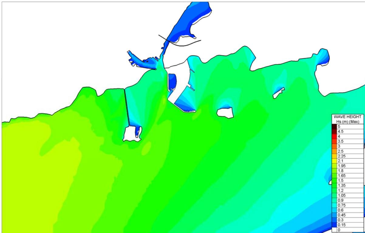
Figure 4.4.20 Computed Significant Wave heights for Local SSE Storm Winds - Proposed
