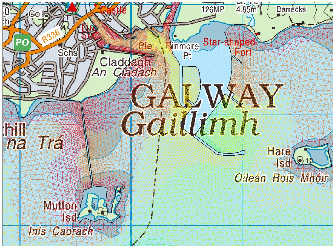
Figure 4.3.3 Swan Wave Model Domain and refined mesh in vicinity of Harbour Development (similar to hydrodynamic model mesh)
