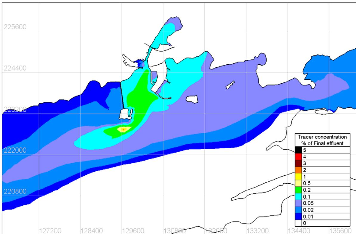
Figure 4.8.26 Maximum surface concentration of Tracer under SW 15m/s wind conditions– Proposed
