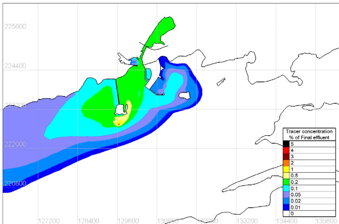
Figure 4.8.38 Maximum surface concentration of Tracer under S 15m/s wind conditions– Proposed
