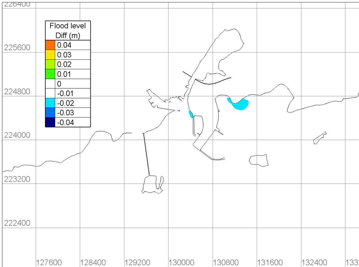
Figure 4.6.13 Difference Plot between predicted existing and Proposed peak flood levels
