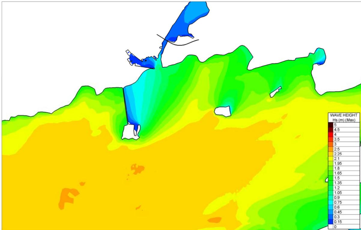
Figure 4.4.13 Computed Significant Wave heights for Local SW Storm Winds - Existing
