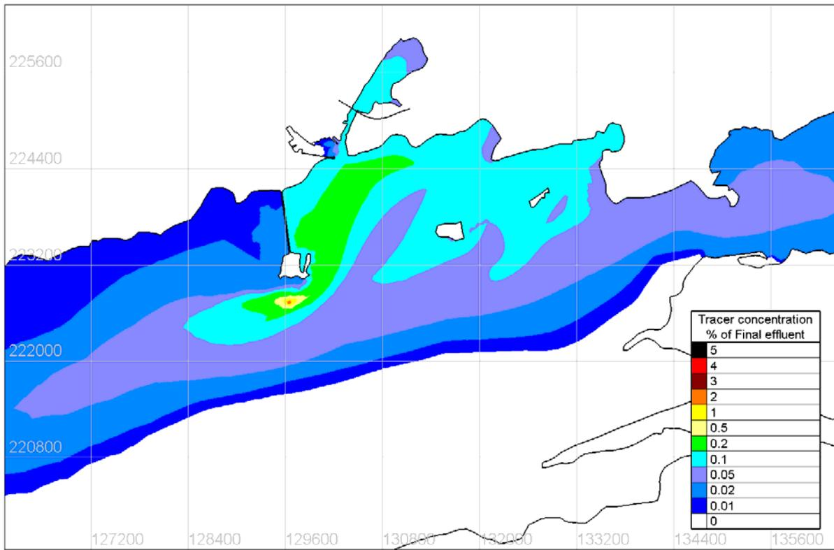
Figure 4.8.25 Maximum surface concentration of Tracer under SW 15m/s wind conditions– Existing
