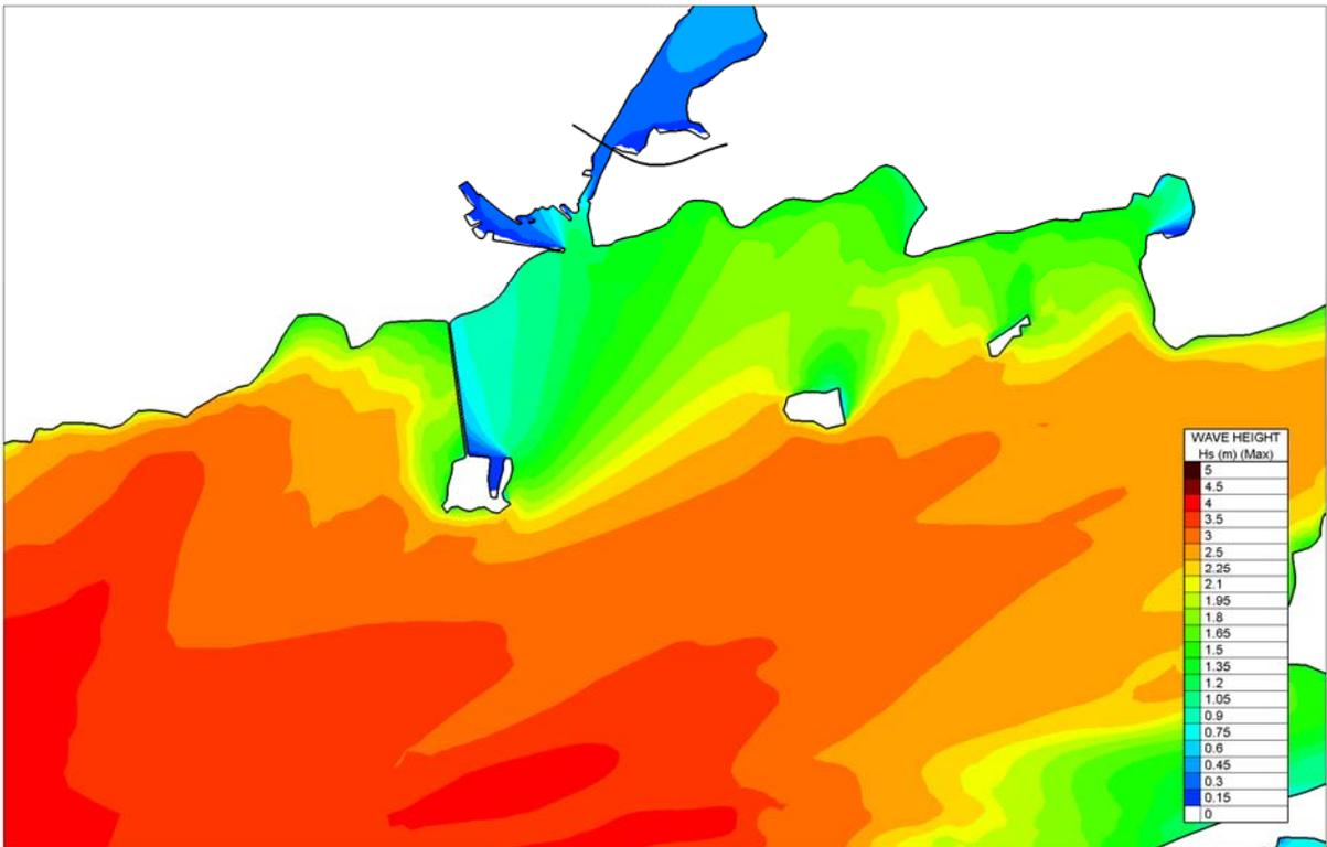
Figure 4.3.10 Predicted Wave Climate for SSW storm Wind without including tidal velocities – Existing
