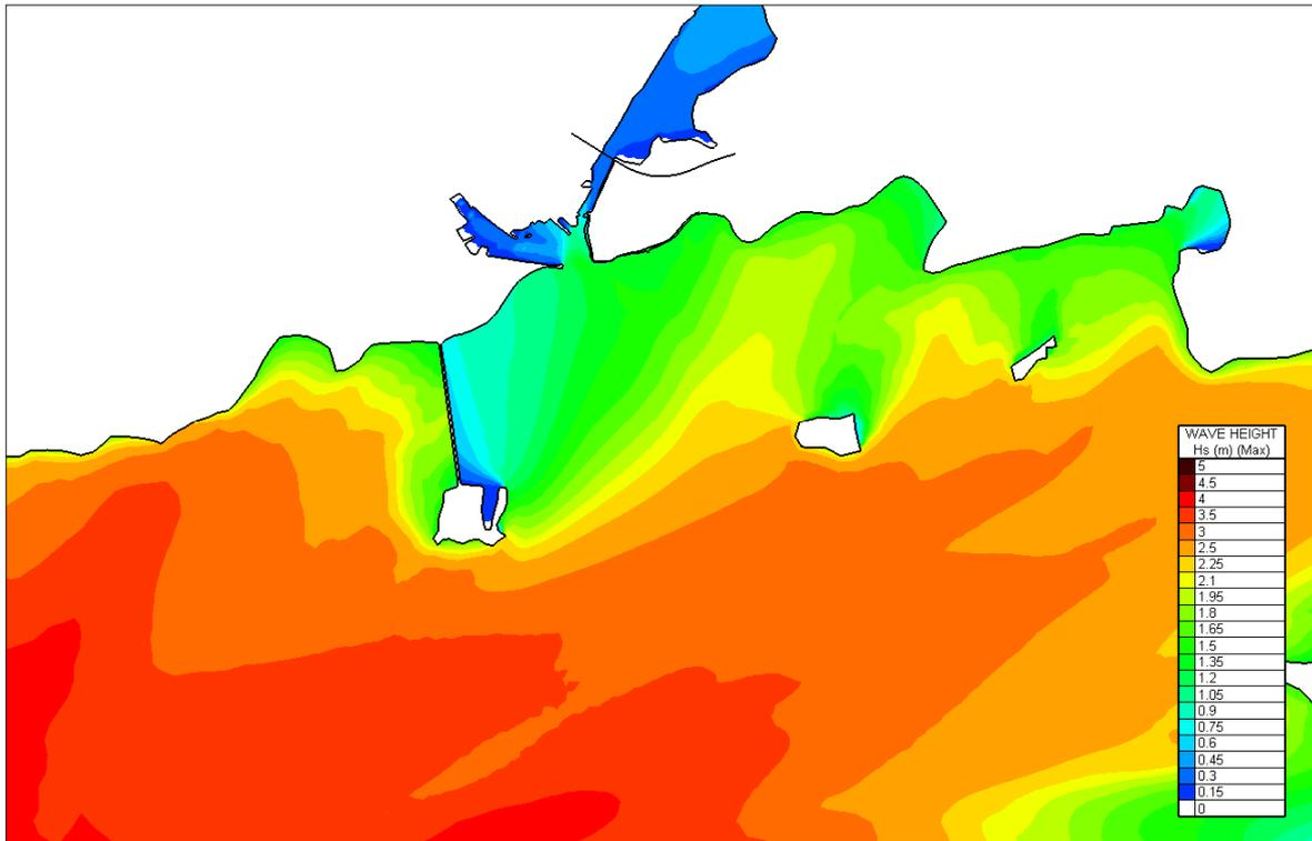
Figure 4.4.7 Computed Significant Wave heights for Atlantic Storm and SSW Storm Winds - Existing
