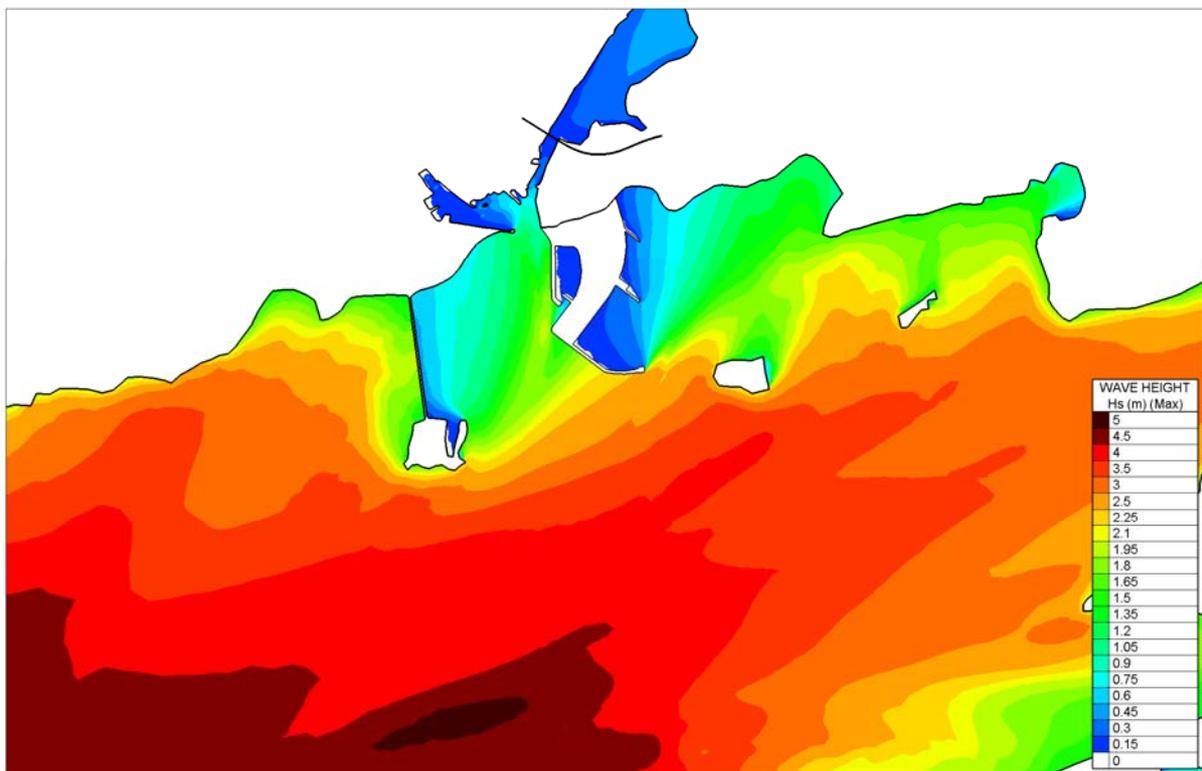
Figure 4.4.4 Computed Significant Wave heights for Atlantic Storm and WSW
