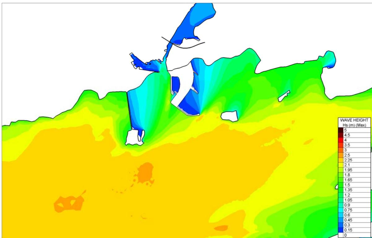
Figure 4.4.14 Computed Significant Wave heights for Local SW Storm Winds - Proposed
