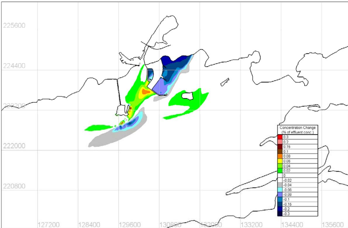
Figure 4.8.35 Predicted change in maximum surface tracer concentration – SSW 15m/s Wind Conditions
