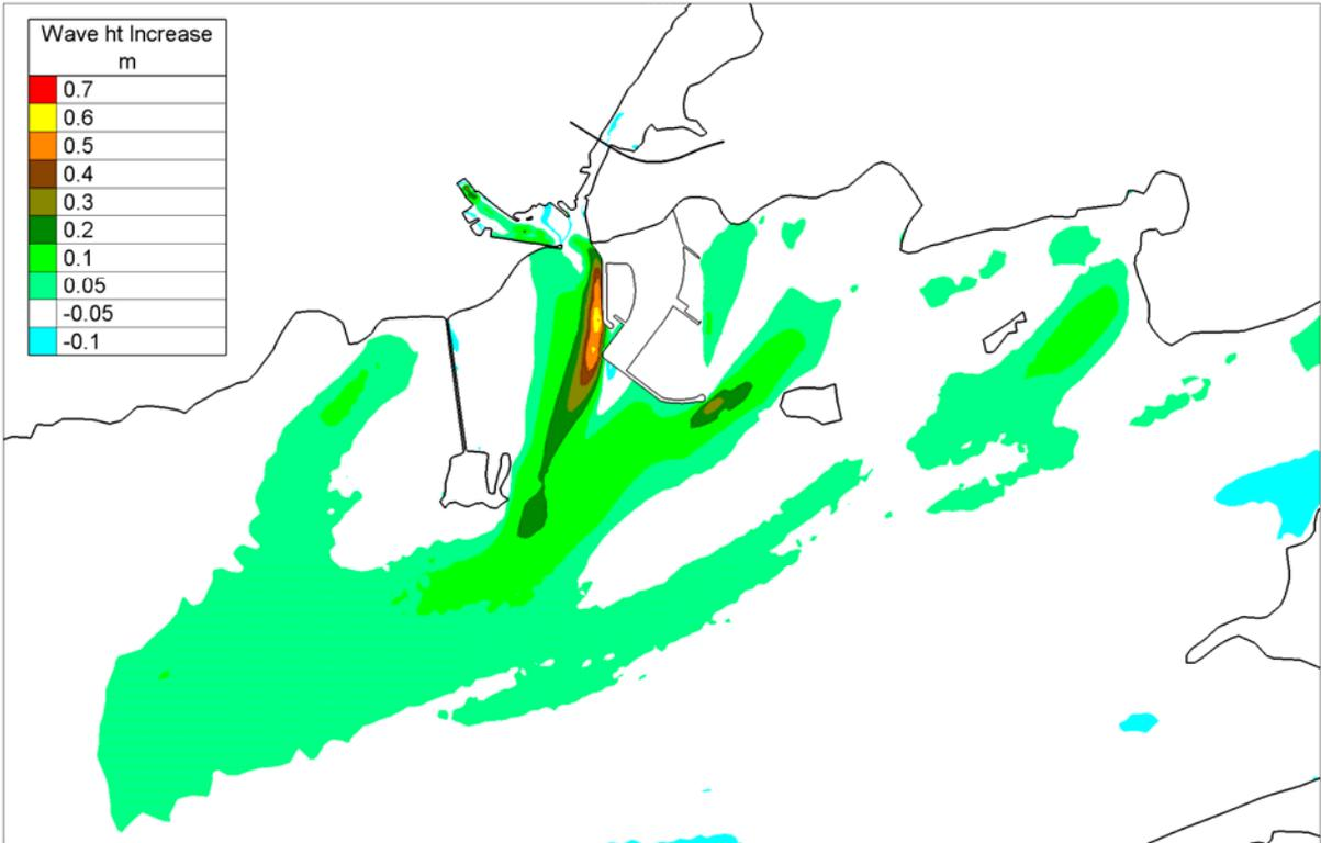
Figure 4.3.6 Difference Plot showing the effect of Tidal velocities on Wave height for SSW Storm wind conditions - Proposed
