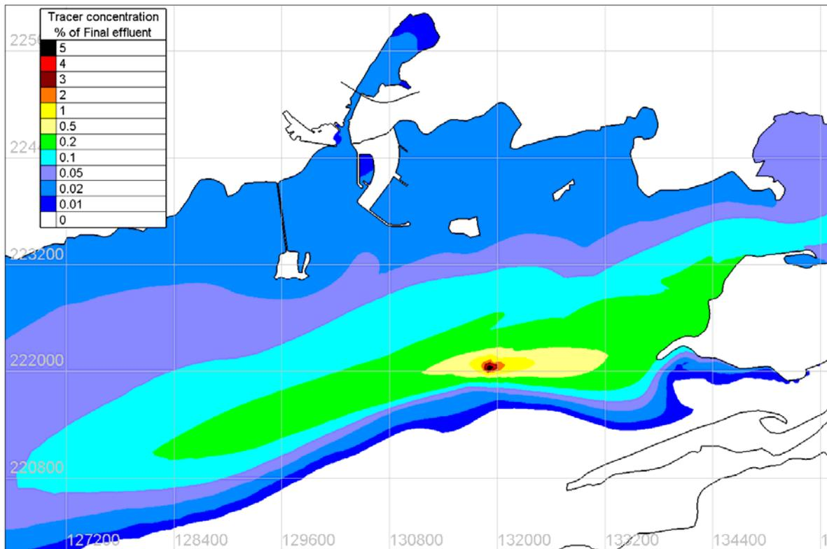
Figure 4.8.50 Maximum surface concentration of Tracer under SW 15m/s wind conditions– Proposed
