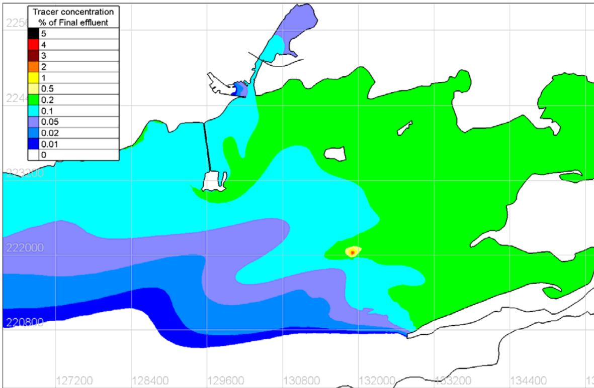
Figure 4.8.63 Tidal mean tracer concentration under SE 15m/s wind conditions – Existing Case
