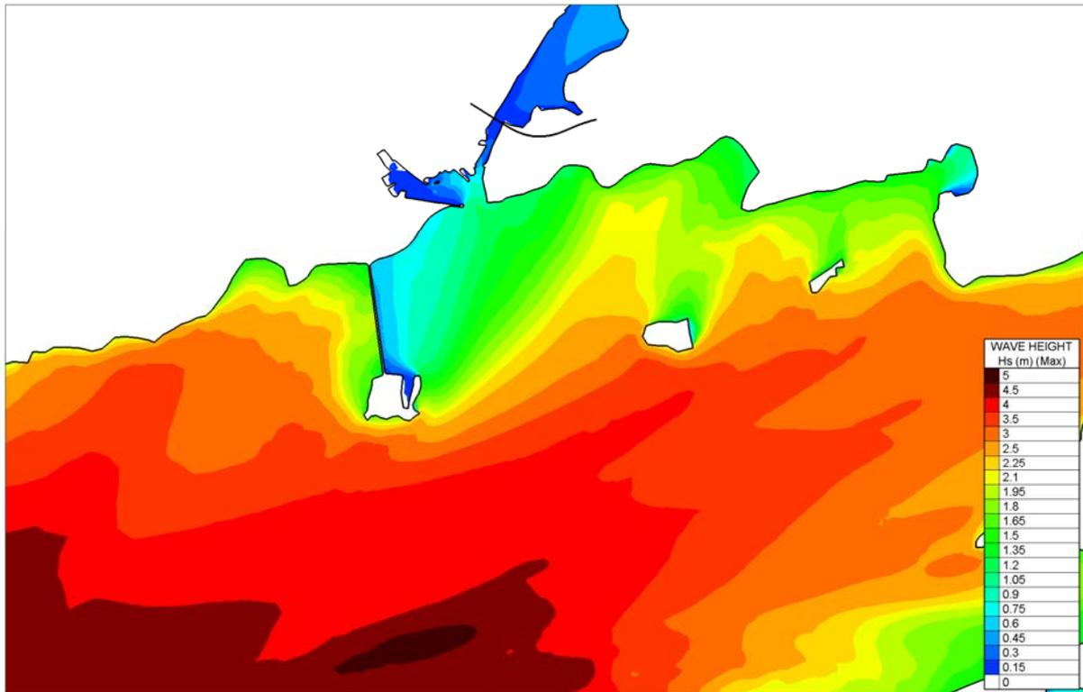
Figure 4.4.3 Computed Significant Wave heights for Atlantic Storm and WSW
