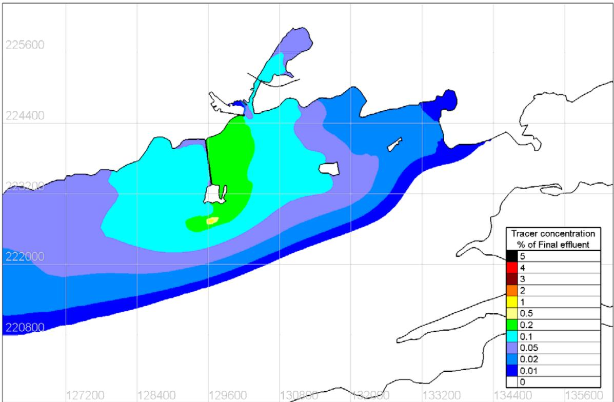
Figure 4.8.21 Tidal mean tracer concentration under South 5m/s wind conditions – Existing Case
