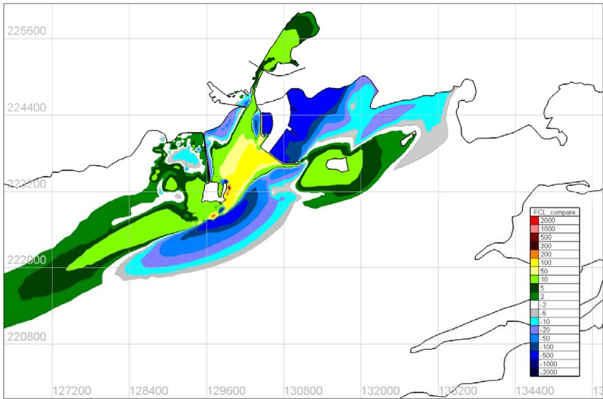
Figure 4.8.48 Predicted change in maximum surface tracer concentration – SSW Wind Conditions
