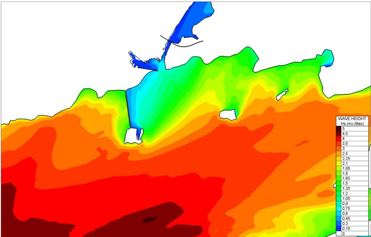
Figure 4.4.1 Computed Significant Wave heights for Atlantic Storm and West Storm Winds - Existing
