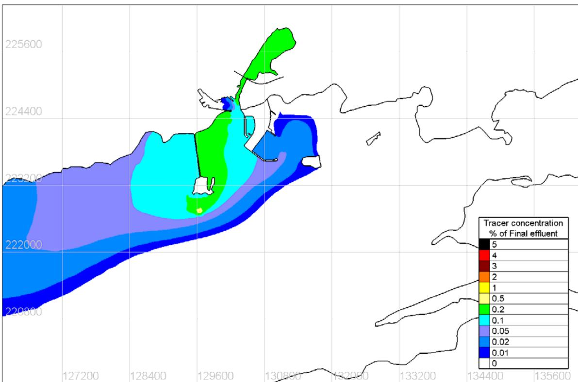
Figure 4.8.40 Tidal mean tracer concentration under S 15m/s wind conditions – Proposed Case
