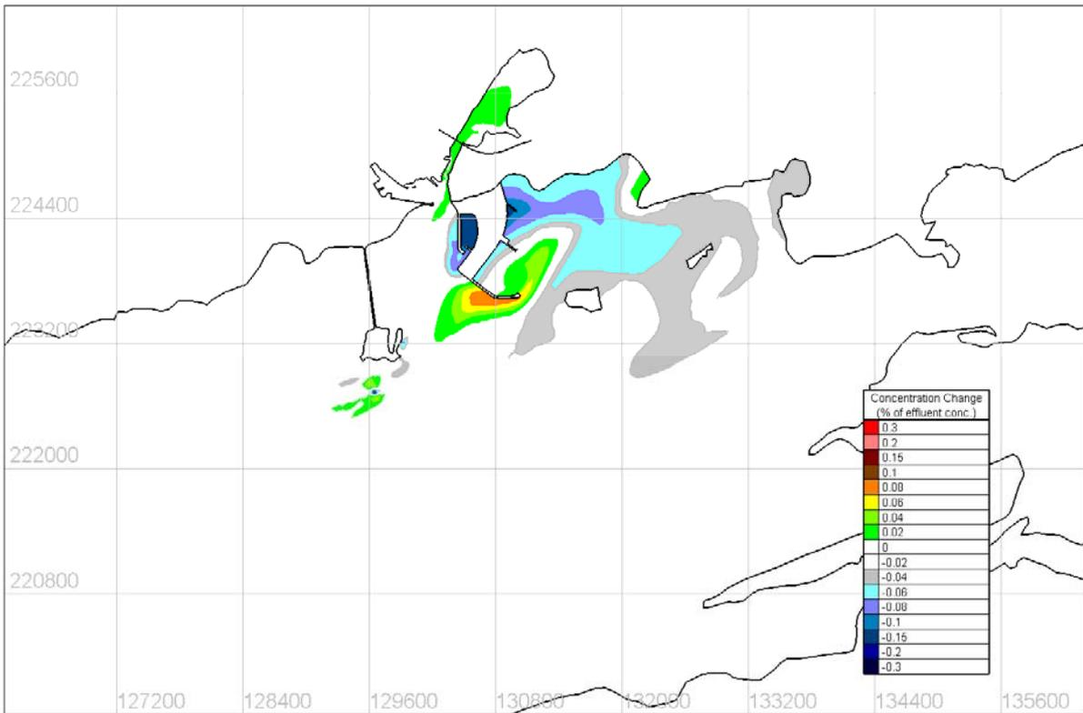
Figure 4.8.29 Predicted change in maximum surface tracer concentration – SW 15m/s Wind Conditions
