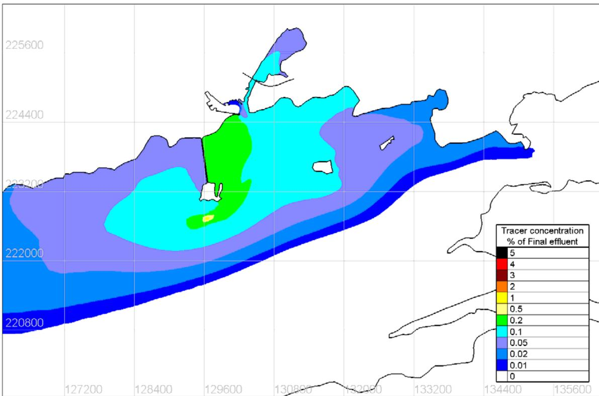
Figure 4.8.15 Tidal mean tracer concentration under SSW 5m/s wind conditions – Existing Case
