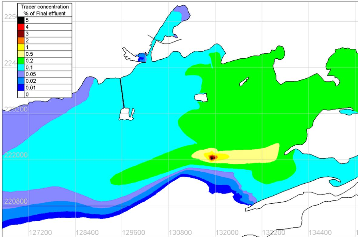
Figure 4.8.55 Maximum surface concentration of Tracer under S 15m/s wind conditions– Existing
