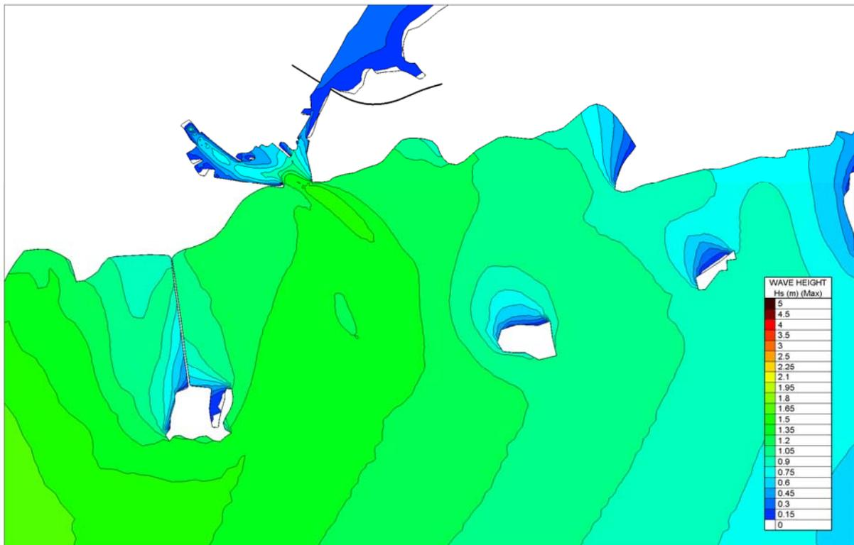
Figure 4.3.17 Predicted Wave Climate for local SE storm wind waves with tidal velocities included - Existing
