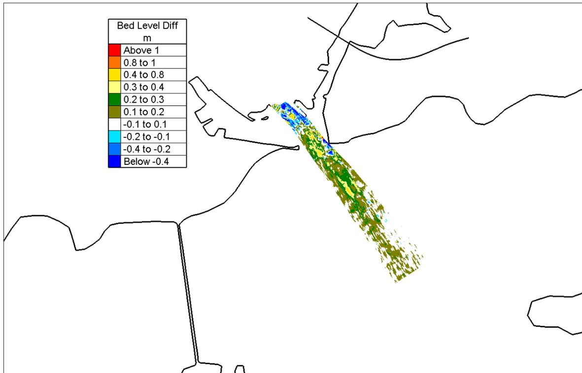
Figure 4.1.1 Difference plot of existing navigation channel HSL Survey - January 2014 and January 2012 showing principal deposition over 2 year period occurring primarily at and near the Corrib entrance.
