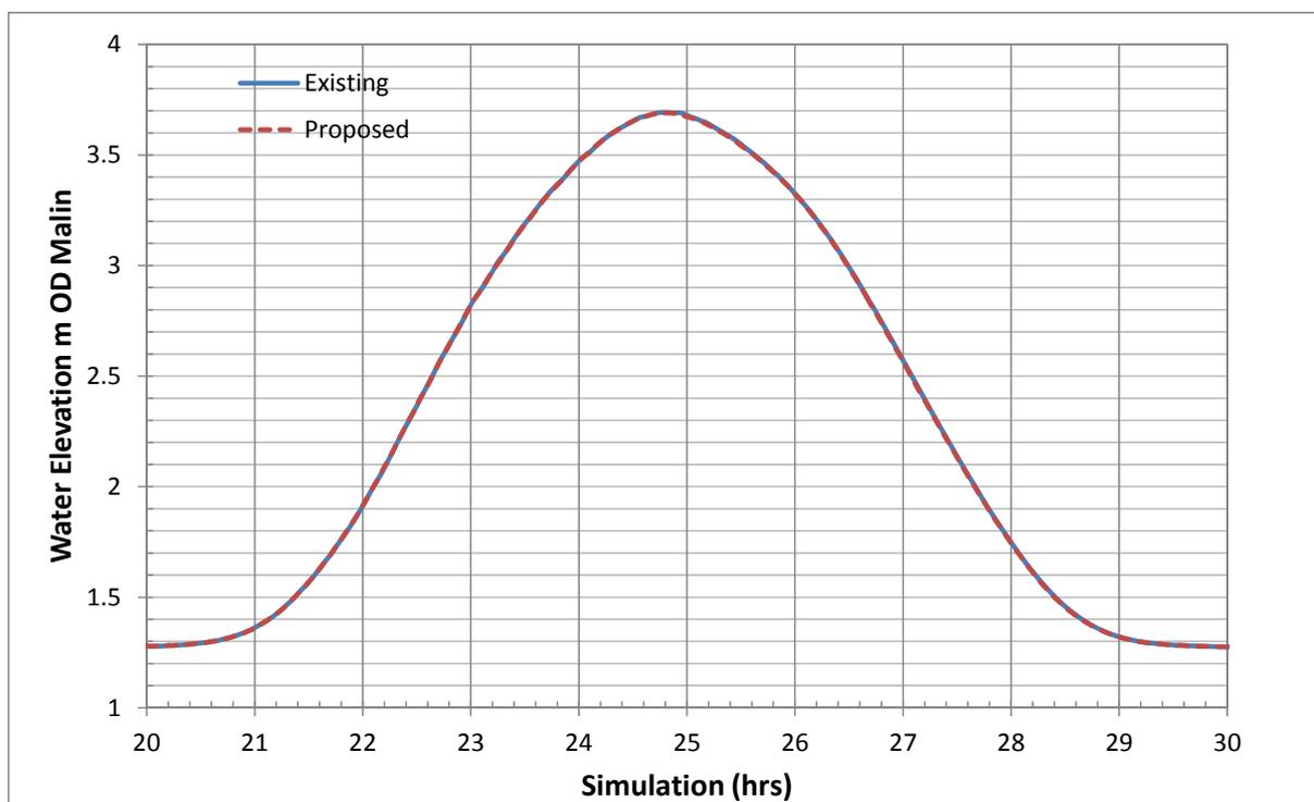
Figure 4.6.12 Comparison of Tide level at Site 1 Cladagh Basin for proposed and existing case under 3.5m tidal surge, 100year Corrib flood Flow and 20m/s southerly wind for proposed and existing scenarios (Existing and Proposed overlapping)
