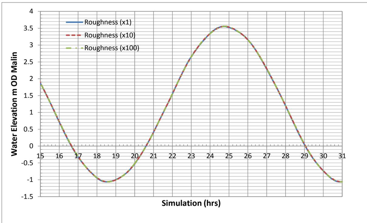
Figure 4.6.3 Sensitivity of elevation to Roughness factor at Site 2
