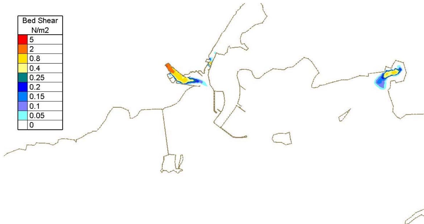
Figure Error! No text of specified style in document..30 - Computed bed shear at mid-flood with new harbour extension development – Neap Tide and Median River Corrib Flow (82 m 3 /s)
